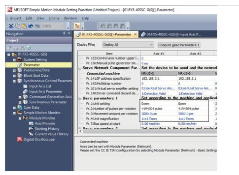
• The basic position information per rotation for the servo amplifier is 26 bit (67108864 pulse).
