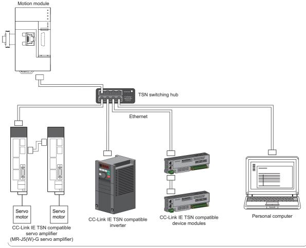
FX5-40SSC-G: Up to 4 Motion control stations + 16 standard stations FX5-80SSC-G: Up to 8 Motion control stations + 16 standard stations
