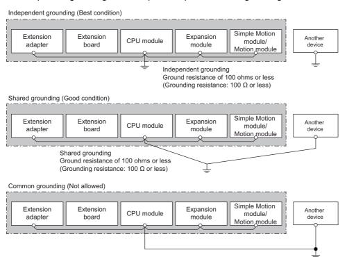
• Limit the distance between the grounding point and the programmable controller as much as possible and keep the grounding wire short.
