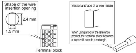
The following table shows wire ferrules and its associated tools compatible with the terminal block. The shape of the wire ferrule differs depending on the crimp tool to be used, use the reference product. If the product other than referenced products is used, the wire ferrule cannot be removed. Sufficiently confirm that the wire ferrule can be removed before use.
