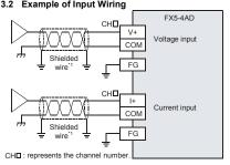
\*1 For analog input wiring, use shielded twisted-pair cables (double-core type). Separate them from other power lines or lines which are sensitive to
