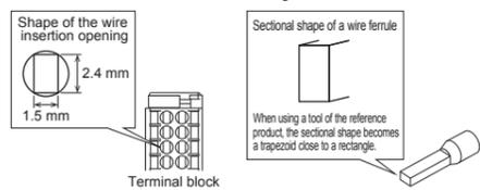
The following table shows wire ferrules and its associated tools compatible with the terminal block. The shape of the wire ferrule differs depending on the crimp tool to be used, use the reference product. If the product other than referenced products is used, the wire ferrule cannot be removed. Sufficiently confirm that the wire ferrule can be removed before use.
