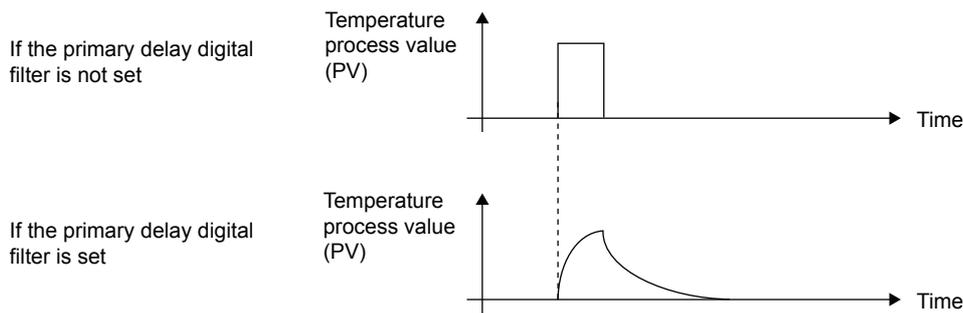
The time for the temperature process value (PV) to change by 63.3% can be set by the primary delay digital filter setting (filter setting time).
