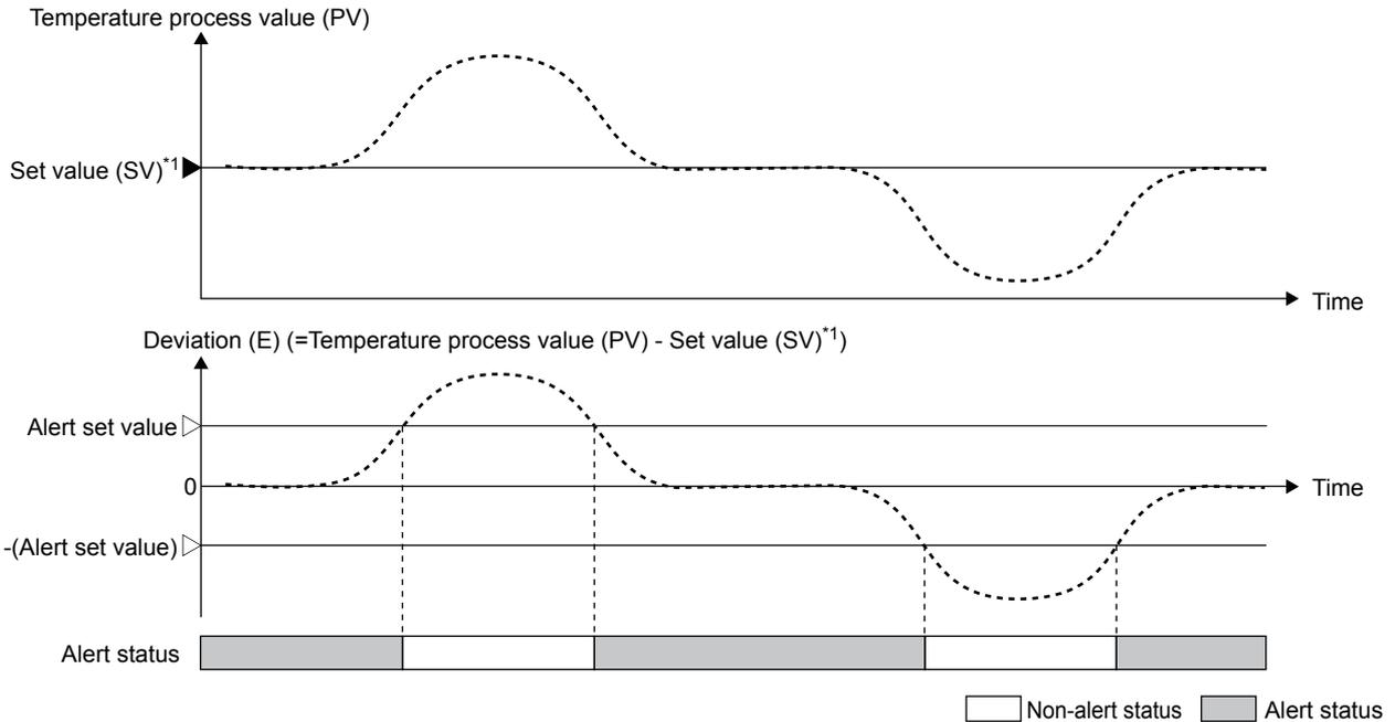
\*1 Depending on the alert mode setting, this value becomes the set value or the monitored value. The setting range of the alert set value is  $-(\text{Full scale of the input range})$  to the full scale of the input range. (Page 54 Setting the set value (SV) and the setting change rate limiter)
