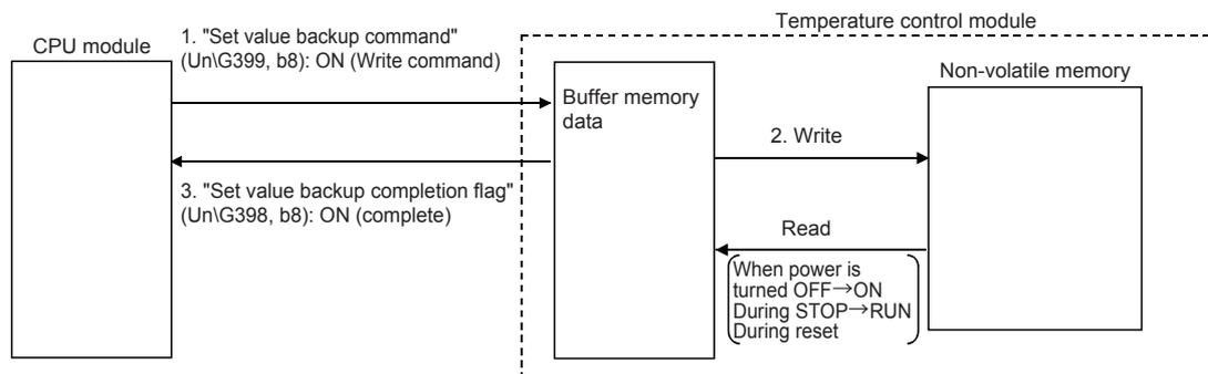
If writing the data to the non-volatile memory is not completed successfully, 'Setting value backup failure flag' (Un\G398, b10) turns ON.
