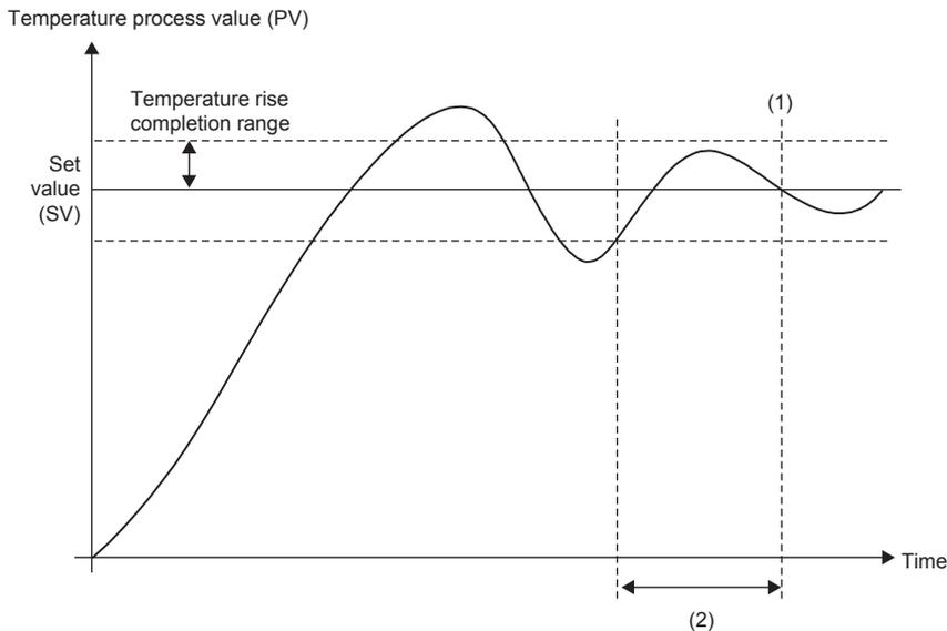
(1) At this time, 'CH1 Temperature rise judgment flag' (Un\G404) is set to Within temperature rise completion range (ON).
