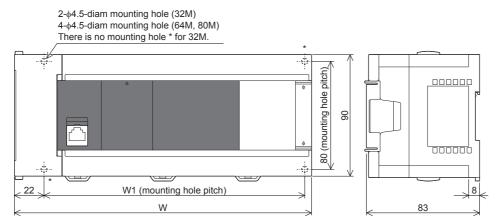
External color: Munsell 0.6B7.6/0.2 Unit: mm The terminal block uses M3 terminal screws
