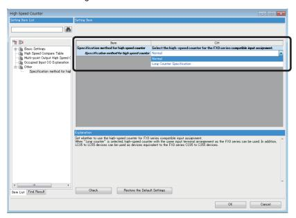
2. Set the function of the high-speed counters used with the FX3U.
