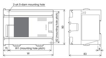
External color: Munsell 0.6B7.6/0.2 Unit: mm The terminal block uses M3 terminal screws
