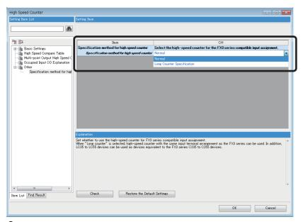
**2.** Set the function of the high-speed counters used with the FX3G.
