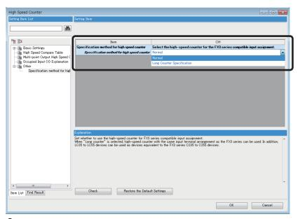
**2.** Set the function of the high-speed counters used with the FX3UC.
