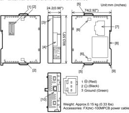
[1]FX3UC Main unit, FX2NC/FX3UC Extension block connector [2]FX3UC Main unit, FX2NC/FX3UC Extension block connecting hook
