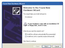
Add a check mark to [ Install from a list or specific location (Advanced) ] and click [ Next > ]. The window to select the installation path for the files will
