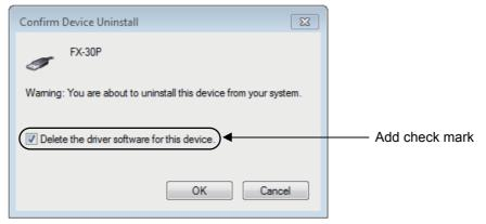
Add a check mark to [ Delete the driver software for this device. ], and click [ OK ]. The USB driver is uninstalled.
