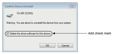
Add a check mark to [ Delete the driver software for this device. ], and click [ OK ]. The USB Serial Port software is uninstalled.
