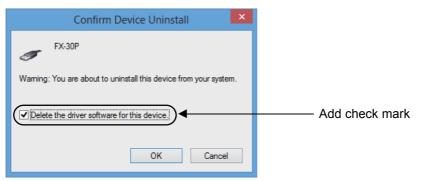
Add a check mark to [ Delete the driver software for this device. ], and click [ OK ]. The USB driver is uninstalled.
