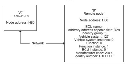
1) Tx/Rx User messages and one RUN>STOP message configured, but no Remote Address to ECU Name assignment
