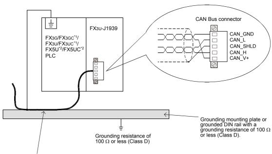
Strip a part of the coating of the shielded twisted pair cable as shown in subsection 4.2.3. Ground the PLCs grounding terminal there.
