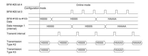
The user interval set for the message is restarted every time the message is transmitted. In case the transmission is triggered by a request message from the network or manual trigger (BFM #1280 to #1284), the next transmission after externally/manual triggered message will not be sent in the former interval "\*1," but in the new interval related to the external/manual trigger event.
