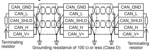
For electromagnetic compatibility (EMC), it is recommended to ground the cable shield at both ends.
