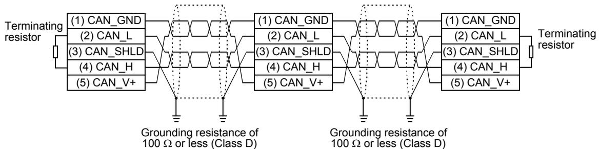
For electromagnetic compatibility (EMC), it is recommended to ground the cable shield at both ends.
