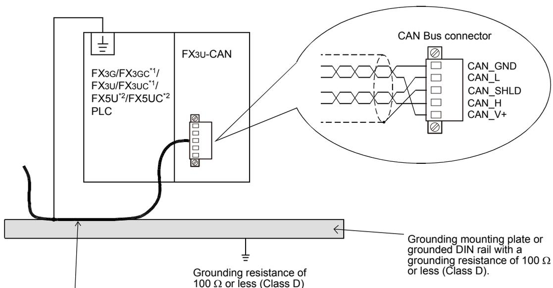
Strip a part of the coating of the shielded twisted pair cable as shown in subsection 4.2.3. Ground the PLC's grounding terminal there.
