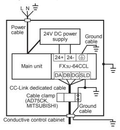
· Wiring simplified diagram
