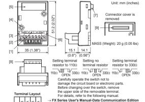
[1]Terminal resistor changing-over switch (110Ω/OPEN/330Ω)
