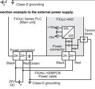
1) Connection example with the power supply through crossover wiring to the FX2NC input extension block
