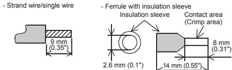
When using a ferrule with insulation sleeve, choose a wire with proper cable sheath referring to the above outside dimensions, or otherwise, the wire cannot be inserted easily. The tightening torque must be 0.22 to 0.25 N·m. Do not tighten terminal screws with a torque outside the above-mentioned range. Failure to do so may cause equipment failures or malfunctions.
