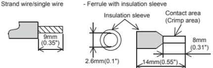
When using a ferrule with insulation sleeve, choose a wire with proper cable sheath referring to the above outside dimensions, or otherwise, the wire cannot be inserted easily. The tightening torque must be 0.22 to 0.25 N·m. Do not tighten terminal screws with a torque above the above-mentioned range. Failure to do so may cause equipment failures or malfunctions.
