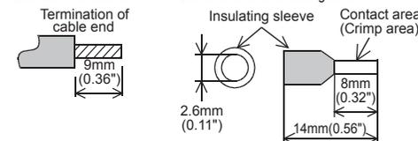
When using a stick terminal with an insulating sleeve, choose a wire with proper cable sheath referring to the above outside dimensions, otherwise the wire cannot be inserted easily.
