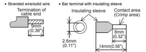
When using a stick terminal with an insulating sleeve, choose a wire with proper cable sheath referring to the above outside dimensions, otherwise the wire cannot be inserted easily. Tighten the screws to a torque of 0.22 to 0.25 N·m. Do not tighten terminal screws with a torque outside the above-mentioned range. Failure to do so may cause equipment failures or malfunctions.
