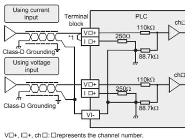
\*1 Make sure to short-circuit the 'V+' and 'I+' terminals when current is input. (□: input channel number)
