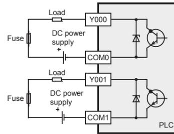
2. External Wiring of Source Output Type
