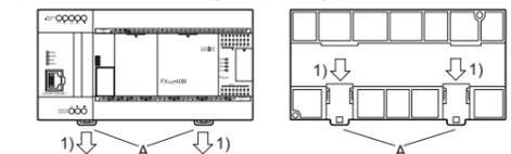
2) Fit the upper edge of the DIN rail mounting groove (right fig.B) onto the DIN rail.
