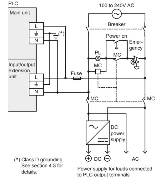
4.2.3 Example of external wiring (DC power type)
