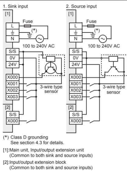
4.4.3 Examples of input wiring [DC power type]
