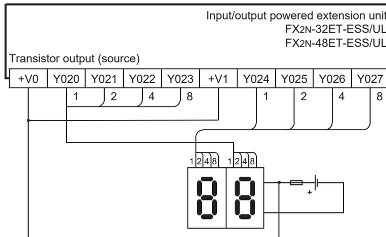
7-segment display to be used for source wiring (in the case of transistor output)
