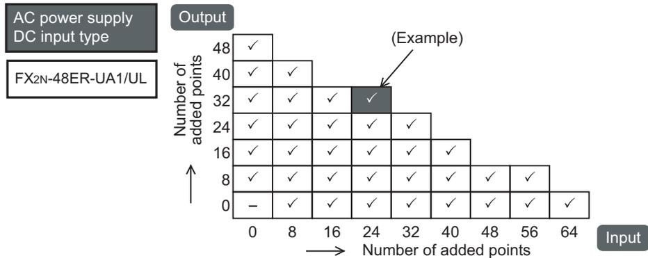
(Example) When adding 24 inputs to FX2N-48ER-UA1/UL, a maximum of 32 outputs are expandable
