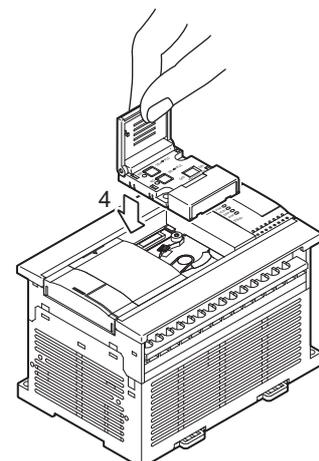
**5** The memory cassette (E in the right figure) can be fixed with provided M3 tapping screws (D in the right figure) to the main unit. This work is not required when fixation is not necessary.
