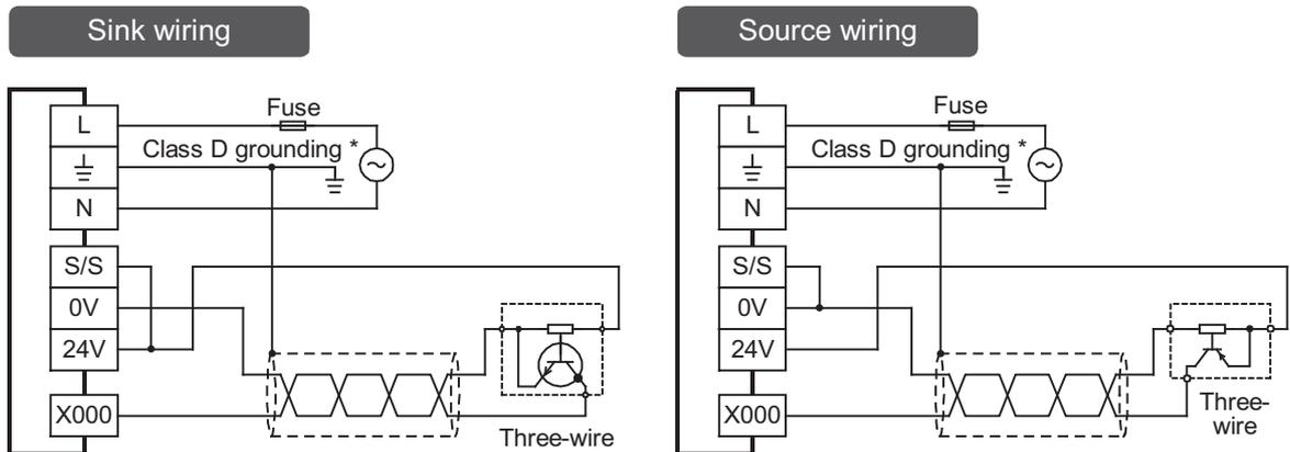
\* The grounding resistance should be 100Ω or less.
