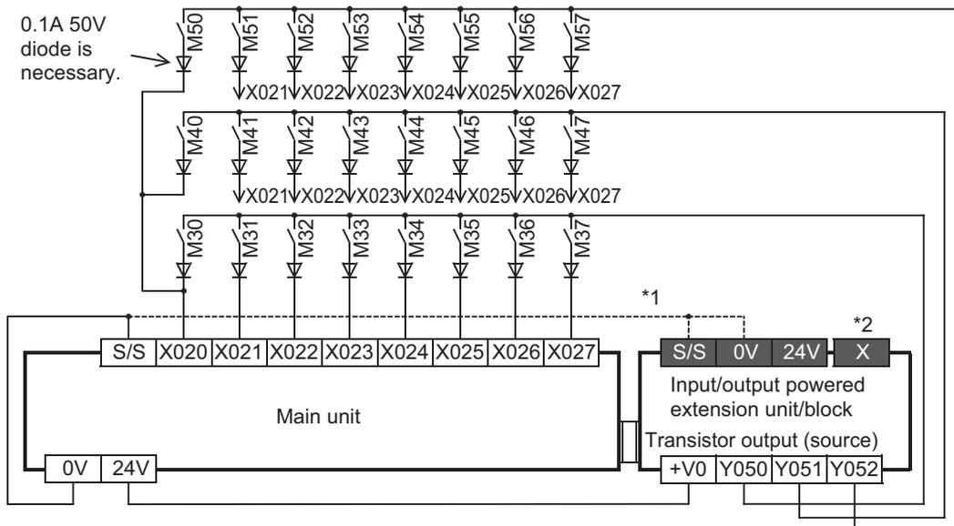
\*1 To use the input terminal (X) of the input/output powered extension unit, wire the terminal as shown by the dotted line.
