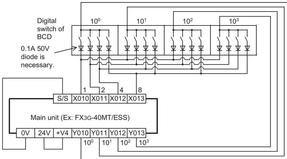
**2. Main unit + input/output powered extension unit/block**
