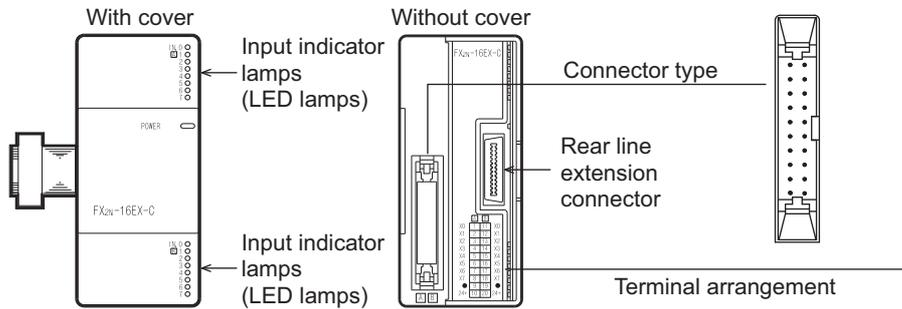
Connector pin arrangement
