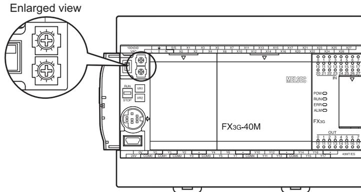
The current value of each variable analog potentiometer is stored in special data registers shown below.
