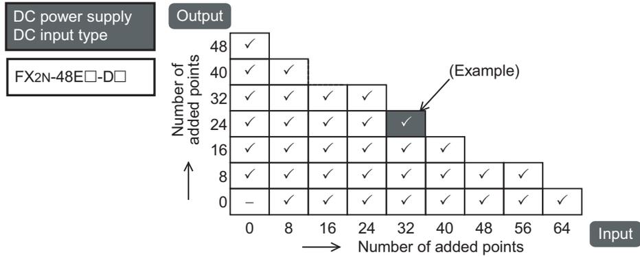
(Example) When adding 32 inputs to FX2N-48ER-DS, a maximum of 24 outputs are expandable
