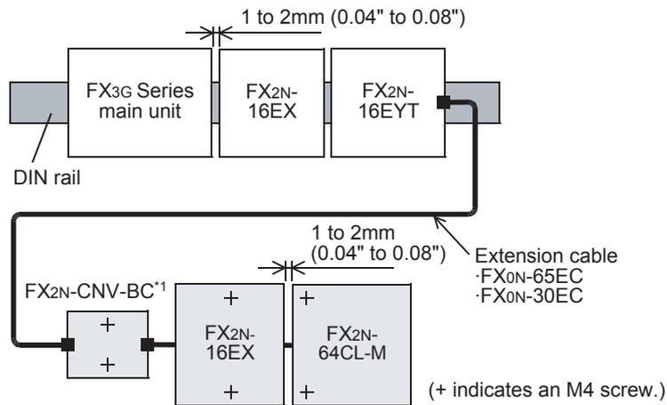
\*1. FX2N-CNV-BC can be installed directly in the enclosure but cannot be installed on the DIN rail.
