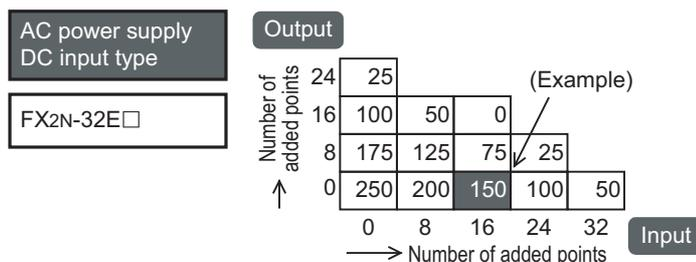
(Example) When a 16-input and 0-output point extension block is connected to FX2N-32ER-ES/UL, the current of the 24V DC service power supply becomes 150mA or less.
