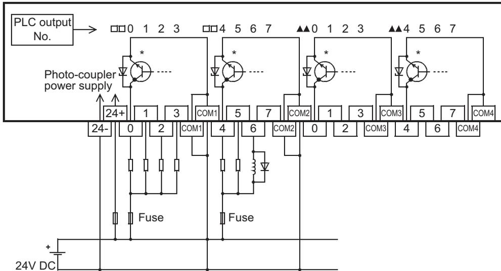
\* For the FX-16EYT-H-TB, the output transistor elements are as shown in the figure below.
