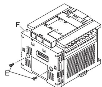
2. This paragraph explains how to connect the connector conversion adapter to the main unit.
