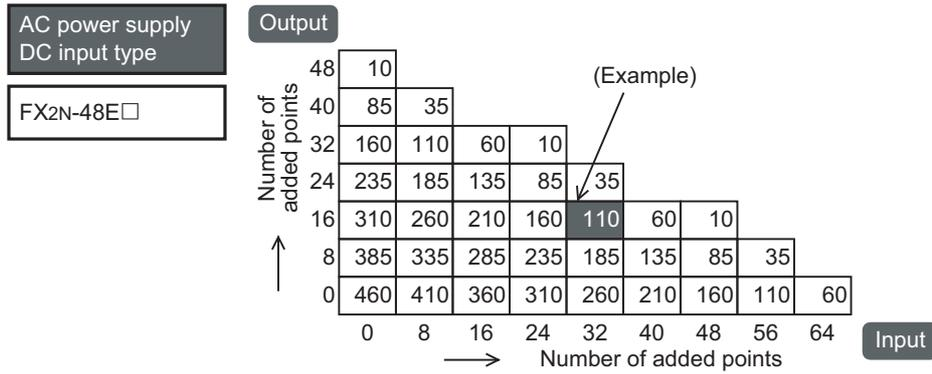
(Example) When a 32-input and 16-output point extension block is connected to FX2N-48ER-ES/UL, the current of 24V DC service power supply becomes 110mA or less.
