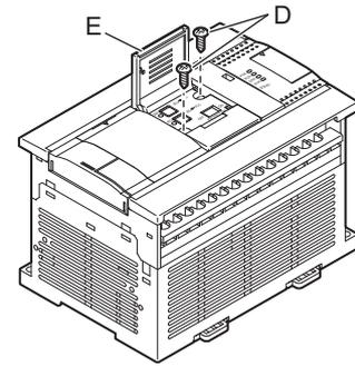
**21.3.2 Installation (when the expansion board/connector conversion adapter is used together)**
