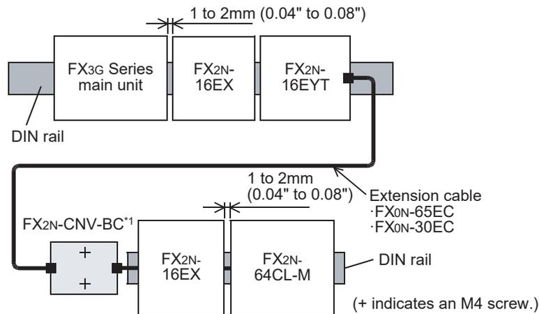
\*1. FX2N-CNV-BC can be installed directly in the enclosure but cannot be installed on the DIN rail.
