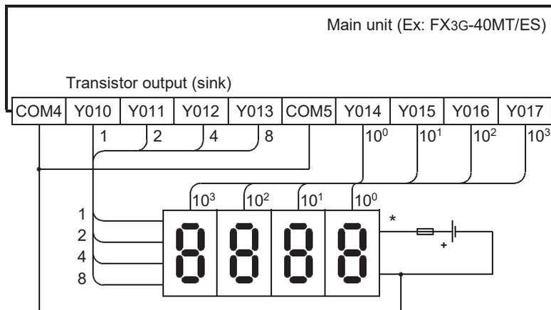
\* Use a 7-segment display with a latch and a built-in BCD decoder.
