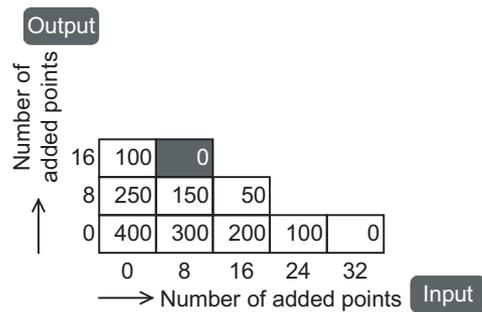
After 8 input points and 16 output points are connected, the remaining current of the 24V DC service power supply is 50mA or less. Accordingly, it is possible to add 8 input points and 16 output points.
