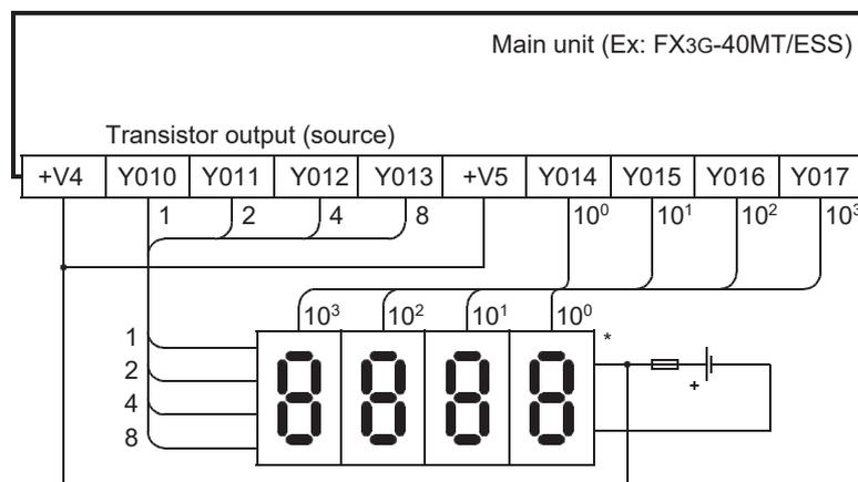
\* Use a 7-segment display with a latch and a built-in BCD decoder.
