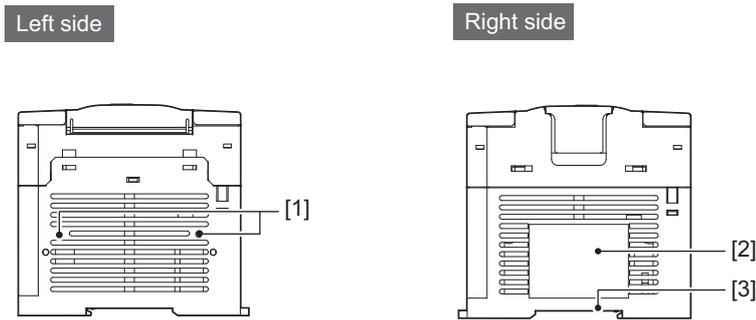
**[1] Connector conversion adapter connecting screw holes (2 places)**
