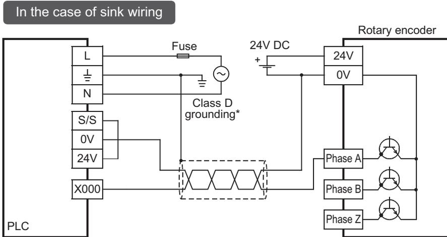
\* The grounding resistance should be 100Ω or less.
