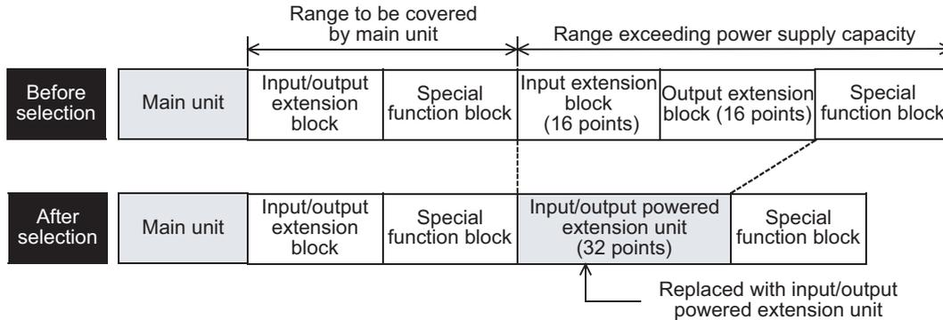
Determine whether extension devices can be connected to the input/output powered extension unit by the following method.
