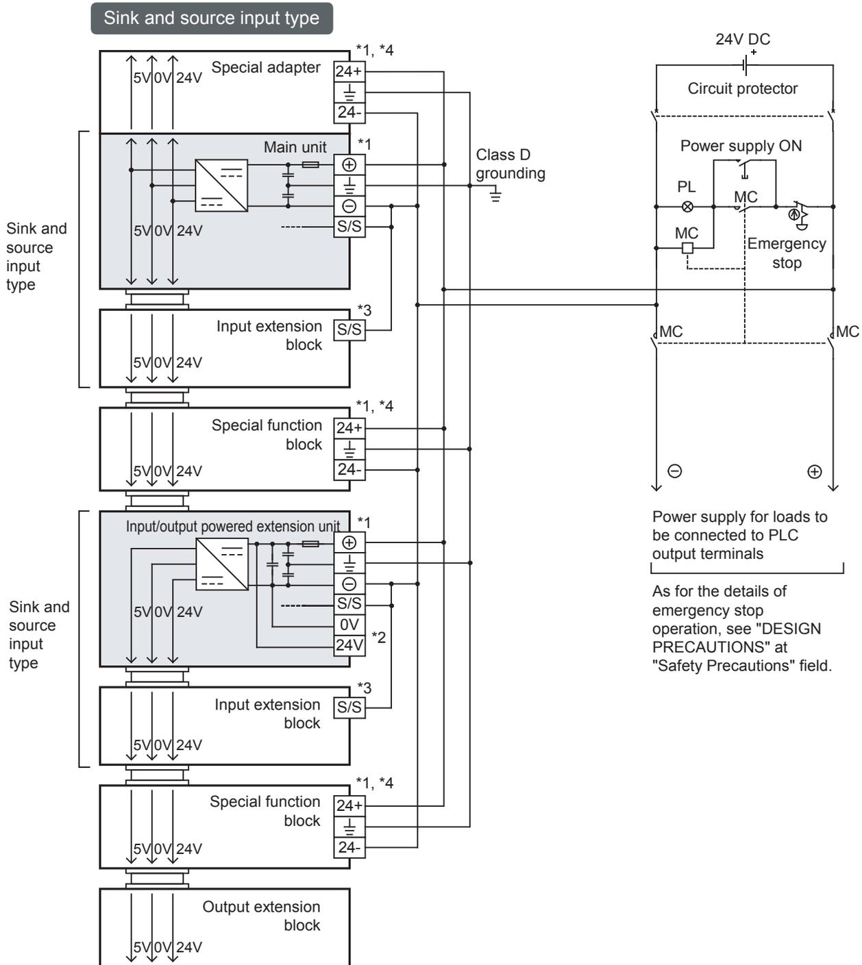
\*1 Connect DC power to [⊕] and [⊖] terminals. The same power source for the main unit, extension units, special function unit/blocks and special adapters is preferable. When using the different power source from the main unit, turn ON the peripheral devices' power simultaneously, or earlier than the main unit's. When turning OFF the power, confirm the safety of the system, and then turn OFF the power of the PLC (including special extension equipment) at the same time.
