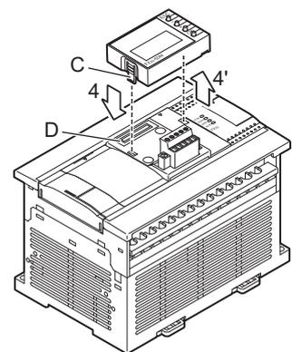
Remove the display module while pressing and holding the display module fixing hook (C in the figure on the right) as shown in the right figure (arrow 4').
