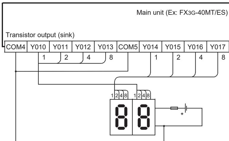
7-segment display to be used for sink wiring (in the case of transistor output)
