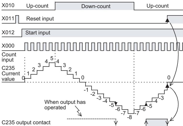
C235 is set to the up-count or down-count mode through interruption by the count input X000.
