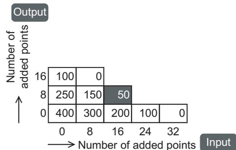
After 16 input points and 8 output points are connected, the remaining current of the 24V DC service power supply is 50mA or less. Accordingly, it is possible to add 16 input points and 8 output points. The remaining power supply capacity (50mA) can be used as a power supply for external loads (such as sensors), special adapters and special function blocks by the user.
