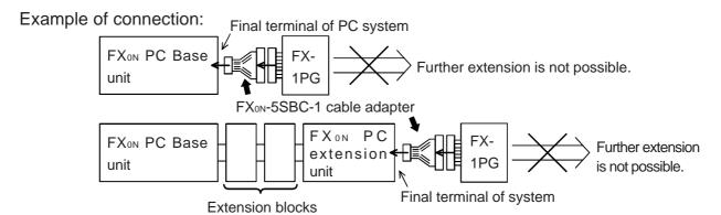
Note: • The number of FX-1PG blocks connected to the system is limited to only one.
