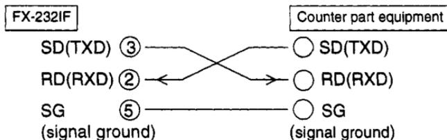
Communication is performed in accordance with the condition determined by the software in the 232IF and the counterpart equipment.
