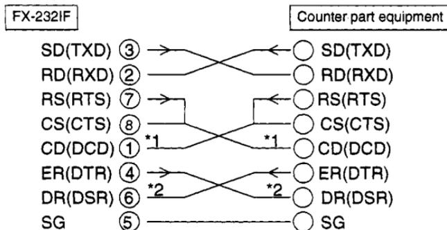
Because the carrier to send (CS) signal pin of the 232IF itself receives the request to send (RS) signal, signal transfer is performed as if the counterpart equipment is functioning.
