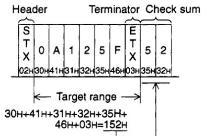
The total value including the terminator and excluding the header (1st byte of the header only) is calculated. Then, the lower 1 byte is converted into the ASCII code, and sent or received. The data converted into the ASCII code is placed in the order of upper digit and lower digit.
