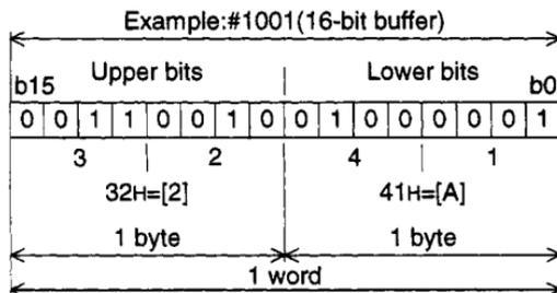
A numeric in the send/receive buffer is treated as hexadecimal (HEX).
