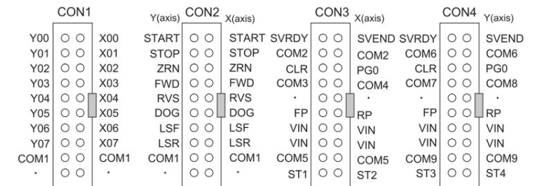
All terminals with identical names are shorted internally (Ex. COM1-COM1, VIN-VIN, etc.).
