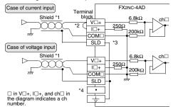
\*1 When wiring the analog output cable, use a shielded two-core twisted cable, and separate it from other power cables and cables easily affected by induction.
