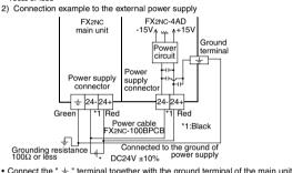
to the ground of the power supply equipped with grounding resistance of 100 $\Omega$  or less.
