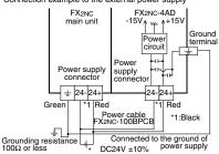
• Connect the "  $\frac{1}{2}$  " terminal together with the ground terminal of the main unit to the ground of the power supply equipped with grounding resistance of 100 $\Omega$  or less
