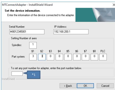
\* Entering the port No. for MTConnect Adapter of this screen is optional. Port Nos. 7878 to 7927 are set automatically to MTConnect Adapter when no port No. is set. When any port No. is entered on this screen, that port No. will be set to MTConnect Adapter.
