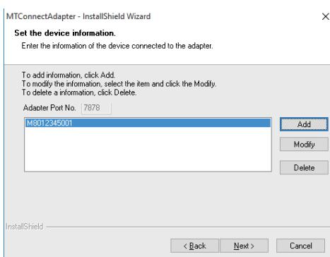
(Note) The port No. of the device selected on the list appears in the box of "Adapter Port No." Write down these port Nos. as they will be used to set MTConnect Agent.
