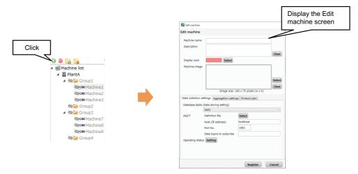
(2) After setting the necessary information in the Edit machine screen, press the [Register] button. For details on the settings, refer to "Edit machine screen" (Chapter 4.1).
