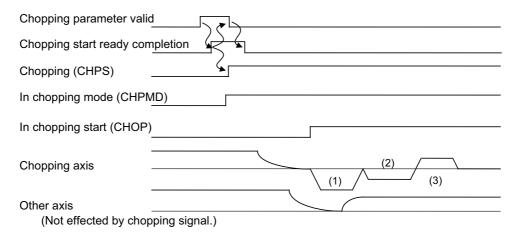
The "In chopping start" is entered after the chopping axis movement has been completed.
