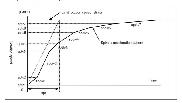
The spindle specification parameters need to be set as follows for the operation of acceleration/deceleration during the spindle-mode rotary axis control. These settings are the same as for the multi-step acceleration/deceleration under spindle synchronization control.
