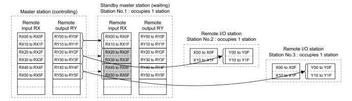
Data sent from the master station to the remote input RX and remote register RWr in the standby master station (shown by the shaded areas in the above diagram) are used as output data when the master station becomes faulty; these data should be saved in another device using the sequence program. When the master station becomes faulty, the saved data are transferred to the remote output RY and remote register RWw in the standby master station using the sequence program.
