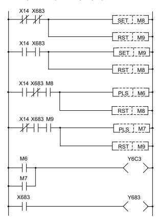
Under sequence control in the above example, the switch marks on the PLC switch screen can be operated from both external and PLC switches.
