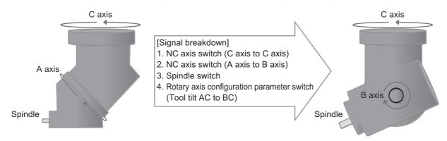
An example for the signals used to make the head swapping is as follows.
