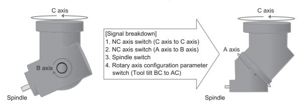
An example for the signals used to make the head swapping is as follows.
