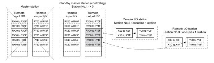
Data sent to the remote output RY and remote register RWw in the standby master station by the sequence program are then transmitted to other stations as output data.
