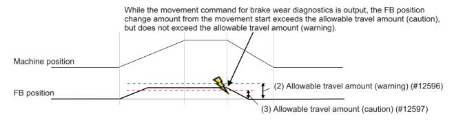
(2) Operation error (M01 0371) "Brake wear diagnostics (warning)"
