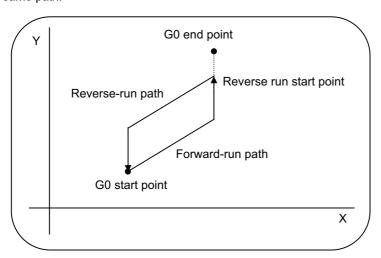
(5) During the creep distance movement in the unidirectional positioning (G60), a reverse run ends at the creep distance movement start point.
