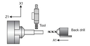
Machining process when Sub part system control is OFF
