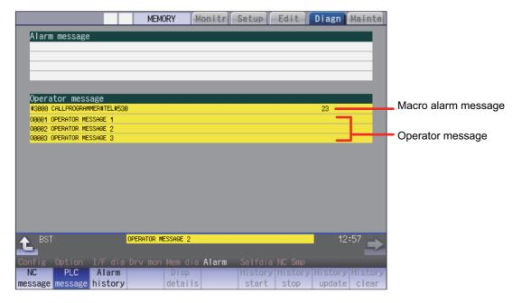
When variable #3000 is issued in the machining program, the message of the alarm No. specified by variable No. #3000 is extracted from the message file to be displayed. (Note that variable No. #3006 cannot be used to extract the corresponding message.)
