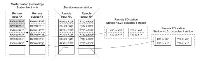
The information in the master station's shaded areas is either input or held in accordance with the setting of the network parameter "Setting of data link faulty station".
