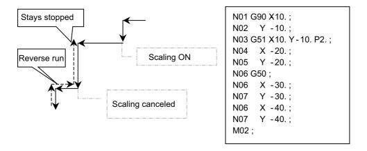
(4) Corner R/C, linear angle command and geometric command are not successfully executed during the reverse run. Corner R/C stays stopped before the corner.
