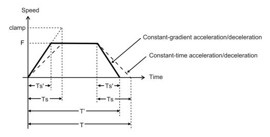
clamp : Cutting feedrate for clamp function (#2002 clamp)
