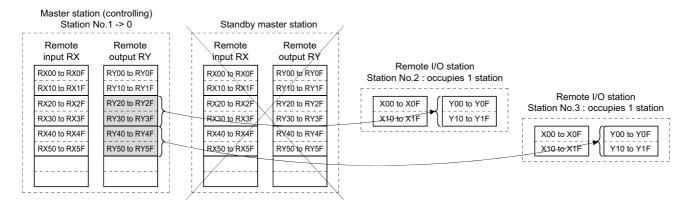
Data sent to the master station's remote output RY and remote register RWw using the sequence program are transmitted to the other station as output information.
