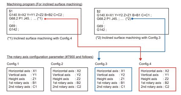
You can check the rotary axis configuration parameters being applied with rotary axis configuration parameter output (R656).
