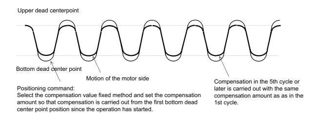
The stroke compensation completion signal is output when the difference between the commanded stroke and the actual stroke has reached the tolerance specified with the parameter (#2080 chwid).
