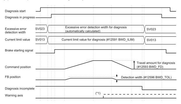
(\*1) It turns ON when the diagnostics result is in the caution state or warning state.
