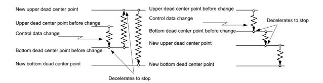
The upper and bottom dead center points are switched while moving from the bottom dead center point to the upper dead center point.
