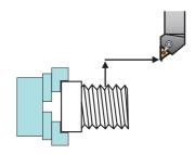
(2) Memorizing thread groove position (memorizing lead axis and spindle position)
