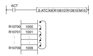
(Note 1) In this control mode, pointer always indicates "0" (tool table head).
