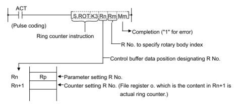
The ring counter is a binary counter; it is used as an up/down counter of "start from 0" or "start from 1" according to the parameter rotary body instruction.
