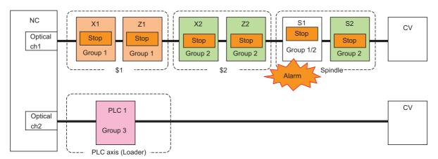
When an alarm occurs at PLC1 axis, the PLC1 axis which belong to the machine group 3 performs the alarm stop. However, other axes/spindles/PLC axes are able to continue the operation without the alarm stop.
