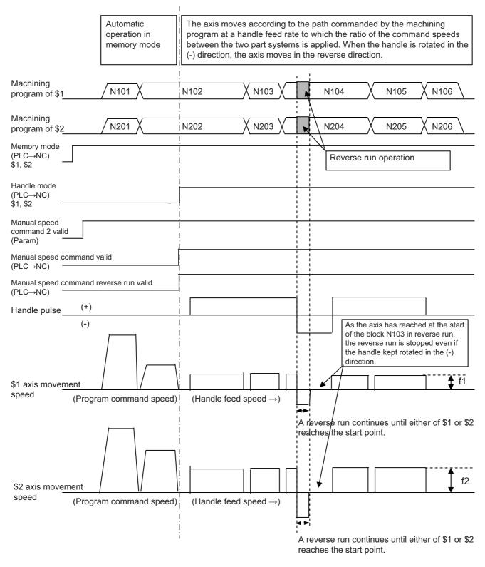
The movement speed value of f1, f2 is calculated by multiplying the command speed ratio between two part systems by the handle speed.
