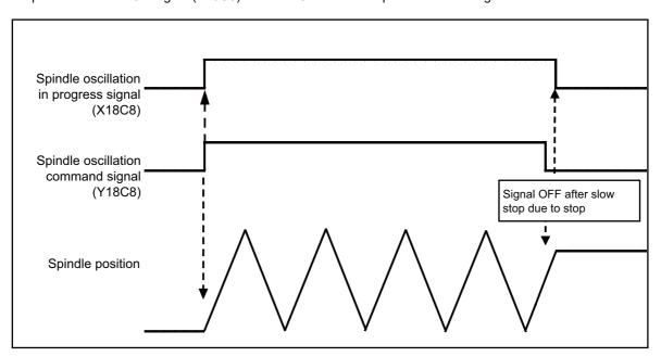
The spindle oscillates in accordance with the spindle oscillation amplitude and spindle oscillation configured to the R registers.
