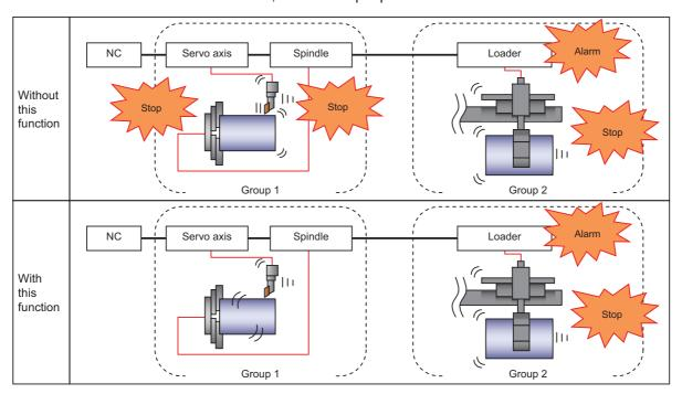
Likewise, when this function is used in a machining center system, the axes belonging to a different machine group from the axis for which an alarm has occurred can continue the operation as illustrated below. Without this function, the alarm stop is performed for all the axes when an alarm occurs.
