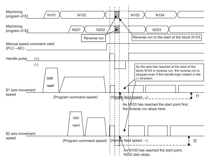
The movement speed value of f1, f2 is calculated by multiplying the command speed ratio between the two part systems by the handle speed.
