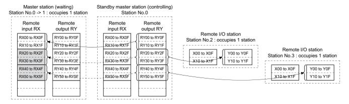
Data sent from the standby master station to the remote input RX and remote register RWr in the master station (shown by the shaded areas in the above diagram) are used as the output data in case of the standby master station's failure.
