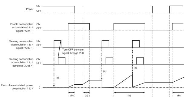
Illustrated below is a timing chart of the operation to obtain the accumulated power consumption data.
