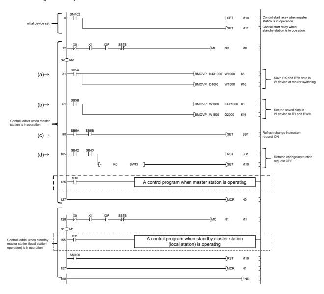
(5) When data link control is compulsorily transferred from standby master station to master station
