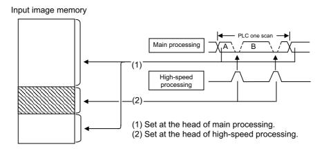
The hatched area is high-speed input designation part. Whenever the high-speed processing program runs, data is reset in the hatched area. Thus, the signal in the hatched area may change in main processing (A) and (B) because the high-speed process interrupts between (A) and (B) and re-reads the input signal in the hatched area.
