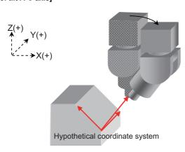
Rotary axis travel command: Rotation with the tool tip as the center
