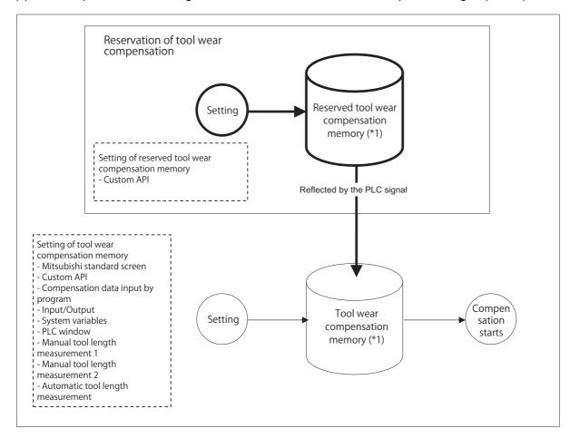
(\*1) This function supports the following types of tool wear compensation memories.
