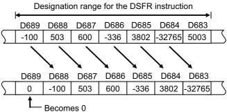
(2) The following program shifts the contents of D683 to D689 to the left when XB is ON.
