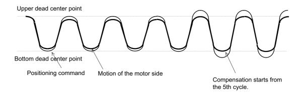
However, with this method, if the grindstone contacts with the workpiece, the chopping width before and after compensation may be differed, and which may affect the machining surface. In this case, the compensation value fixed method is appropriate.
