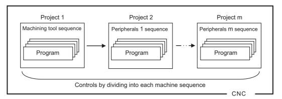
For example, when creating the sequence of machine tool and the peripherals separately, this function allows the each sequence to be created/managed in separate project. This will enable the machine to start smoothly without having the program setting error or device redundant error, because the program setting/ device can be controlled by each sequence.
