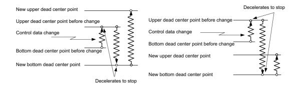
Chopping control data can be changed at any time in the chopping start state. Checking the NC side status or considering the timing is not necessary.
