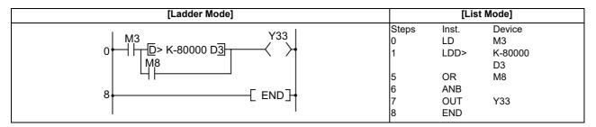
(4) The following program compares the data in D0 and D1 with the data in D3 and D4, and establishes continuity if the data in D0 and D1 is equal to or less than the data in D3 and D4.
