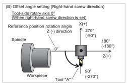
When you use any tool with the hexagon turret and "#1450 5axis\_Spec/bit3" (Select specifications of rotation direction parameter) is set to "0" (disabled), the offset angle is set as follows:
