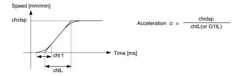
When the upper dead center point, bottom dead center point and number of cycles are set with chopping control data, the speed pattern in which acceleration a is "clamp speed/time constant" will be commanded to the servo drive unit.
