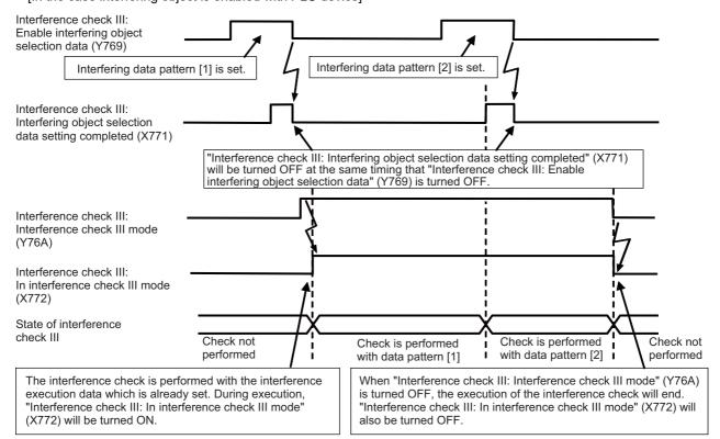
If you turn OFF and ON the "Interference check III: mode" signal, the interfering data you set lastly is used for the interference check between interfering objects.
