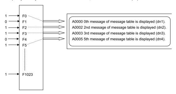
The highest priority is assigned to the F0 signal. The message corresponding to Fn set to "1" is fetched from the message table and displayed in order starting at F0. If no messages are prepared or Fn without prepared message is set to "1", the message "USER PLC ERROR n" is displayed.
