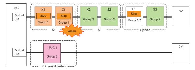
When an alarm occurs at S1 spindle, the axes/spindles which belong to the machine group 1 and 2 perform the alarm stop. However, other PLC axes are able to continue the operation without the alarm stop.
