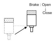
[Step1] Move to the brake wear diagnostics start position. Then, apply the brake. (Ladder)
