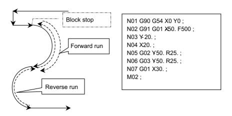
(3) If the "Automatic operation "start" command" signal is turned ON and OFF during the automatic operation pause, the forward run starts after the execution for the remaining distance of the command. Therefore, the forward run usually must be started during the automatic operation stop.
