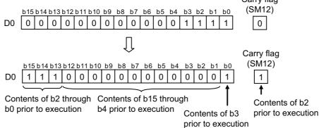
(2) The following program rotates the contents of D0, including the carry flag, 3 bits to the right when XC is ON.
