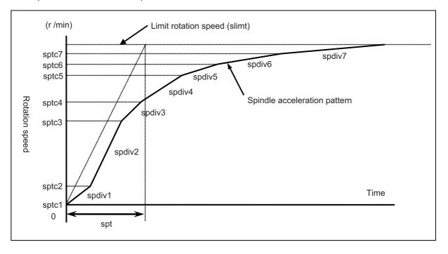
To specify the acceleration and deceleration of spindle-mode servo motor control, configure the following spindle spec. parameters.
