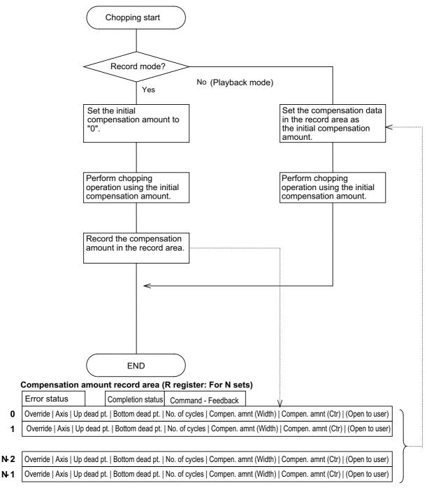
14 R registers are required per one set. For N sets, the number of R registers required is 14\*N+4.
