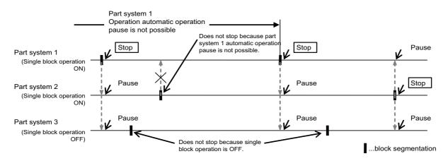
In this case, the system enters the cycle operation suspension disabled state and so cycle operation is not suspended.
