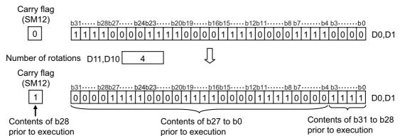
(2) The following program rotates the contents of D0 and D1, including the carry flag, 4 bits to the left when XC is ON.
