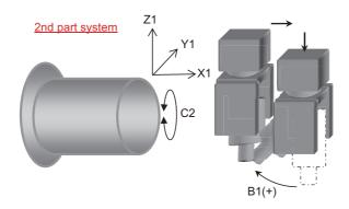
position where the rotary axis angle is 0°.
