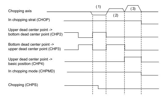
The "In chopping start" and the "In chopping mode" signals are turned OFF after returning to the basic position completes.
