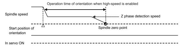
By enabling the high-speed proximity switch method orientation (parameter "#3128 ori\_spec/bit1" = "1"), the high-speed function is valid.
