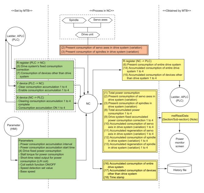
(Note) The use of custom API library function (melReadData) allows you to obtain the present power consumption data and accumulated power consumption data.
