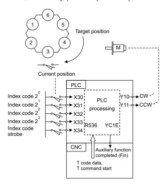
In the example of ladder circuit shown below, the rotation direction is determined by the T command and current position data given by the machine, and the rotary body is rotated in that direction until the target position reaches the current position. When indexing is completed, the auxiliary command completion signal is turned ON.
