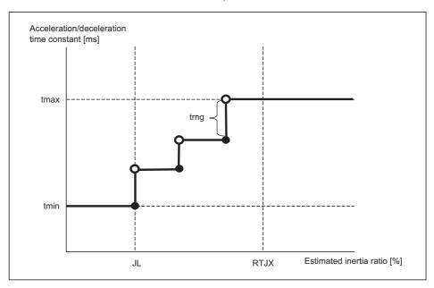
tmax: Maximum value of switching time constant tmin: Minimum value of switching time constant
