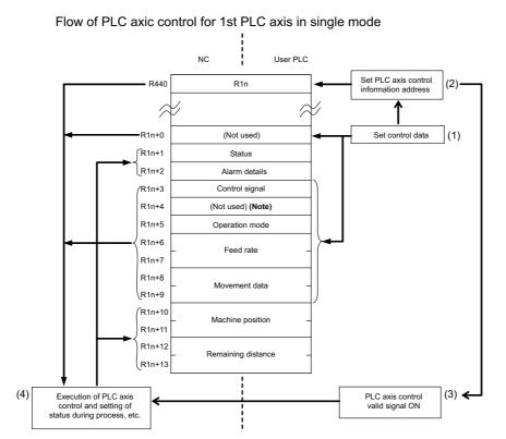
(Note) Refer to "(4) Axis specification" in "Details of PLC Axis Control Information Data" for the explanation of unused register No. R1n+4.
