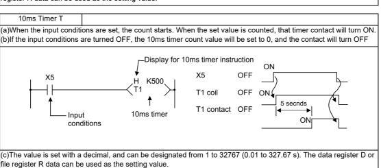
(2) With the device T, the contact/coil is handled as bit device, and the current value is handled as word device. In the function instructions described after, the word device T indicates the current value even if there is no description about it.
