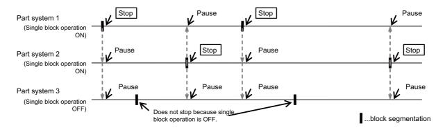
For the following scenario, the stopping of single block operation is disabled and so single block operation does not stop.
