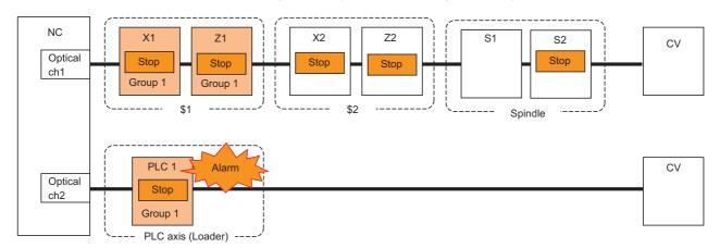
When an alarm occurs at Z2 axis, only the axes which are set to "0" and "FF" in the machine group numbers perform the alarm stop. Although the S1 spindle is the machine group "0", S1 continues the operation because "#3197 mgrspnum2 (Spindle machine group No. 2)" is set to "00".
