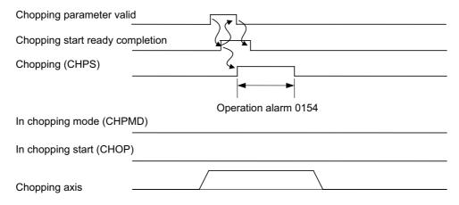
In the handle mode, when the chopping axis is not selected for the handle axis, the chopping operation is started at the rising edge of the "Chopping" signal.
