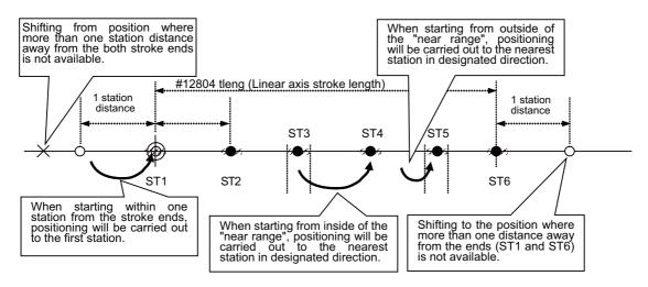
[Special operation of linear axis in uniform assignment]
