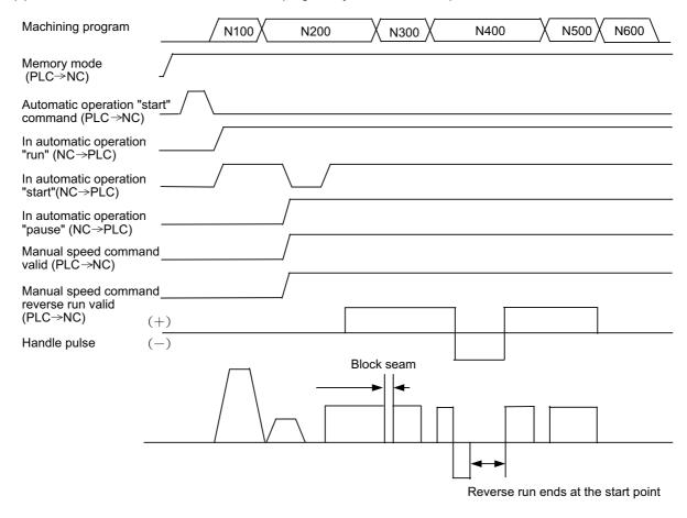
(Note) When the reverse run is not valid, the movement follows the machining program, not the handle feed direction.
