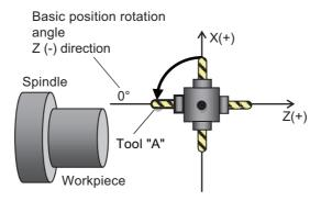
Rotate the target tool by the basic position rotation angle, then issue G174/G53.1 command.
