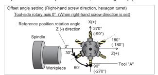
In the R address of the G174/G53.1 block and R register, specify the tool angle relative to the reference position rotation angle when the tool axis rotation angle is at 0 degree. Thus, even when the tool axis rotation angle rotates and the tool axis rotation angle of the target tool is not at 0 degree, make sure to designate the offset angle at which the tool axis rotation angle is at 0 degree, for the tool axis rotation angel compensation amount.
