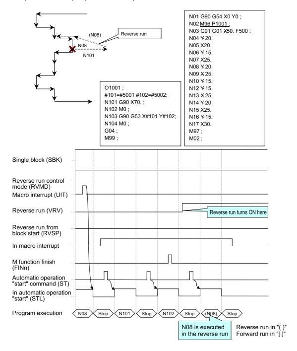
(b) In a macro interrupt program, start a reverse run at the point (or the block start point) where the interruption occurs and which a M99 (complete sub program) block follows.
