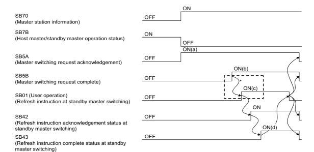
\* When SB5B is turned ON, the sequence program switches RX to RY and RWr to RWw. In addition, SB01 is turned ON by the sequence program. (Enclosed with dotted lines)
