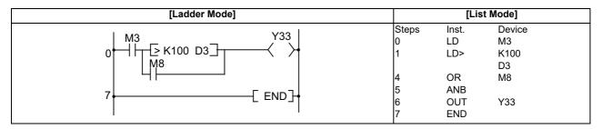
(4) The following program compares the data in D0 and D3, and if the data in D0 is equal to or less than the data in D3, establishes continuity.
