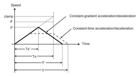
clamp : Cutting feedrate for clamp function (#2002 clamp)
