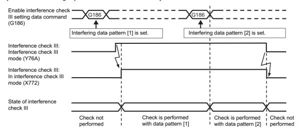
[In the case interfering object is enabled with PLC device]
