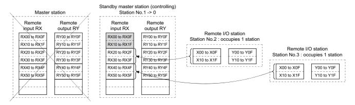
Data in the standby master station's shaded areas are either input or retained in accordance with the parameter "Setting of data link faulty station".
