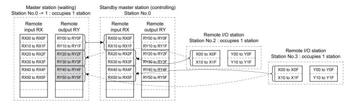
Data sent to the master station's remote output RY and remote register RWw are used by the master station as input information to operate the local stations. Thus, there is no need to save these data in another device.
