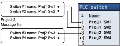
The PLC switch names described in message files of each project are combined and displayed.
