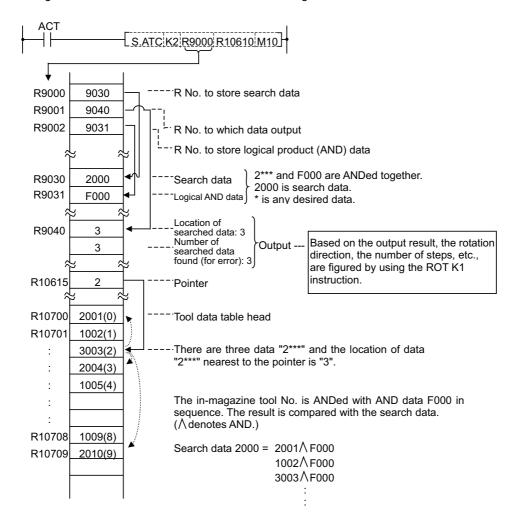
(Note 1) Pointer and location are counted up, like 0, 1, 2 .... 9, in the tool data table, starting from the tool data table head.
