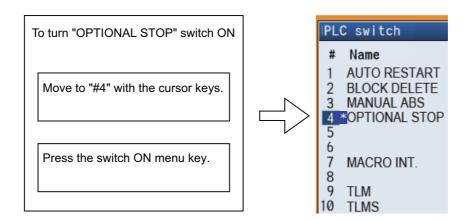
To display the switch validity state, etc., the switch name can be highlighted. To do this, turn ON or OFF output device Y corresponding to the switch name.
