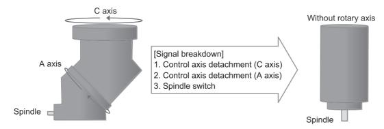
An example for the signals used to make the head swapping is as follows.
