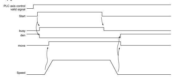
(Note) The axis moves by jog feed only during start ON.
