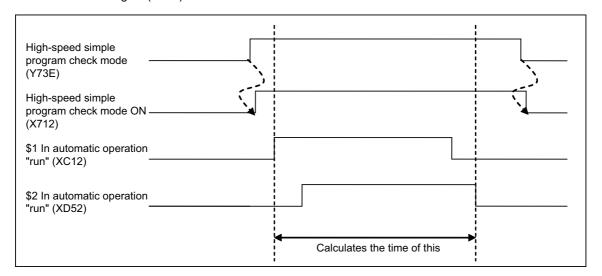
(2) Operation sequence (turning ON the high-speed simple program check mode signal (Y73E) while any part system is in cycle operation).
