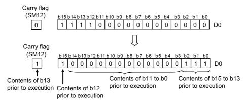
(2) The following program rotates the contents of D0, including the carry flag, 3 bits to the left when XC is ON.
