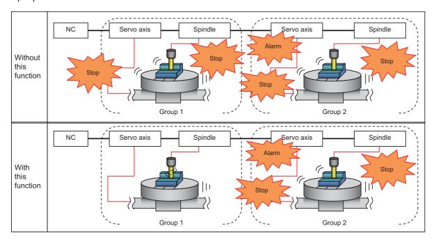
(Note) The machining group number can be set for each servo axis and spindle in this function, and incorrect setting may lead to accidents. Set the machine group number with enough care.
