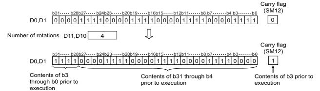
(2) The following program rotates the contents of D0 and D1, including the carry flag, 4 bits to the right when XC is ON.
