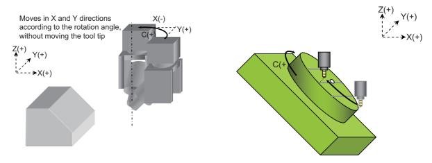
Select the hypothetical coordinate system from among the table, feature or tool axis coordinate system. If not selected, standard manual feed and interruption are carried out in the machine coordinate system.
