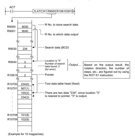
(Note 1) Pointer and location are counted up, like 0,1,2...9, in the tool data table, starting from the tool data table head.
