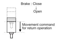
[Step3] Return the command till the brake wear diagnostics start position. (NC operation) Then, release the brake. (Ladder)
