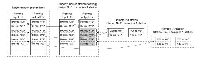
Data sent to the remote output RY and remote register RWw in the standby master station are used as input data by the standby master station when local stations are operating; thus these data don't need to be saved in another device.
