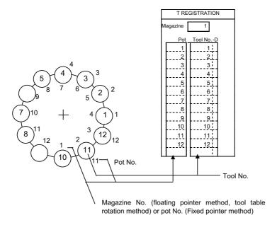
When the floating pointer method or tool table rotation method is selected on the tool registration screen, correspondence display between the magazines and tools changes each time the magazine rotates; when the fixed pointer method is selected, it does not change.
