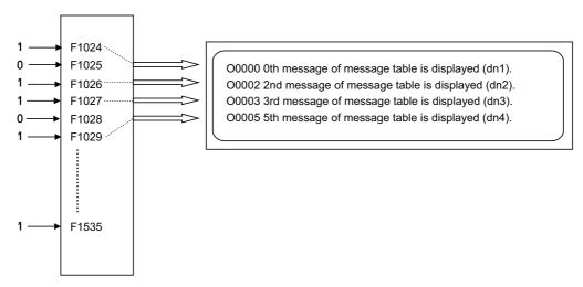
The highest priority is assigned to the F1024 signal. The message corresponding to Fn set to "1" is fetched from the message table and displayed in order starting at F1024. If no messages are prepared or Fn without prepared message is set to "1", the message "USER PLC ERROR n" is displayed.
