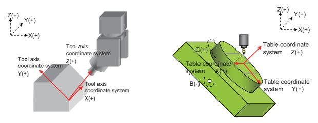
"Rotation with the tool tip as the center" is applied to a rotary axis travel command. The manual feed is carried out using the rotary axes and the three linear axes so that the positional relationship between the workpiece and tool tip can be kept.
