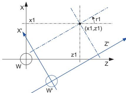
With spinning around on the center coordinate of the rotation (x1, z1), the rotation takes place in the counterclockwise direction by the angle designated in rotation angle r1.
