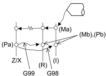
G83 (G87) X(z)\_\_\_ C\_\_\_ Z(x)\_\_\_ R r Pp F f Kk Mm ;
