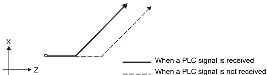
(Example 2) When the next block is a one-axis movement command with absolute position
