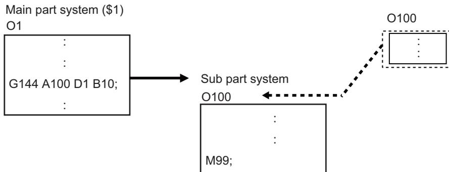
**Sub part system activation with the completion wait method (D=0)**
