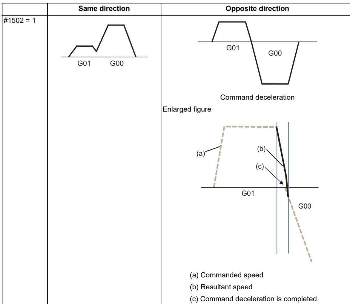
Example of program: When there is a deceleration check in the movement of several axes
