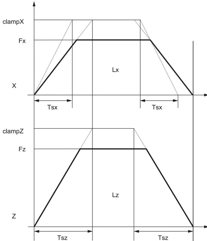
$T_{sx}$  : X axis acceleration/deceleration time
