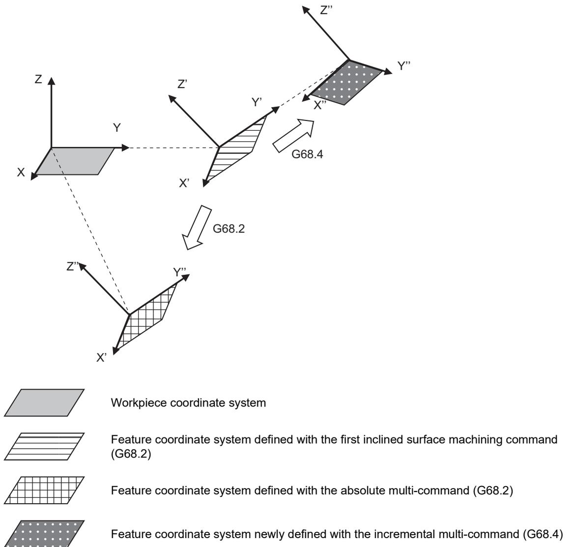
Furthermore, the inclined surface machining multi-command can also be issued to the feature coordinate system defined with the inclined surface machining multi-command. There are no restrictions regarding the nesting level.
