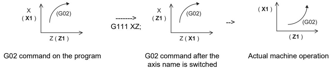
(6) The plane selection will return to the state before G111 is commanded by canceling the axis name switching.
