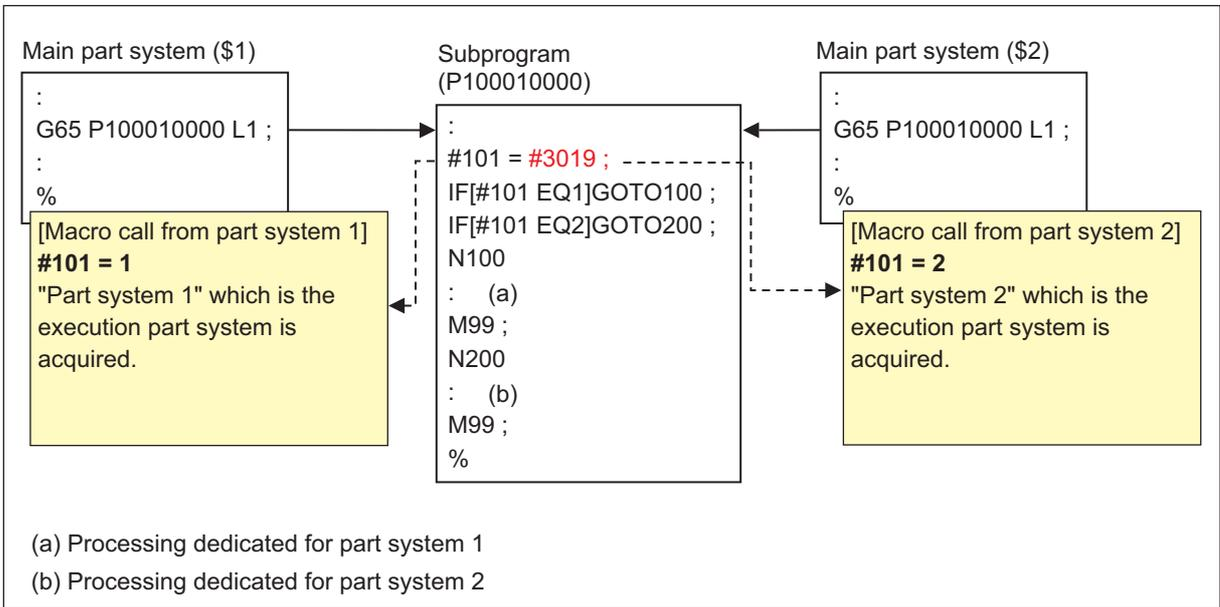
(Example 2) Example of combined operation of sub part system control II (G144) and #3019
