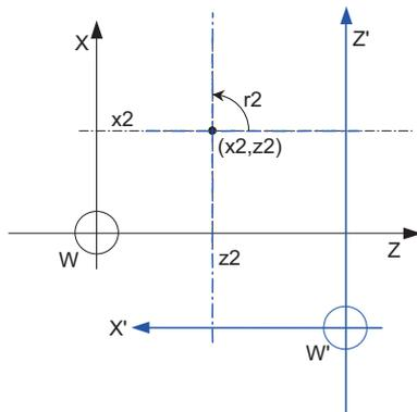
The center coordinate of the rotation switches from  $(x_1, z_1)$  to  $(x_2, z_2)$ , and the rotation angle is cleared once. Then the rotation takes place in the counterclockwise direction by the angle designated with  $r_2$
