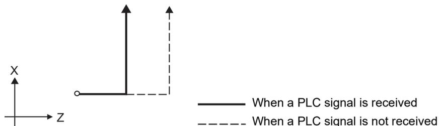
(Example 3) When the next block is a two-axis movement command with absolute position
