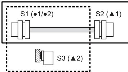
1st set: Spindle synchronization I command [S1(●1) - S2(▲1)]
