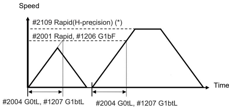
(\*) When "#2109 Rapid(H-precision)" (rapid traverse rate for high-accuracy control mode) is set to "0", "#2001 rapid" is used.
