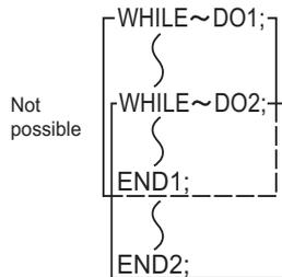
(8) Branching externally out of the WHILE - DOm range, is possible.
