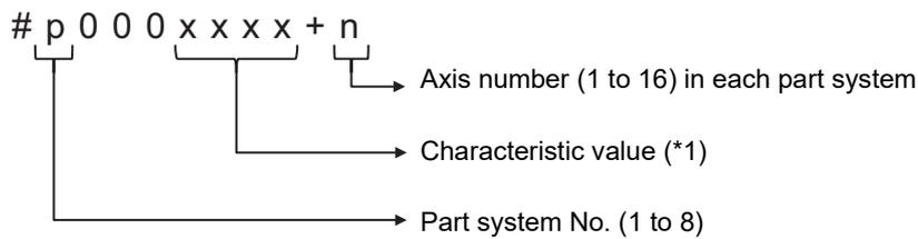
(\*1) System variable number of the variable to acquire the position information by part system. Refer to "23.11 System Variables (Position Information by Part System)".
