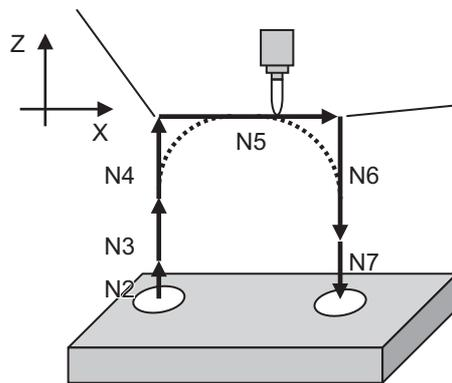
X axis in-position width is set to 1 mm with the J address command.
