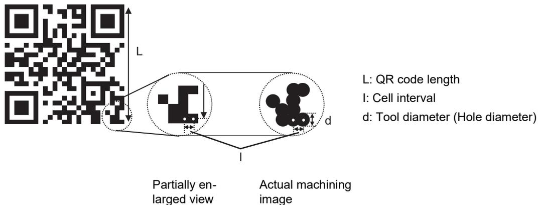
To machine a QR code that is easy to recognize, the tool diameter (hole diameter) must be approximately 1.0 to 1.1 times the cell interval, and an unmachined surface of 4 cells (cell interval  $\times$  4) or more must be secured around the QR code. The adjustment method is as follows.
