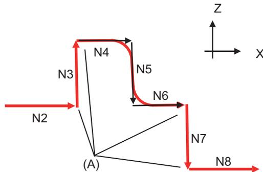
(A) These are the start and end points of movement where the compensation amount is changed by G43/G49; therefore, the rapid traverse block overlap function is invalid.
