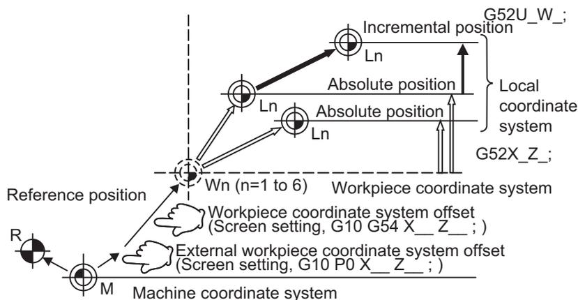
(2) The G52 command is valid until a new G52 command is issued. In the G52 command block, no movement is performed. This command, G52, comes in handy for employing another coordinate system without changing the zero point positions of the workpiece coordinate systems (G54 to G59).
