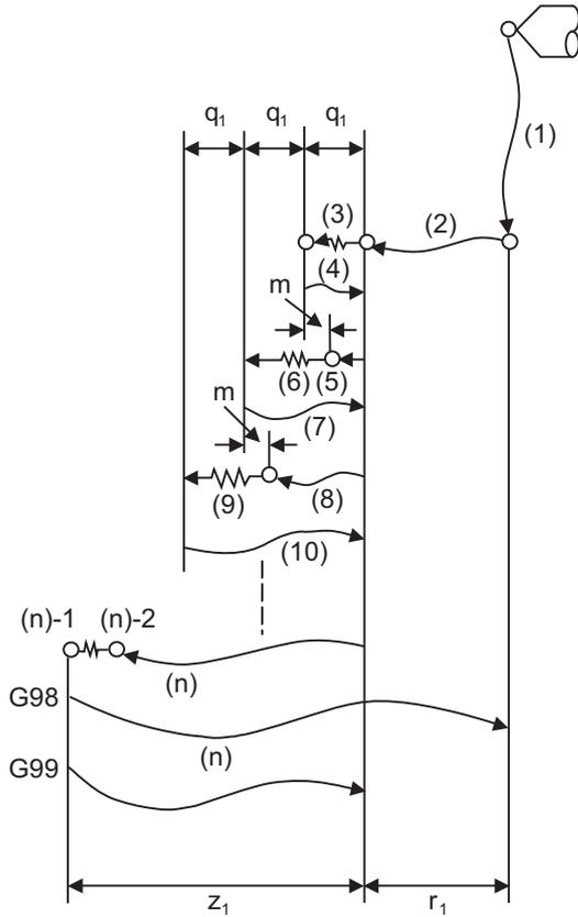
"m" will differ according to the parameter "#8013 G83 n". Program so that " $q_1 > m$ ".
