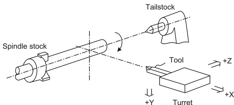
Since coordinates based on the right hand rule are used with a lathe, in the above figure, the positive direction of the Y axis which is at right angles to the X-Z plane is downward.
