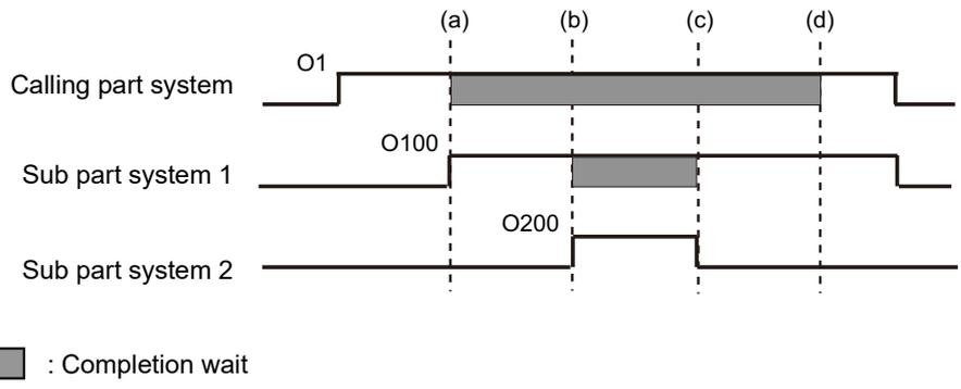
**Sub part system activation command to a sub part system being activated**
