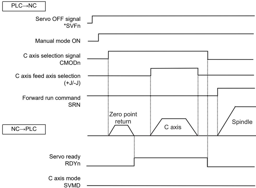
If the C axis selection signal (CMOD) is changed while either the C axis mode or spindle mode is selected in the program command method, the mode is set as follows. The mode is not switched to the C axis mode or spindle mode in the program command method during automatic running when the C axis selection signal is turned ON. Switching follows the state of the C axis selection signal (CMOD).
