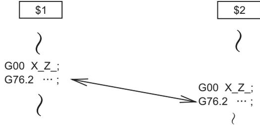
(2) G76.2 assumes the same thread cutting, and deeply cuts in with the cutting amount using 1st part system and 2nd part system alternately.
