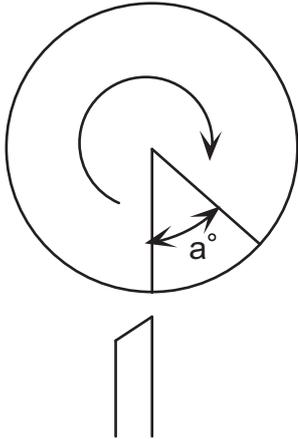
The thread cutting command starts movement after waiting for the spindle encoder's one rotation synchronization signal. However, the start point can be delayed by a degree amount.
