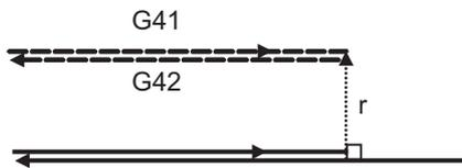
(5) When the compensation direction is switched using G41/G42, the arc may exceed 360°.
