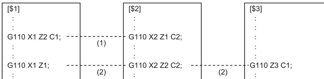
(1) 1st part system and 2nd part system execute timing synchronization operation with each other, and Z1 axis is switched with Z2 axis. Timing synchronization operation is not executed for 3rd part system as all axes of 1st part system and 2nd part system can mix due to 1st part system and 2nd part system's G110 commands.
