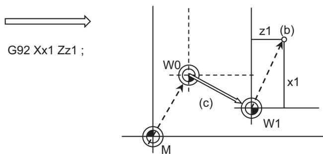
A workpiece coordinate system in which the current tool position is set at (x1, z1) will be newly created.
