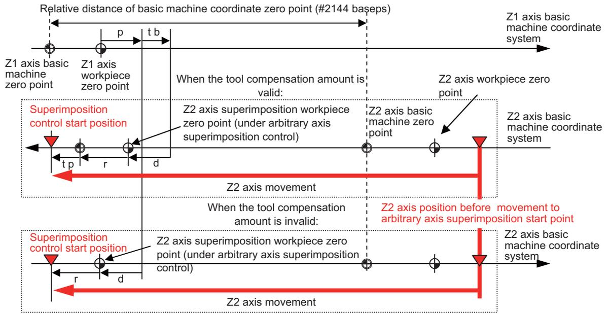
**Operation during arbitrary axis superimposition (workpiece coordinate system)**
