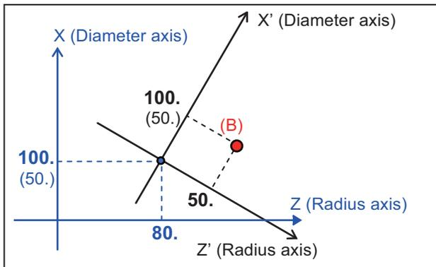
A position command given during the simple inclined surface control mode specifies a position in feature coordinate system.
