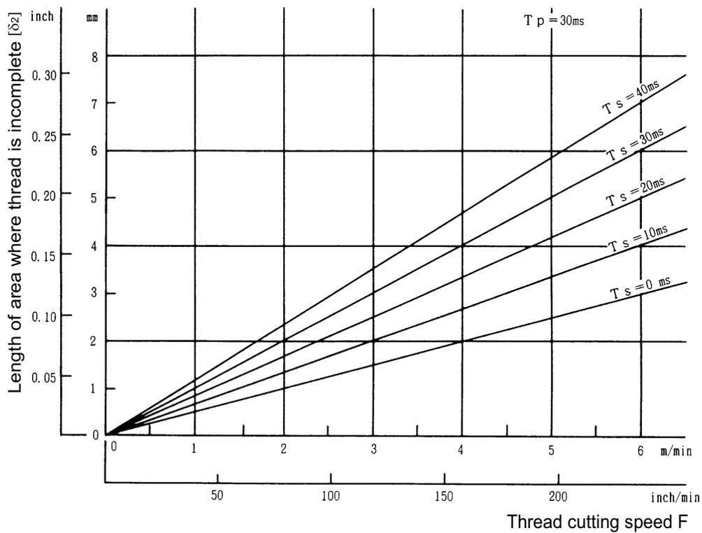
Chart to calculate length of area where thread is incomplete [ δ<sub>2</sub> ]
