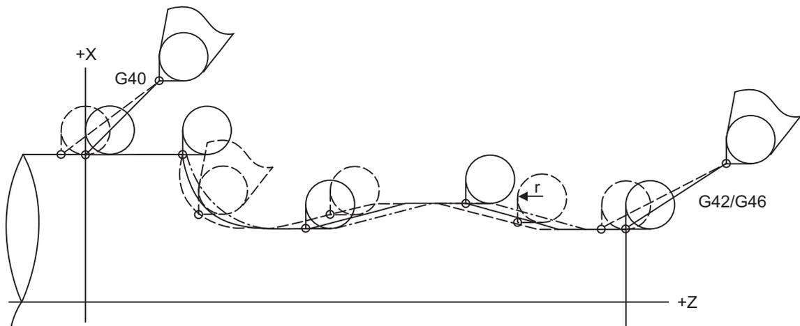
————— Programmed path or machining shape with tool nose radius compensation
