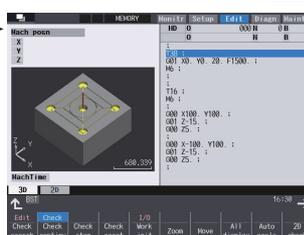
Update the drawing with the material shape changed by the machining program. Then, the machining status is initialized.
