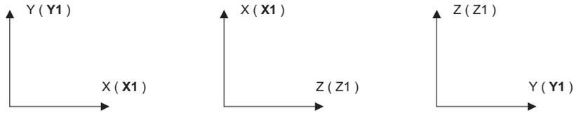
(Ex.2) Plane where axis name switching "G111 X Y ;" is carried out
