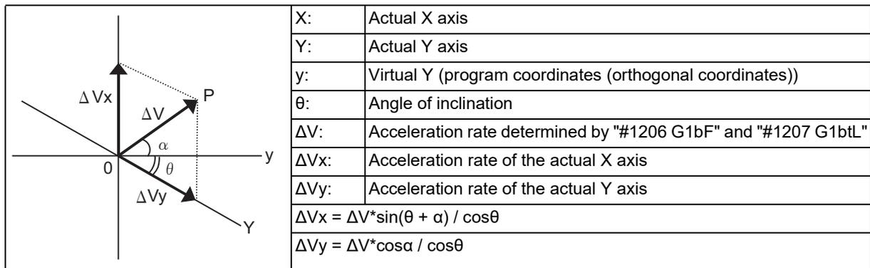
As suggested by the above equations, the maximum acceleration rate of the actual X axis ( $\Delta Vx$ ) and the maximum acceleration rate of the actual Y axis ( $\Delta Vy$ ) respectively take the maximum value when the following equations are true:
