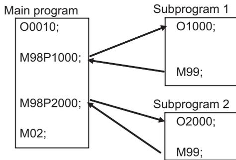
Fixed sequences or repeatedly used parameters can be stored in the memory as subprograms which can then be called from the main program when required.
