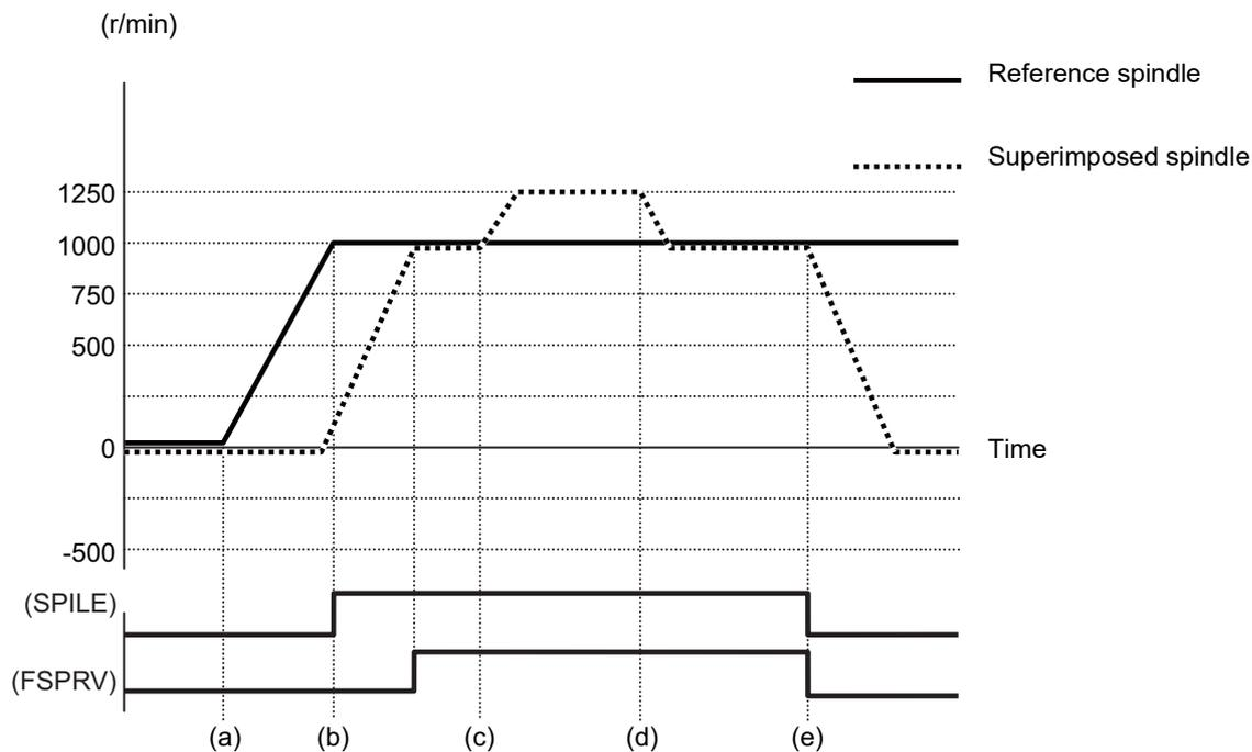
SPILE (Under spindle superimposition control mode): Setting ON outputs the PLC signal indicating that the spindle is in the spindle superimposition control mode.
