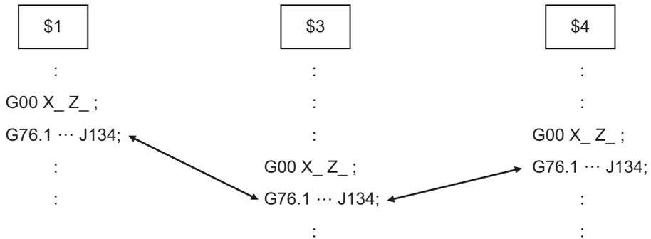
Thread cutting will start simultaneously after waiting for the 1st, 3rd, and 4th part systems.
