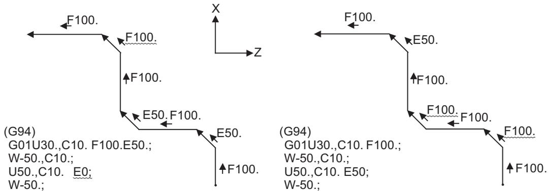
(4) E command modal is not cleared even if the reset button is pressed. It is cleared when the power is turned OFF. (In the same manner as F commands.)
