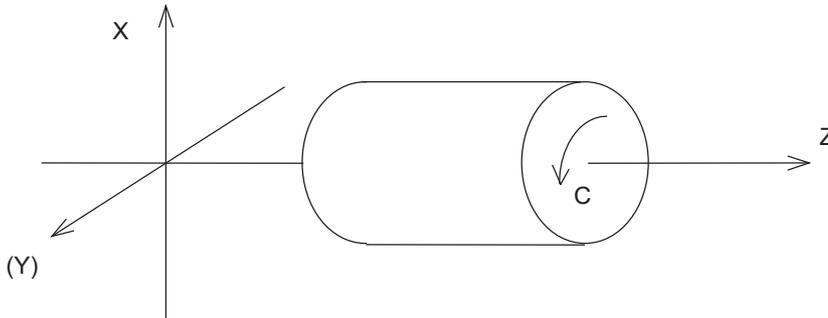
G12.1 command starts a milling and G13.1 command cancels the milling to return to a normal turning.
