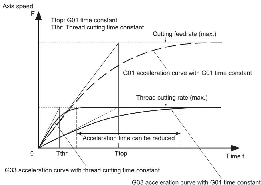
When executing the thread cutting command or executing the thread cutting command in the thread cutting cycle, carry out feed axis acceleration/deceleration in accordance with the MTB settings (thread cutting time constant parameter "#2620 thr\_t"). The following shows the operation when a G33 or G34 command is issued.
