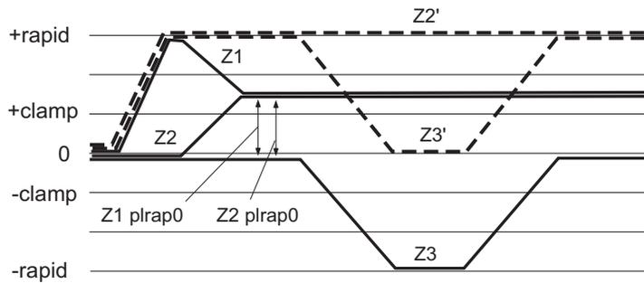
(c) Z1 Rapid traverse, Z2 Rapid traverse, Z3 Rapid traverse (all axes in the same direction)
