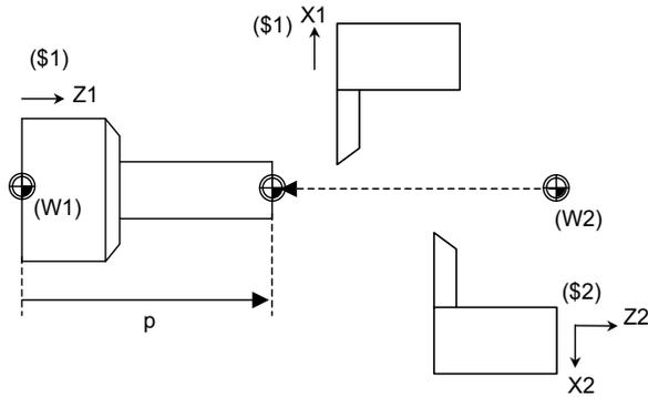
The following figure shows the relationship between the workpiece zero point of Z2 axis superimposition and the address P when the axis superimposition start is commanded in a case where (a) relative polarity is present and a case where (b) relative polarity is absent.
