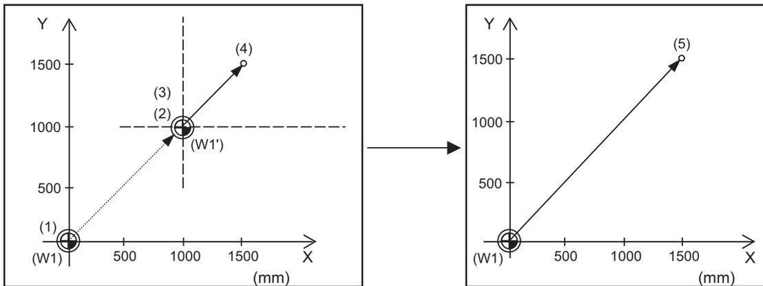
(W1) Workpiece coordinate zero point
