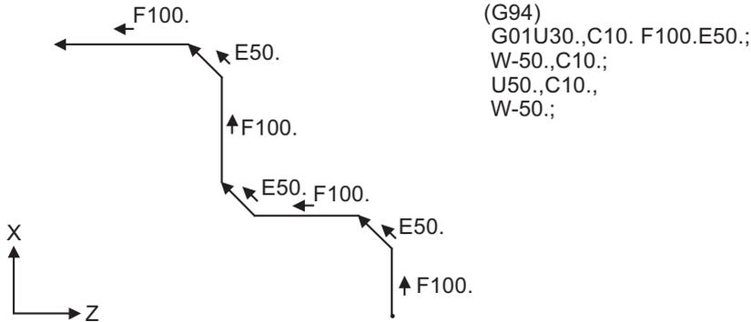
(2) E command modal has separate asynchronous feedrate modal and synchronous feedrate modal functions. Which one is validated depends on the asynchronous/synchronous mode (G94/G95).
