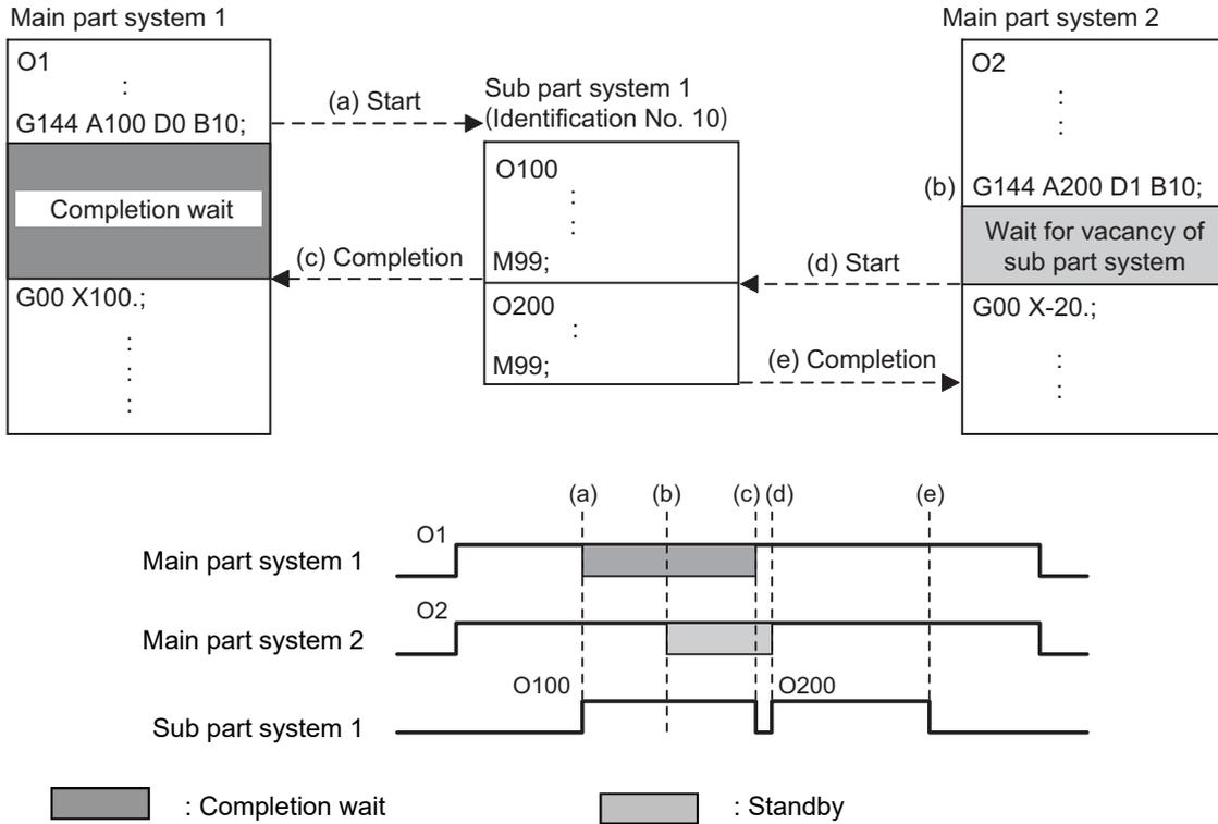
**Using a normal part system as a sub part system**
