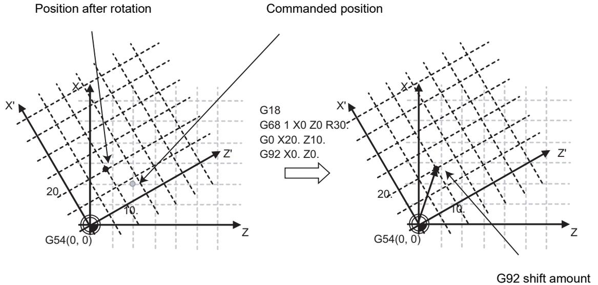
(2) When "#19003 PRG coord rot type" is "1", the position is preset to the current position commanded on the coordinate system before rotation. The coordinate system is rotated after the position is commanded.
