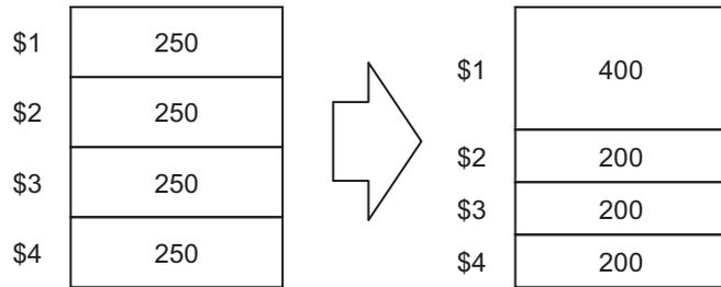
(b) When the number of tool life management sets is set to "0 sets" for the 3rd part system (\$3) of 3-part system to use that part system as an auxiliary-axis part system
