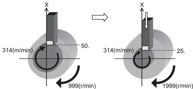
To keep the surface speed constant, this function obtains and automatically adjusts the spindle rotation speed in accordance with the movement of the tool nose point.
