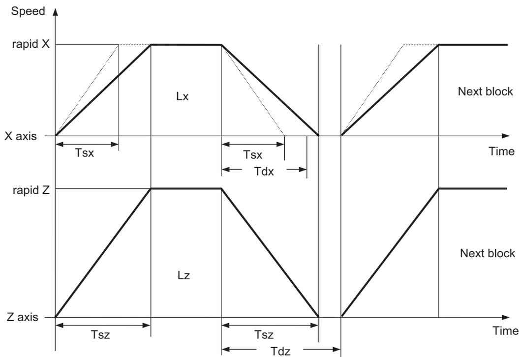
When the result is " $T_{sx} < T_{sz}$ ", the acceleration/deceleration time ( $T_s$ ) of this block is set to  $T_{sz}$  (acceleration/deceleration time of the Z axis).
