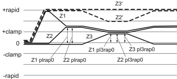
(b) Z1 Rapid traverse, Z2 Rapid traverse, Z3 Rapid traverse (only Z3 in the opposite direction)
