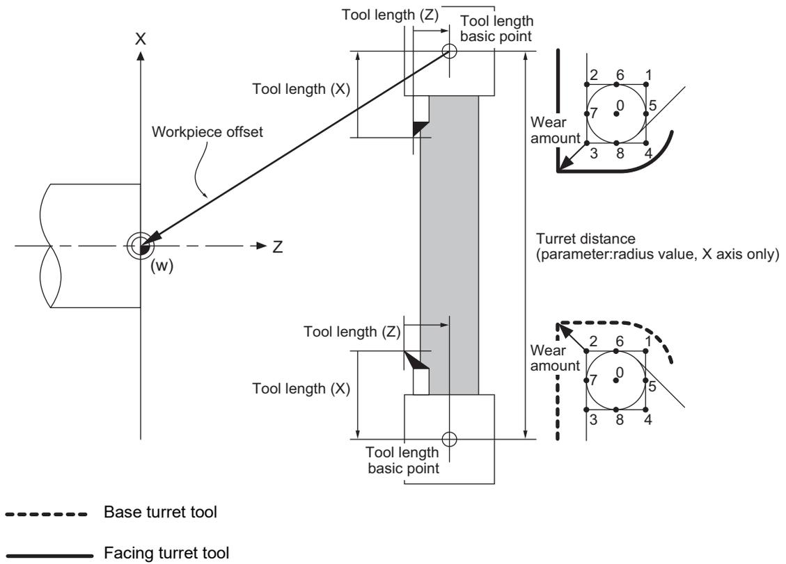
The original tool direction for the facing turret is shown in the drawing.
