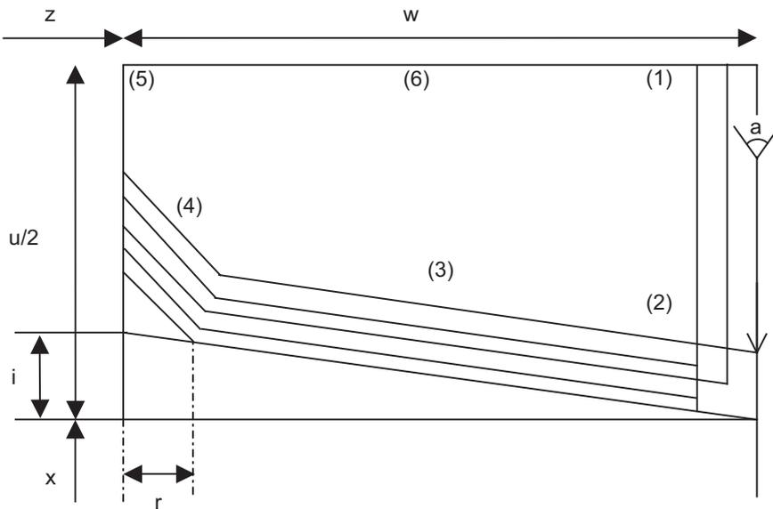
$i$  : Taper height component (radius value) for thread
