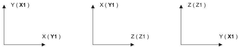
(5) Circular interpolation, nose R and fixed cycle are carried out on the selected plane.
