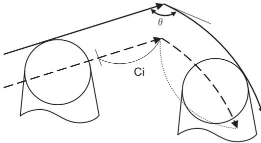
For straight lines, the override set in the parameter (#8007) is applied in the deceleration range Ci.
