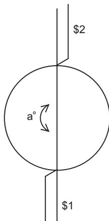
As shown on the left, if the 1st and 2nd part system blades oppose at 180 degrees, the 1st and 2nd part systems thread cutting start shift angle difference is set to 180 degrees.
