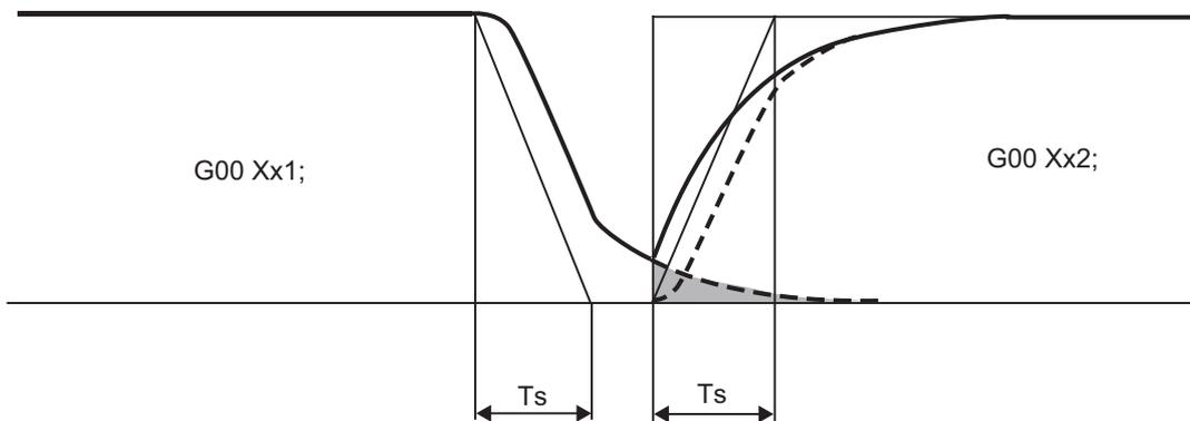
Ts : Cutting feed acceleration/deceleration time constant
