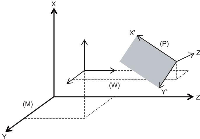
(M) Machine coordinate system    (P) G68.1 Program coordinate system    (W) Workpiece coordinate system
