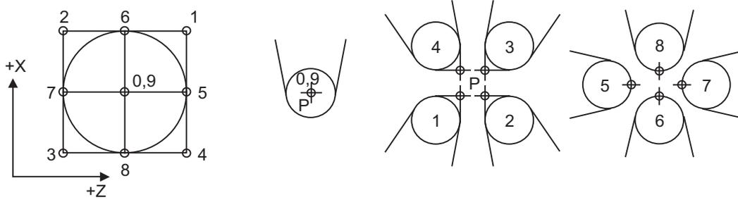
Tool nose point and compensation operation
