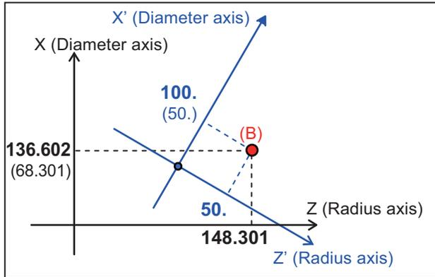
Point (B) in the left-side figure indicates the position (X136.602, Z148.301) on the workpiece coordinate system before rotation.
