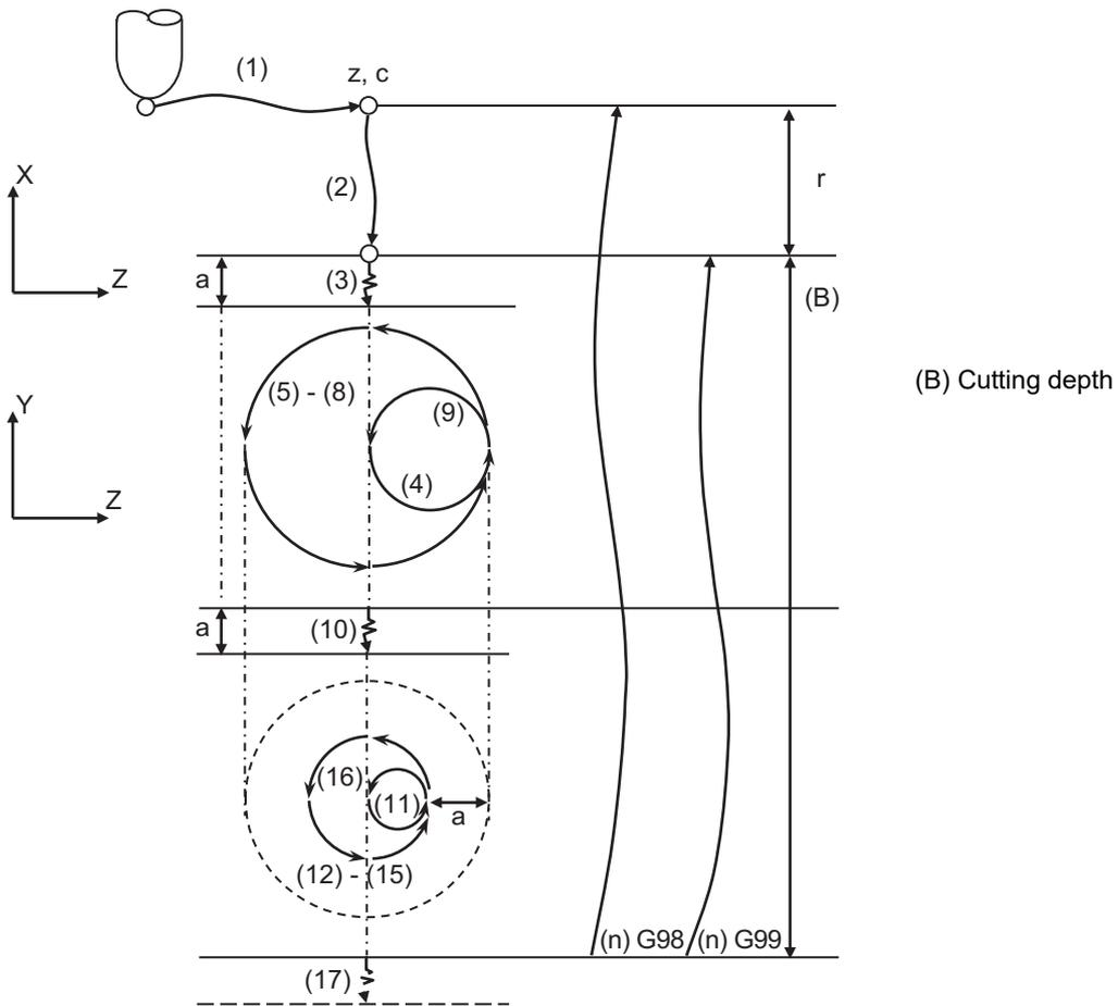
The cutting depth (B) is automatically determined by P (chamfering width) and J (ball end mill radius).
