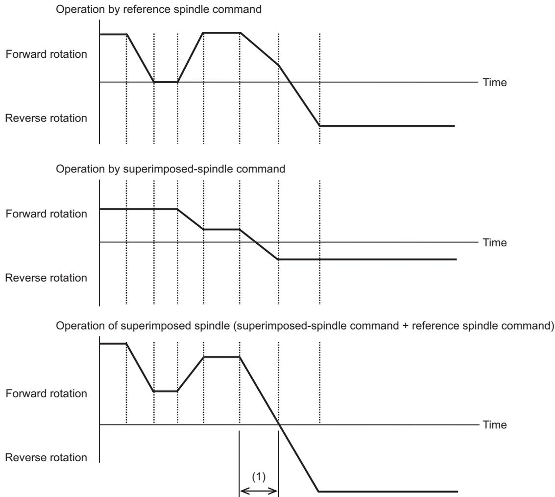
In interval "A", the forward-run deceleration of the reference spindle and the forward- and reverse-run deceleration of the superimposed spindle are carried out frequently; therefore, the acceleration/deceleration time constant is doubled for both the reference and superimposed spindles.
