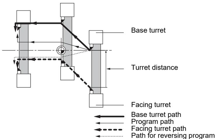
\* This figure does not incorporate the tool length.
