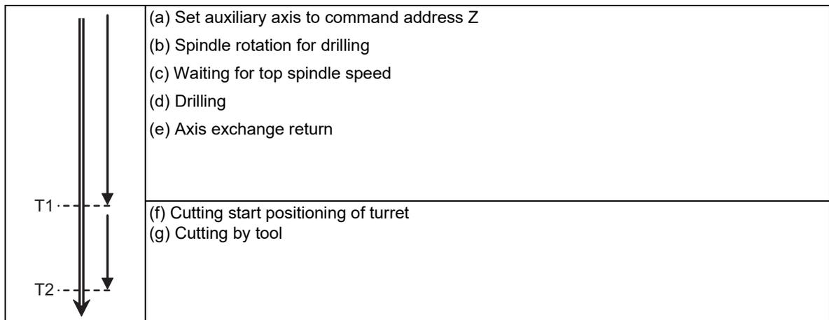
After the back drill machining is complete, cutting by tool is executed.
