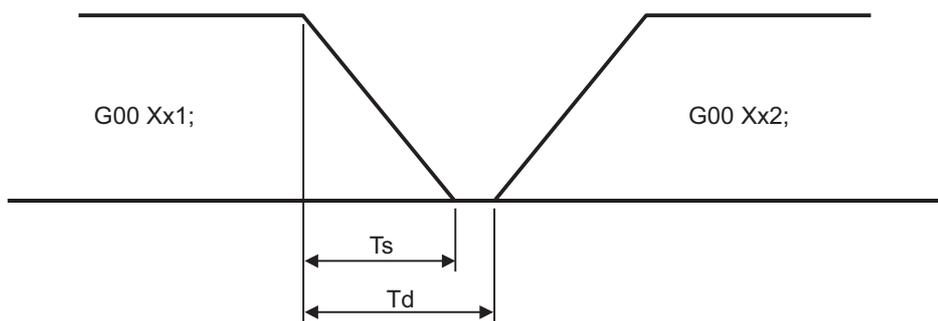
$T_s$ : Acceleration/deceleration time  $T_d$ : Deceleration check time  $T_d = T_s + \alpha$  (0 to 10ms) constant
