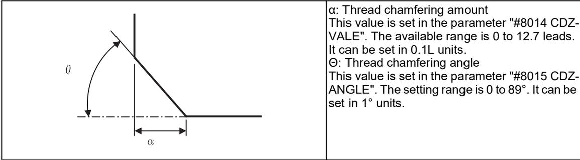
If thread chamfering amount is bigger than a thread lead length, a program error(P192) will occur before starting thread cutting.
