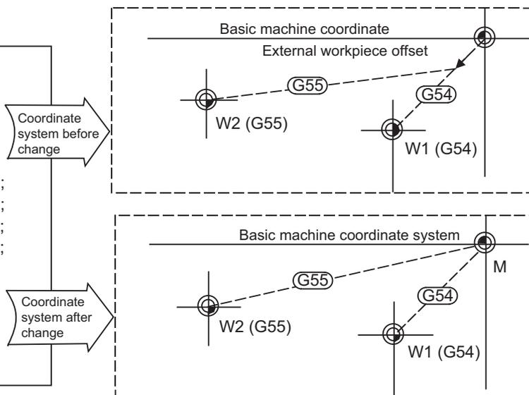
This is an example where the external workpiece compensation values are added to the workpiece coordinate (G54, G55) system compensation values without changing the position of the workpiece coordinate systems.
