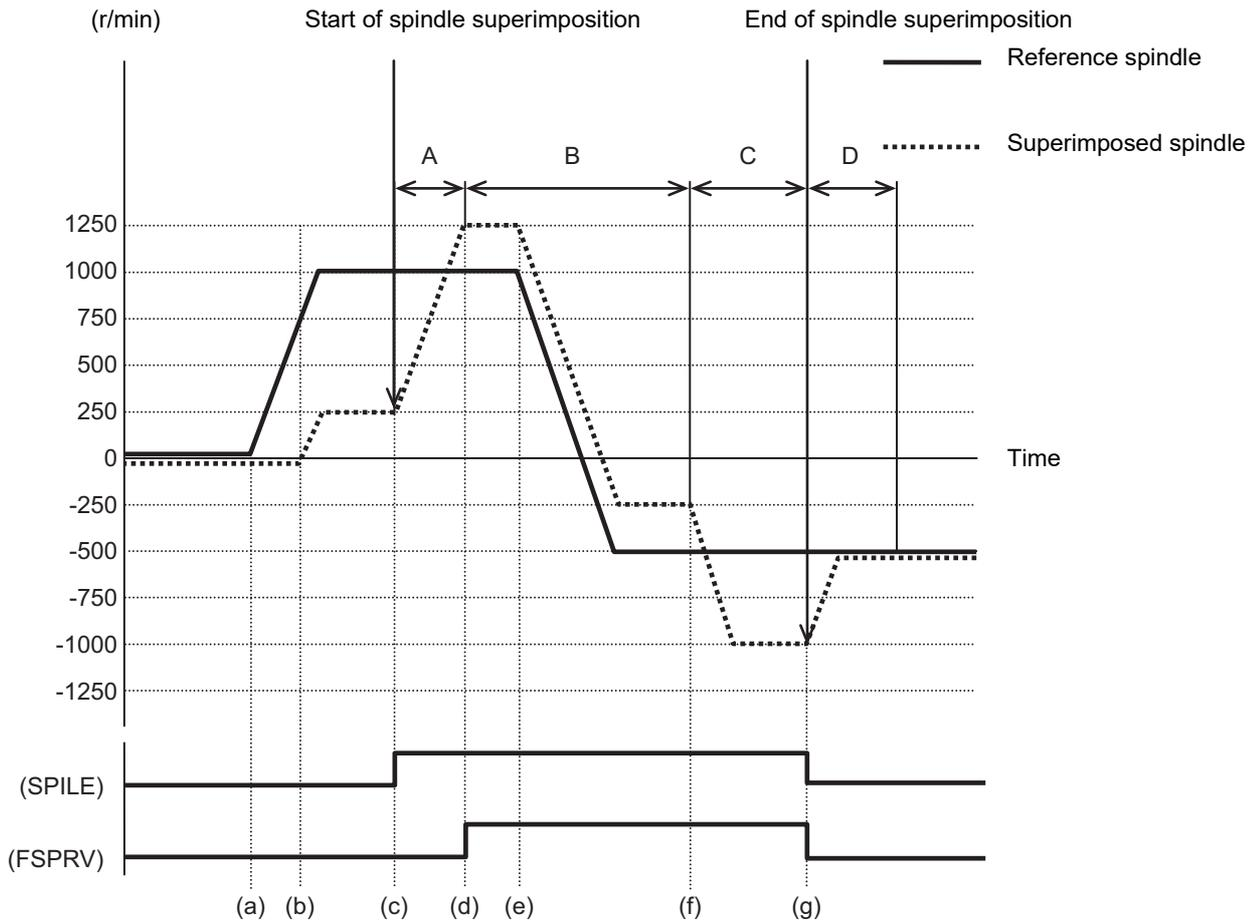
SPILE (Under spindle superimposition control mode): Setting ON outputs the PLC signal indicating that the spindle is in the spindle superimposition control mode.
