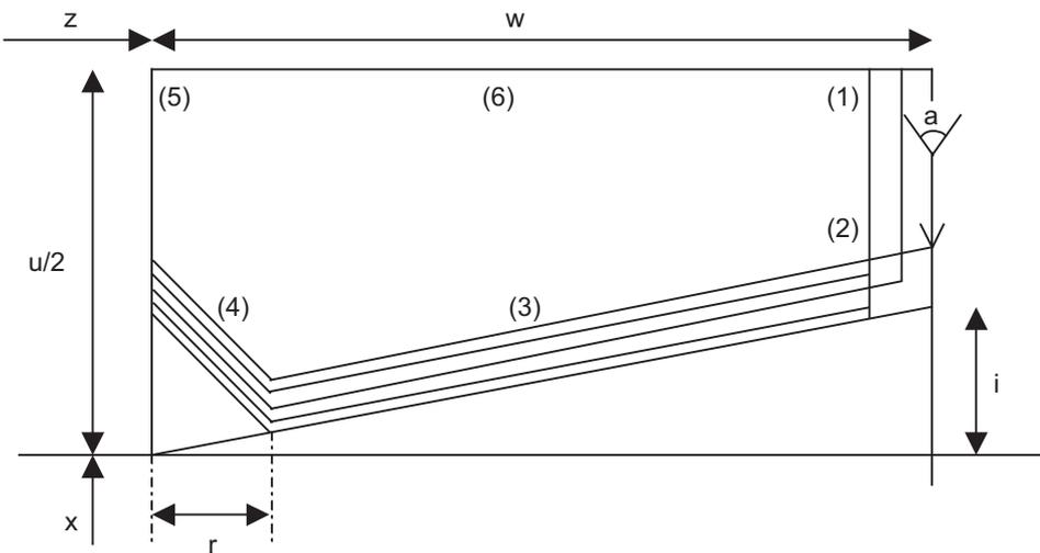
$i$  : Taper height component (radius value) for thread
