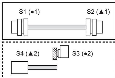
1st set: Spindle synchronization I command [S1(●1) - S2(▲1)]
