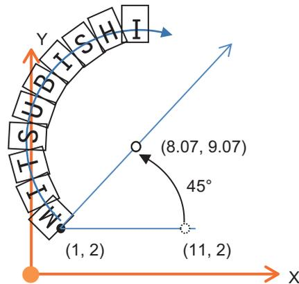
(2) When the text is on an arc
