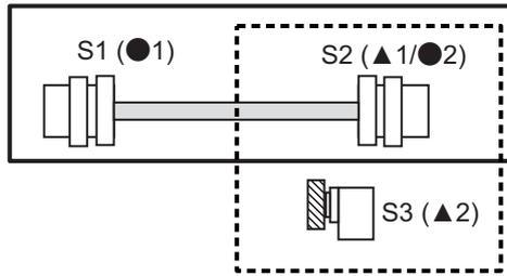
1st set: Spindle synchronization I command [S1(●1) - S2(▲1)]
