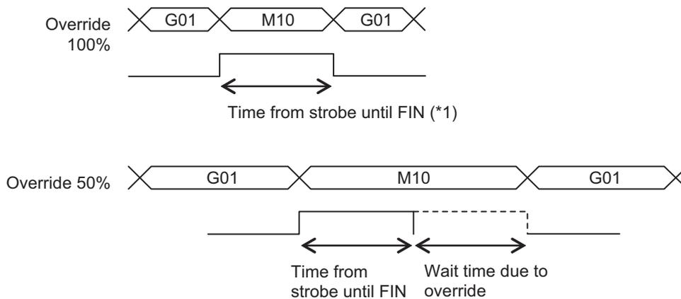
$$\text{Wait time due to override} = \text{Time from strobe until FIN} \times \frac{100}{\text{Override value}} - \text{Time from strobe until FIN}$$
