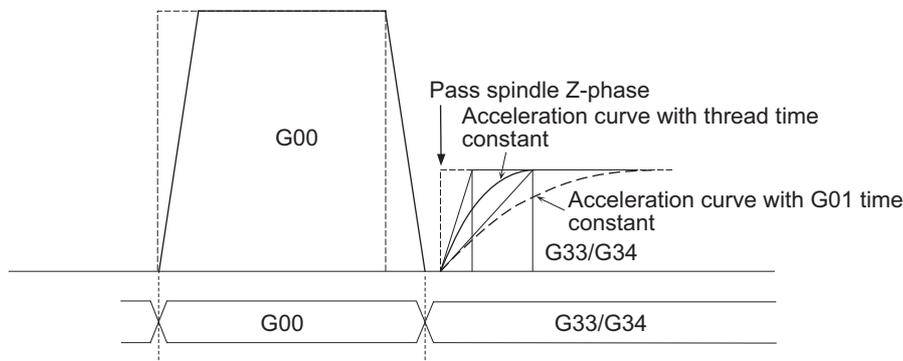
When the thread cutting time constant is valid, thread cutting is clamped at the speed determined in the MTB specifications (parameter "#2619 thr\_clamp").
