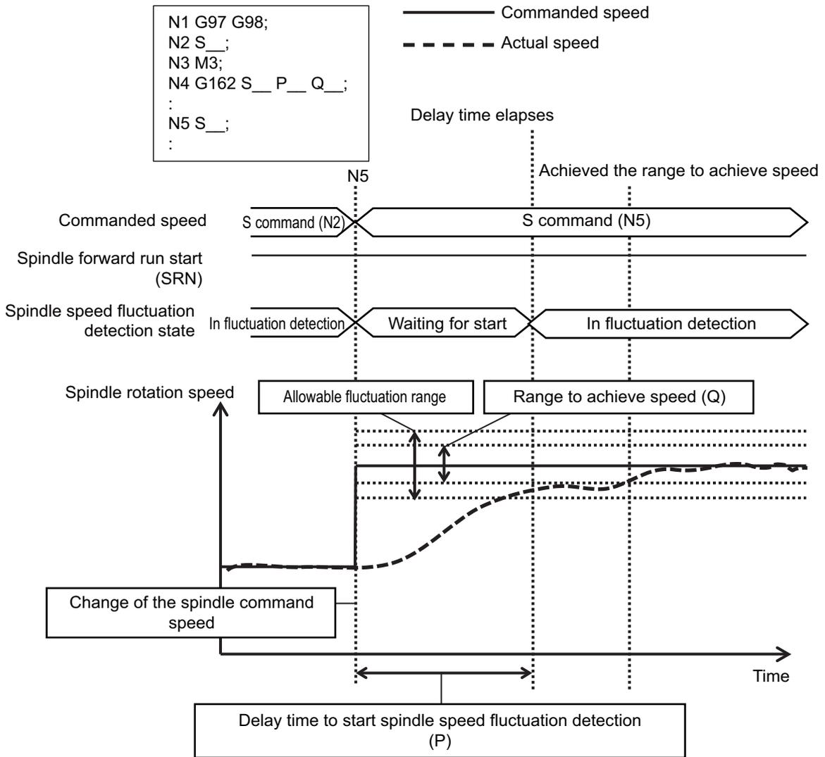
**Temporary cancellation operation of spindle speed fluctuation detection**
