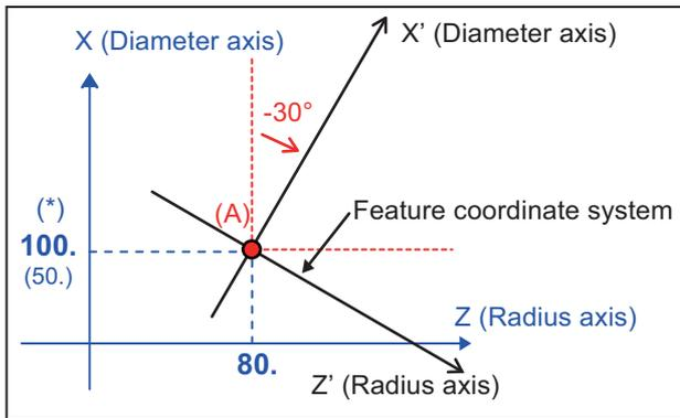
(\*) The contents enclosed in parentheses ( ) indicate the value of the radius value command.
