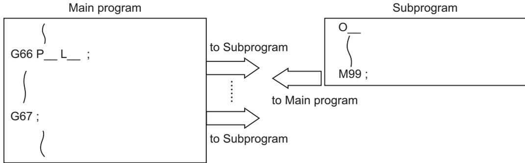
When the block with a movement command is commanded between G66 and G67, the movement command is first executed and then the designated user macro subprogram is executed. A number of user macro subprograms are designated with "L".
