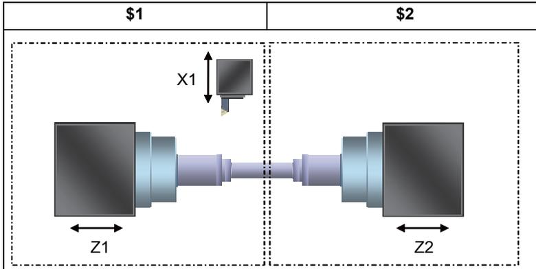
While the synchronization, synchronized axis synchronizes and moves in accordance with the reference axis regardless of conducting automatic operation or manual operation. The movement command cannot be issued to the synchronized axis.
