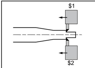
When workpiece that is relatively long and thin is machined on a lathe, deflection may result, making it impossible for the workpiece to be machined with any accuracy.
