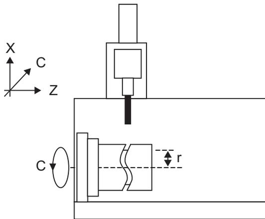
As programming can be carried out to the developed shape of the side of the cylinder, this is effective for machining cylindrical cams, etc. When programmed with the rotary axis and its orthogonal axis, grooves and other shapes can be machined on the side of the cylinder.
