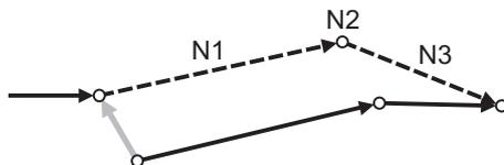
This applies when compensation operation is executed in a block with the move command.
