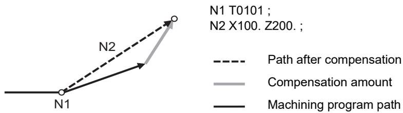
Tool length compensation and tool nose wear compensation are conducted simultaneously.
