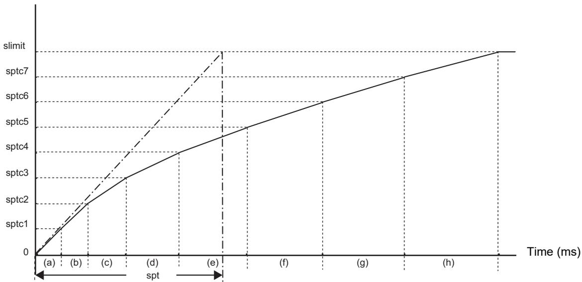
To decrease the number of acceleration/deceleration steps during spindle synchronization, set one of the following for the unnecessary step.
