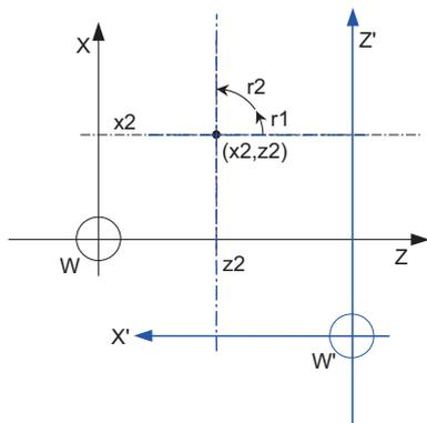
The center coordinate of the rotation switches from (x1, z1) to (x2, z2).
