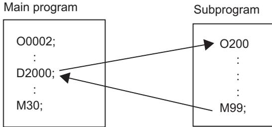
After outputting "2000" to common variable #146, the program No. 200 subprogram is called with the M98 subprogram call type.
