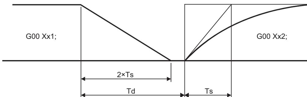
$T_s$ : Acceleration/deceleration time  $T_d$ : Deceleration check time  $T_d = 2 \times T_s + \alpha$  (0 to 10ms) constant
