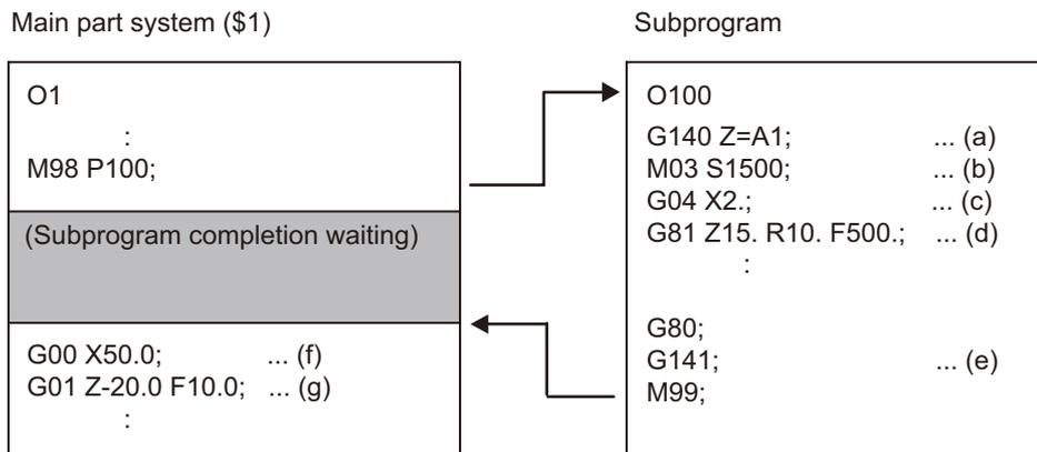
G140: Arbitrary axis exchange command (Lathe system only)
