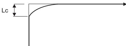
To eliminate corner roundness, set the value as small as possible to servo parameter "#2224 sv024" and perform an in-position check or assign the dwell command (G04) between blocks. (The parameter setting depends on the MTB specifications.)
