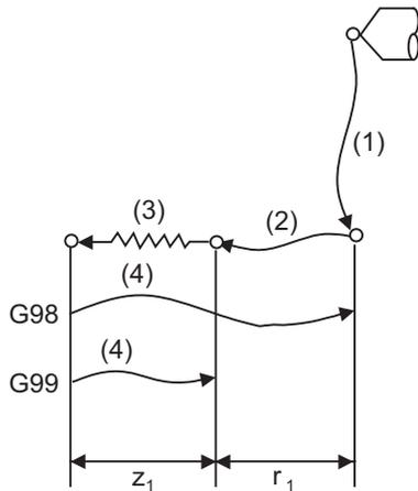
The operation stops at after the (1), (2) and (4) commands during single block operation.
