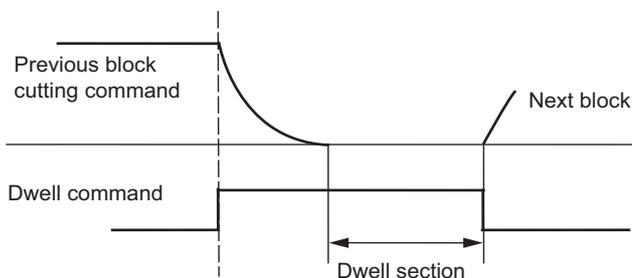
When the number of revolutions for dwell is set to 100 (rev) and the spindle rotation speed is set to 1000 (r/min), the machine waits for 6 seconds during the dwell interval.
