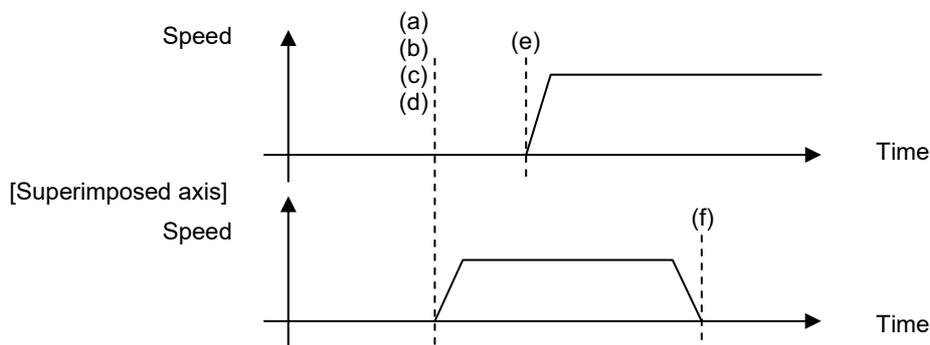
A movement command can be issued to the reference axis while the superimposed axis is moving to the arbitrary axis superimposition end position.
