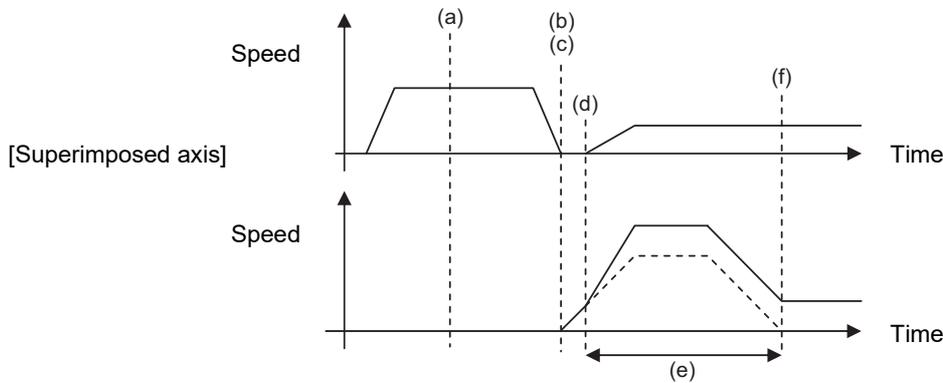
The broken line portion indicates the movement amount to the start position of arbitrary axis superimposition.
