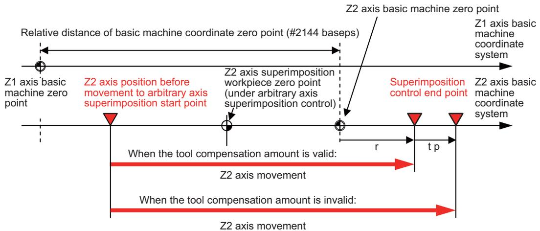
The position is shifted by the amount of the position commanded by R from workpiece coordinate zero point (+ superimposed axis tool compensation amount "tp").
