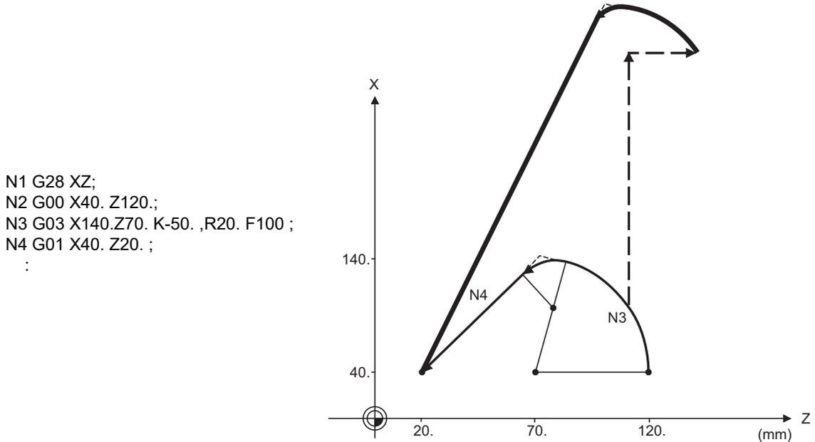
With an incremental command and manual absolute switch OFF
