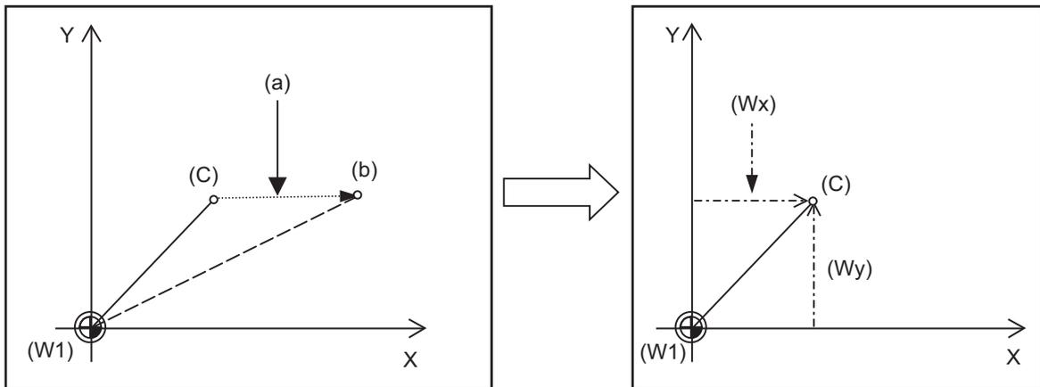
(a) Movement amount during machine lock (b) Workpiece coordinate system coordinate value
