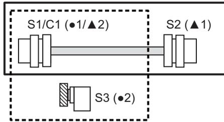
1st set: Spindle synchronization C axis command [S1/C1(●1) - S2(▲1)]
