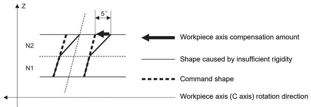
**Feedforward control during tool spindle synchronization II (hobbing) mode**
