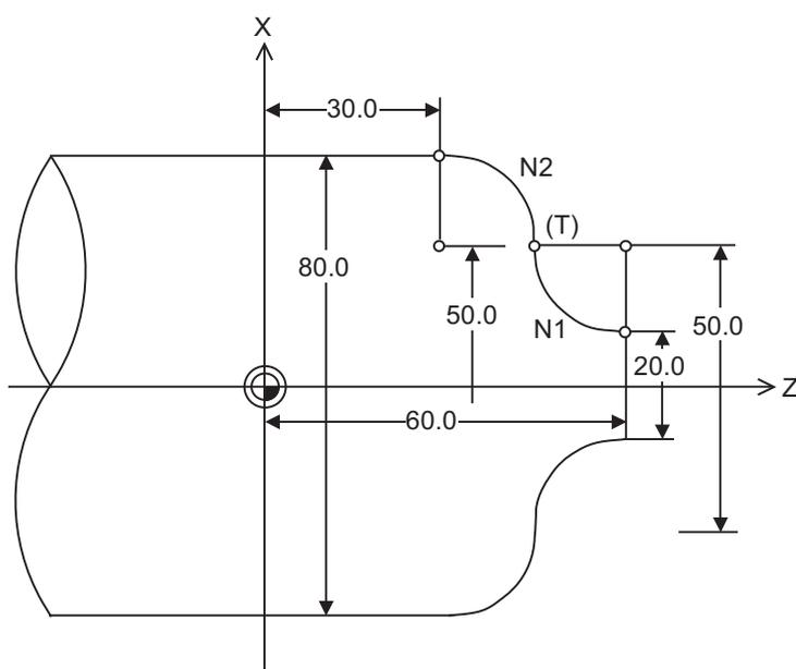
(T) Contact point (calculated automatically)
