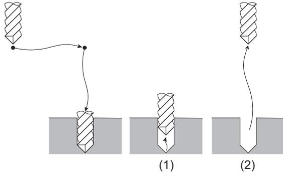
The drill moves up at high-speed ((1) in the figure) and returns to the initial point or R point in rapid traverse ((2) in the figure).
