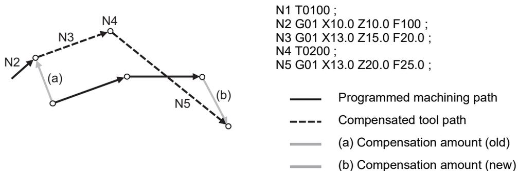
In this example, the tool length is compensated with the tool No. and compensation is performed in the block with the movement command.
