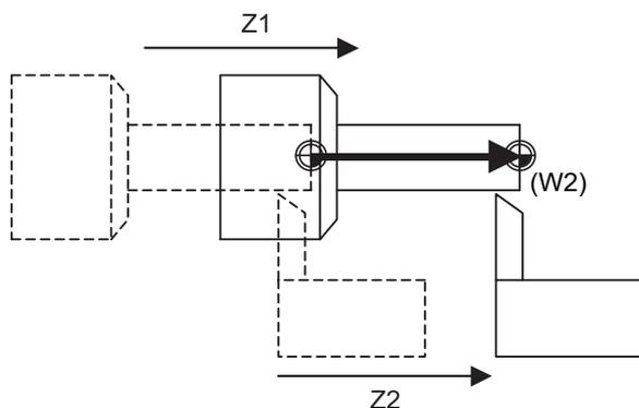
**[Axis movement during the superimposition control]****(1) When commanding movement only to the reference axis**
