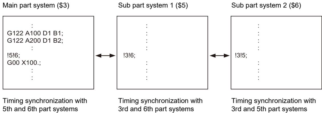
(Example 2) Timing synchronization by designating a sub part system identification No.
