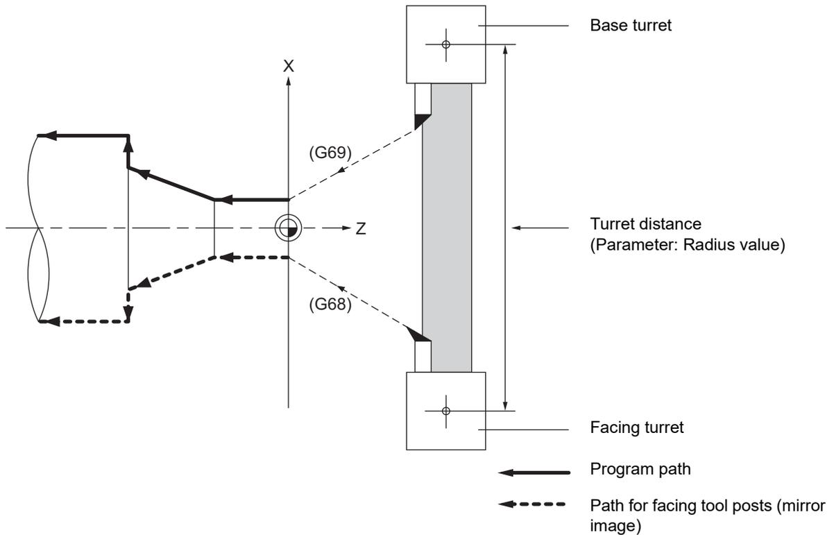
The axis with the mirror image for facing tool posts valid depends on the MTB specifications (parameter "#1273 ext09/bit4").
