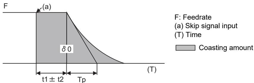
The relationship between the coasting amount and speed when " $T_p$ " is 30 ms and " $t_1$ " is 5 ms is shown in the following figure.
