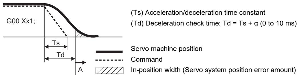
(2) In-position check with programmable command (",I" address command)
