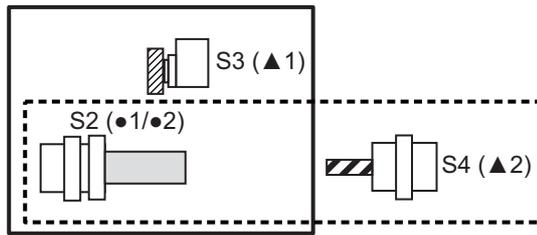
1st set: Tool spindle synchronization IA command [S2(●1) - S3(▲1)]
