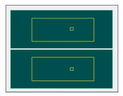
The white-framed display range in the upper and lower areas simultaneously move to the left/right when the  $[\leftarrow]$ ,  $[\rightarrow]$  keys are pressed.
