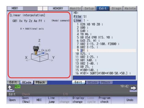
G code displayed in the G code guidance area is refreshed as the cursor moves across the program edit screen. When you change the available edit area during simultaneous program edit (3 programs), G code guidance is also refreshed.
