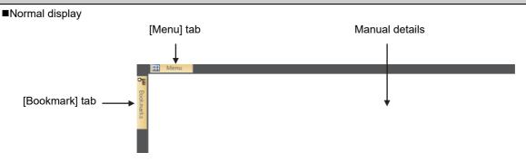
Touch the [Menu] tab to switch to the ribbon display. The ribbon displays the operation buttons such as page switching, enlarging/reducing, rotation and search.
