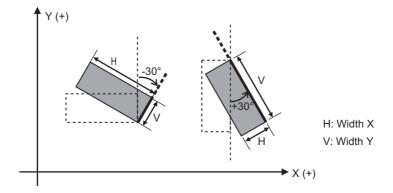
"H: Width X" and "V: Width Y" are the same on the YZ plane and the ZX plane.
