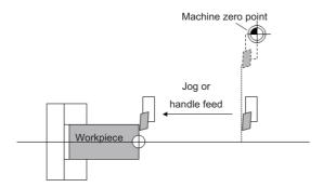
(5) Input the name of the axis to be measured, and the measurement value from the workpiece to the tool nose. Z0.
