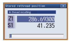
(2) Press the menu [Thrdrecut OFF] in the state "In thread recutting".
