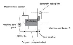
(6) Enter the name of axis to be measured, and the measurement value (radius) of workpiece.
