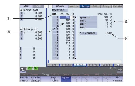
Manual numerical value command can be executed when manual numerical value command window is displayed by inputting an address key such as MST, etc.
