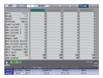
The axis name set in the base axis specification parameter "#1022 axname2" appears at the axis name.
