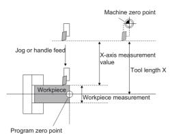
(9) Enter the name of axis to be measured, and the measurement value (diameter) of workpiece.
