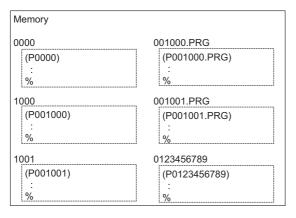
(3) Comparison is carried out. (As the serial/batch files are compared with the leading zeros deleted, changing file names is not required.)
