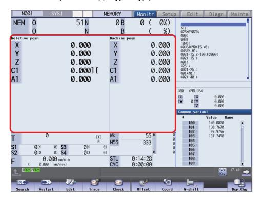
(1) The maximum number of axes that can be displayed is 8 axes. Press the menu [Next axis] to switch display to display the subsequent axes.
