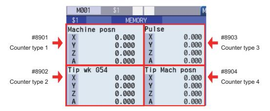
■[Quad counter] (4-part system simultaneous display)
