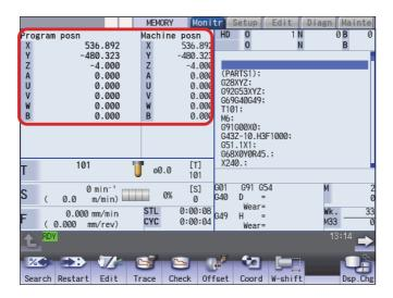
(1) The maximum number of axes that can be displayed is 10 axes. Press the menu [Next axis] to switch display to display the subsequent axes.
