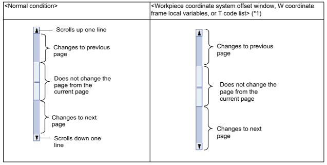
(\*1) For the workpiece coordinate system offset window and local variable window on the monitor screen as well as coordinate system offset frame and T code list window on the setup screen, the page changes to the previous page when [▲] of scroll bar is touched, and the page changes to the next page when [▼] of scroll bar is touched. (It is not possible to scroll in a line unit.)
