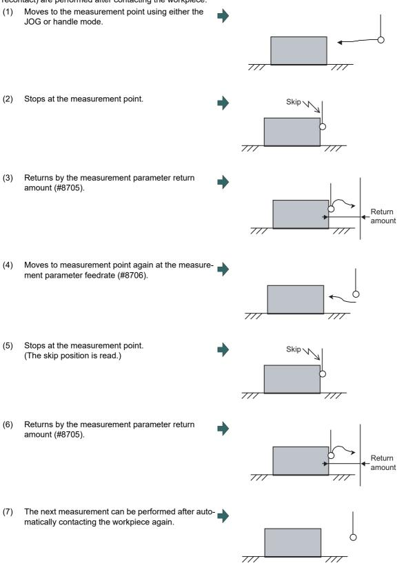
The return speed for (3) and (6) is 40 times the measurement parameter feedrate (#8706). However, if the return speed is faster than rapid traverse rate (override 100%), the rapid traverse rate will become the return speed.
