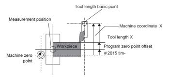
(9) Enter the name of axis to be measured, and the measurement value (diameter) of workpiece.
