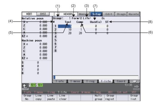
The number of groups to be displayed on a single screen depends on the setting of the parameter "#1107 Tlifsc". (This depends on the MTB specifications.)
