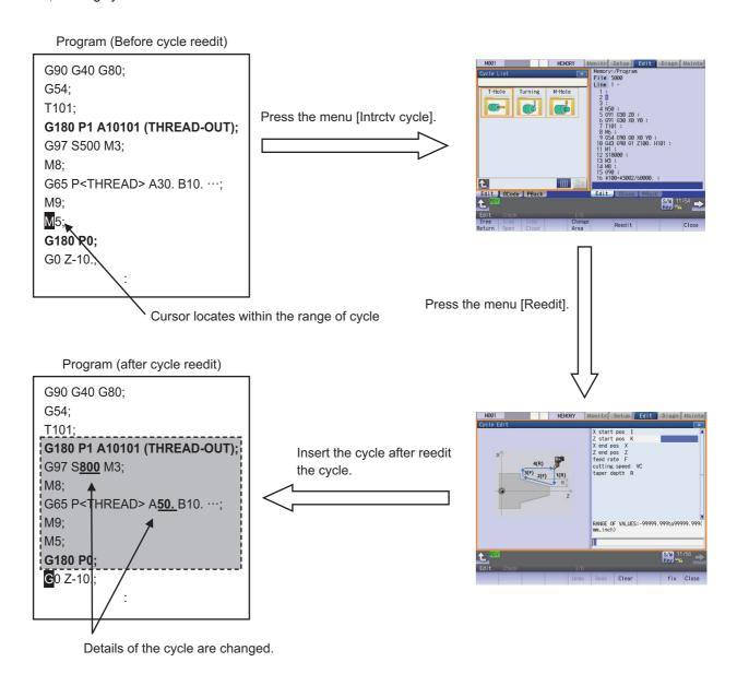
After reediting the cycle, the screen returns to the cycle list window in the state that the reedit results were reflected to the cycle. The inserted cycle is highlighted in the editing area of the program, and the cursor moves to the head of the next line of the cycle. Then, the program is saved.
