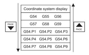
The optional specification is required for the G54.P1 - P300 workpiece coordinate system offset display.
