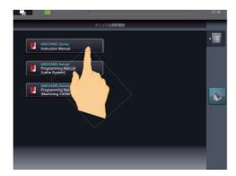
When you operate with keys, move the cursor with  $[\uparrow]$ ,  $[\downarrow]$ ,  $[\leftarrow]$  or  $[\rightarrow]$  key and determine with the [IN-PUT] key to display the selected manual.
