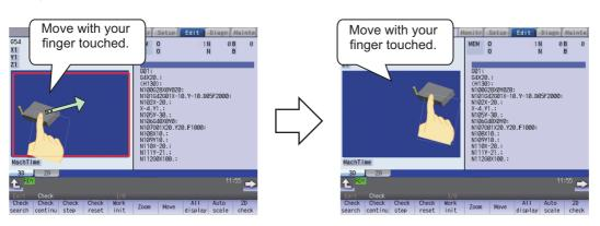
You can rotate a machining shape using a two-finger drag operation (put two of your finger tips on the screen and move them vertically/horizontally without losing contact).
