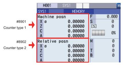
■[Quad counter](2-part/3-part system simultaneous display)
