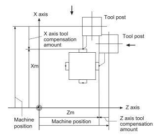
When the tool touches the touch probe while measurement switch is ON, the calculation result is set in the tool data of the compensation No. specified with "Tool No. (Tool length measurement 2)" (PLC device), and the wear data of the compensation No. set in "Wear compensation No. (Tool presetter)" (PLC device) is cleared.
