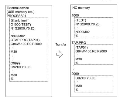
When the external device is serial, the top line is %.
