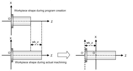
Set "wk\_z" in the workpiece coordinate system shift value.
