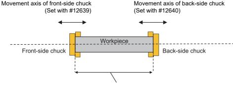
When the workpiece is passed, the distance between the front-side chuck and back-side chuck is regarded as the material length of the workpiece being machined.
