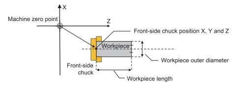
For the chuck position, the setting by the MTB is required.
