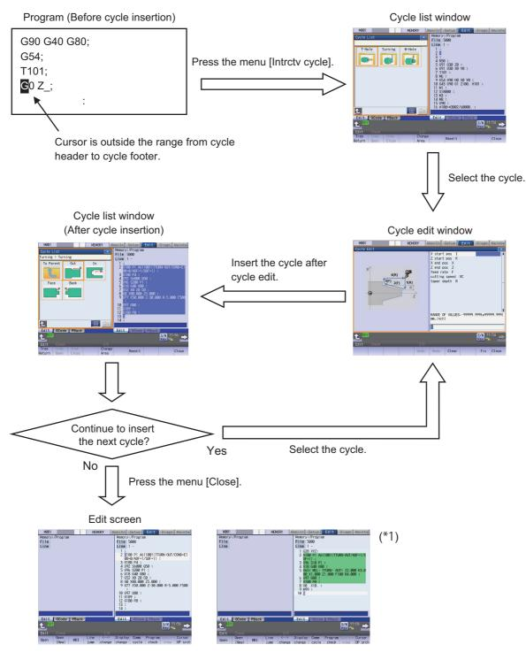
After the cycle insertion, the screen returns to the cycle list window in the cycle inserted state. The inserted cycle is highlighted in the editing area of the program, and the cursor moves to the head of the next line of the cycle. Then, the program is saved
