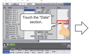
The parameter screen is being displayed (the cursor position is at #1026).
