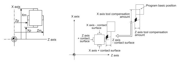
When tool presetter operation is performed at the main spindle side:
