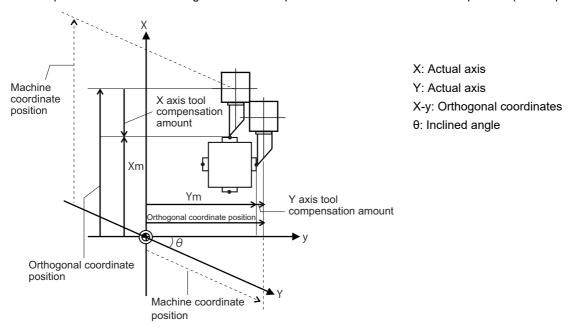
Two inclined axes move at the same time on orthogonal coordinates (X-y). The message "TLM axis is illegal" appears.
