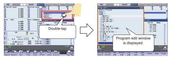
(Example) Displaying the window by double-tapping the selective display area
