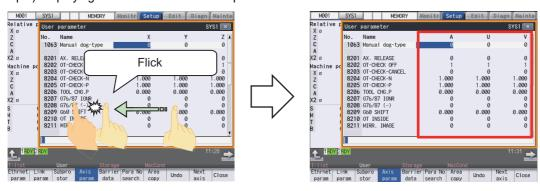
The axis parameters (X, Y and Z axes) are displayed.
