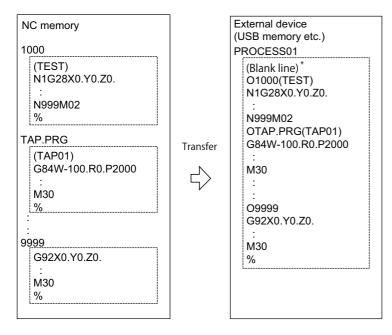
When the external device is serial, the top line is %.
