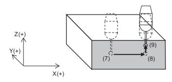
On each measurement point, after contacting the touch probe to the workpiece with skip operation, separate the touch probe from the workpiece once and then measure the coordinate on the workpiece with decelerated skip operation.
