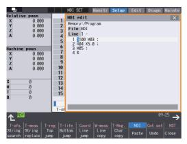
Program example (to rotate the spindle at 100 r/min for 5 seconds)
