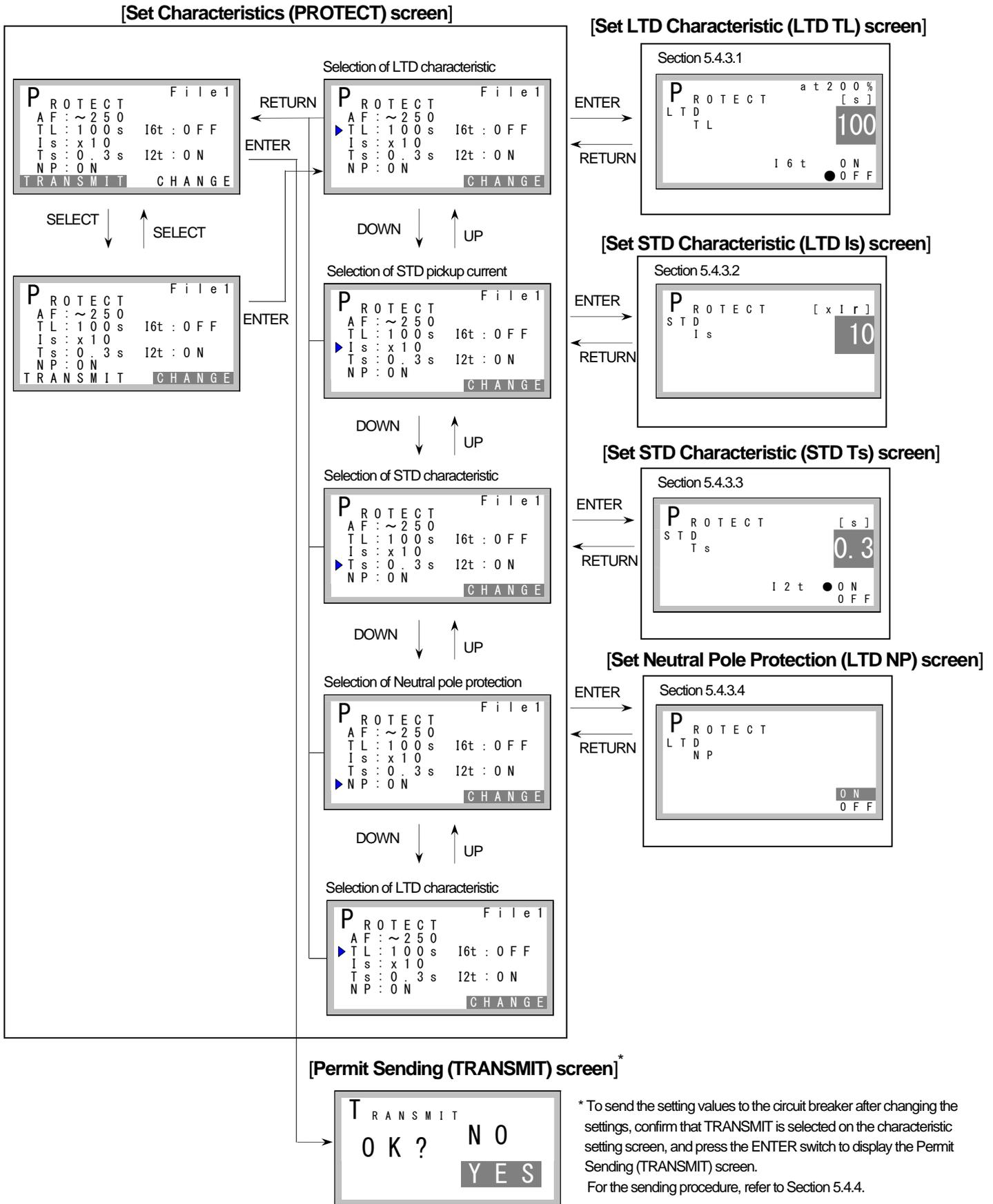
\* To send the setting values to the circuit breaker after changing the settings, confirm that TRANSMIT is selected on the characteristic setting screen, and press the ENTER switch to display the Permit Sending (TRANSMIT) screen. For the sending procedure, refer to Section 5.4.4.
