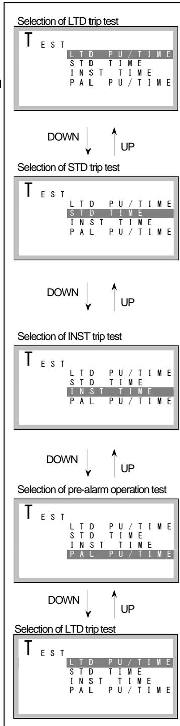
[LTD Trip Test (LTD PU/TIME) screen]
