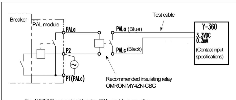
Fig. 4 W&WS series circuit breaker PAL module connection
