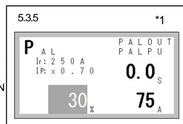
\*1 For a WS-V series circuit breaker or MDU breaker, confirm that Ir, Ii, current, OVER, and PALPU are displayed on the test screen.
