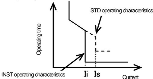
(2) When the STD pickup current ( $I_s$ ) is equal to the INST pickup current ( $I_i$ )
