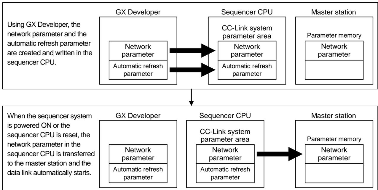
Note : The parameter setting by GX Developer has the following characteristics.
