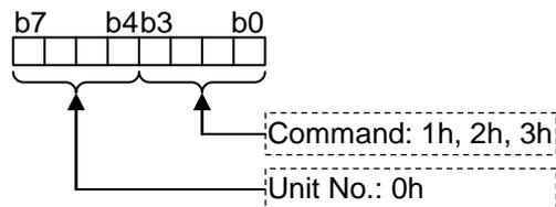
For example, when the unit number is 0h and the command is 1h, the unit number is indicated by "01h".
