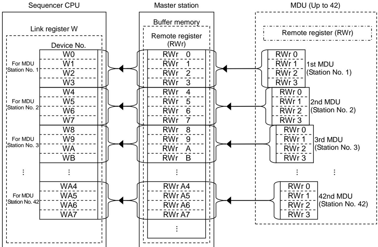
Table 5.2.4.3 Relation of the station number for the remote register (RWr) and the link register W in the sequencer CPU
