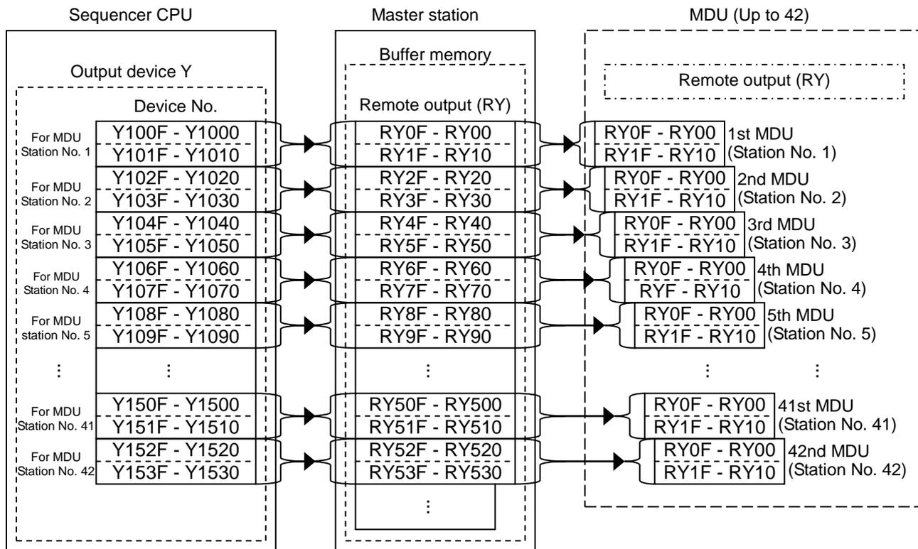
Table 5.2.4.6 Relation of the station number for the remote output (RY) and the output device Y in the sequencer CPU
