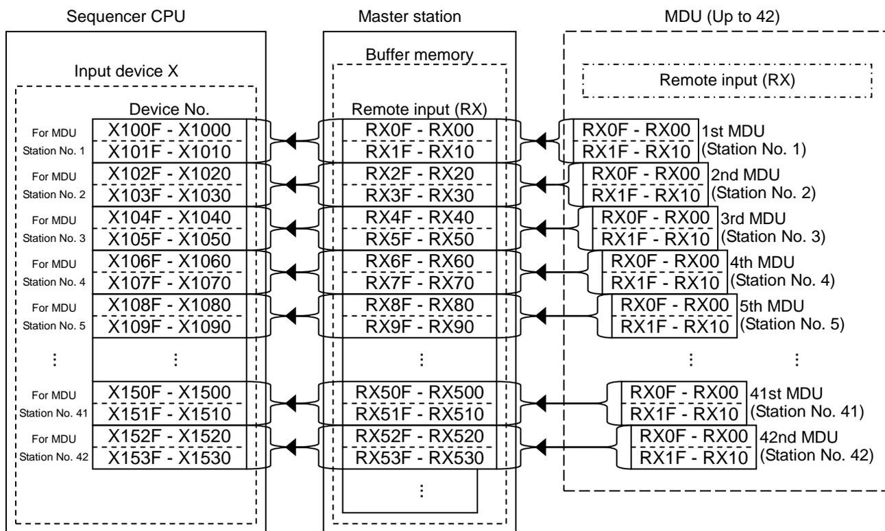
Table 5.2.4.5 Relation of the station number for the remote input (RX) and the input device X in the sequencer CPU
