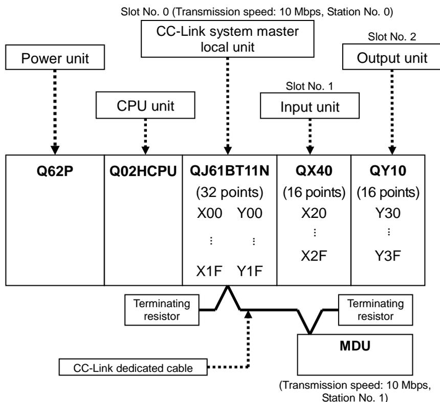
In the sample program, the first input/output number is 00h (or 0000) because the CC-Link master unit (QJ61BT11N) is equipped to the slot No. 0 of the base unit as shown in the configuration above.
