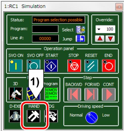
1) Click the "HAND" button in the operation panel to display the Hand Operation panel.
