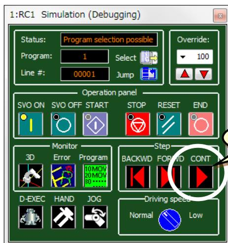
Pressing the "CONT" button on the operation panel continuously executes the program for one cycle.
