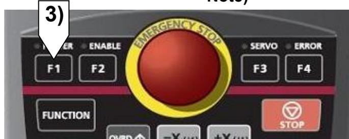
Note) "Electric" appears only when using the electric operated hand. If the function key ([F3] key in this case) corresponding to this is pressed, the <Electric Operated Hand Operation> screen will open.
