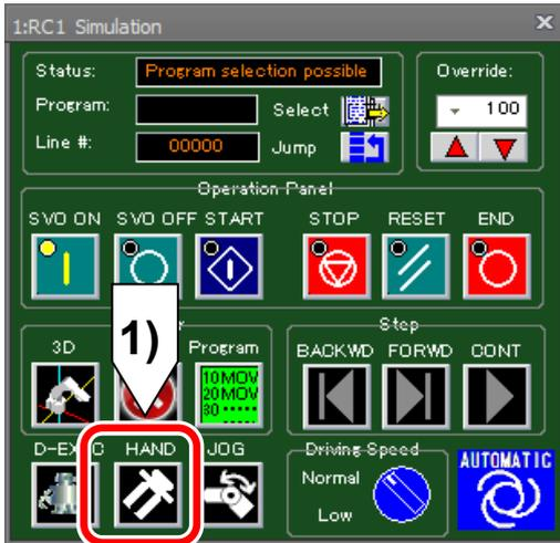
1) Click the "HAND" button in the operation panel to display the Hand Operation panel.
