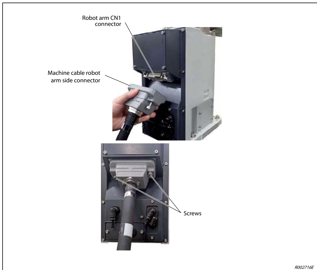
Fig. 4-6: Connecting the machine cable on the robot arm side
