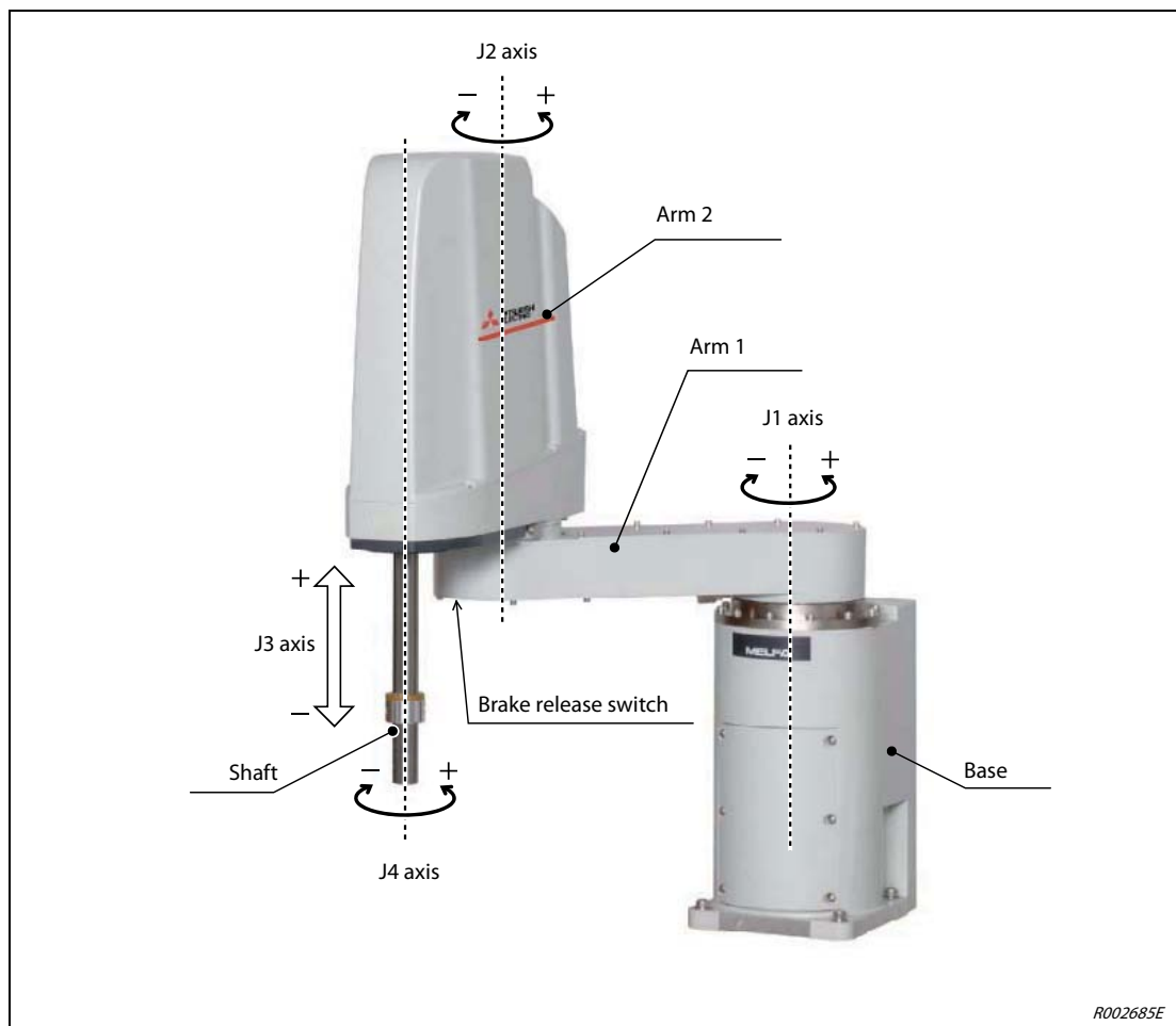
Fig. 2-8: Components of the robot arm RH-3FRH/6FRH/12FRH/20FRH
