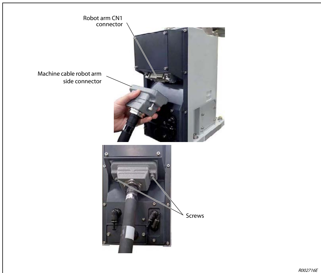
Fig. 4-4: Connecting the machine cable on the robot arm side
