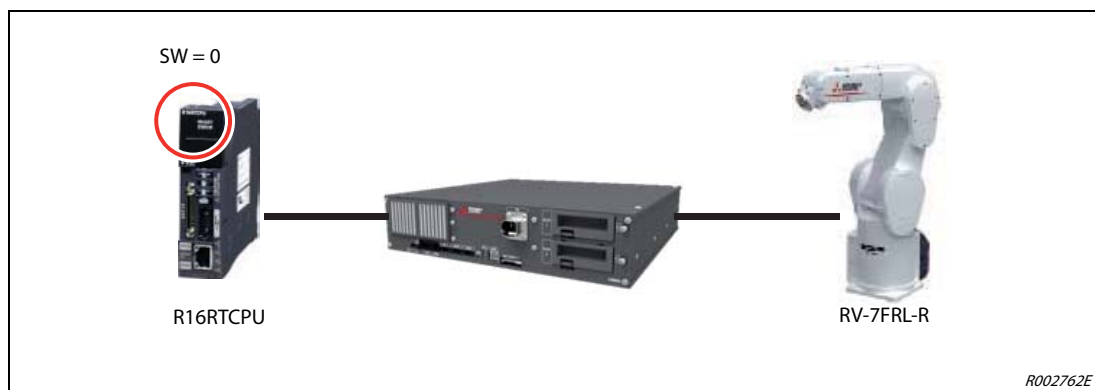
Fig. 5-7: Connect the robot to the controller CR800-R
