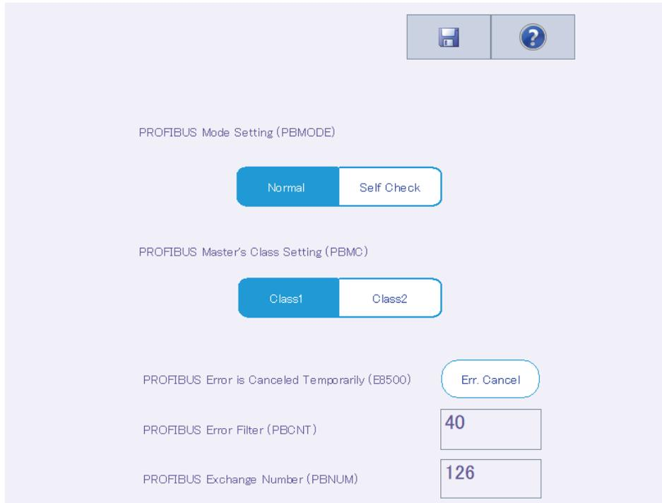
Tapping [Err. Cancel] will reset PROFIBUS interface card errors, and prevent the same error from occurring. This function is enabled while the controller is powered on. When the power is turned off, the error may occur again.
