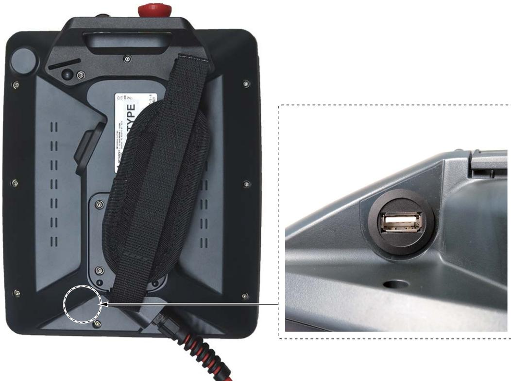
Once the USB memory is connected correctly, it will be detected by the operating system and displayed as a device.
