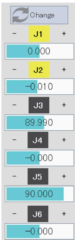
3. Rotating the wheel will move the selected axis. (Rotating the wheel clockwise will move the axis in the positive direction and rotating it counterclockwise will move the axis in the negative direction.)
