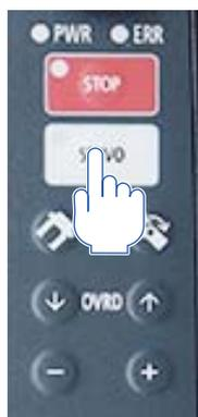
5. The robot moves while the [+] or [-] button (sheet key) corresponding to the displayed jog operation guide is pressed.
