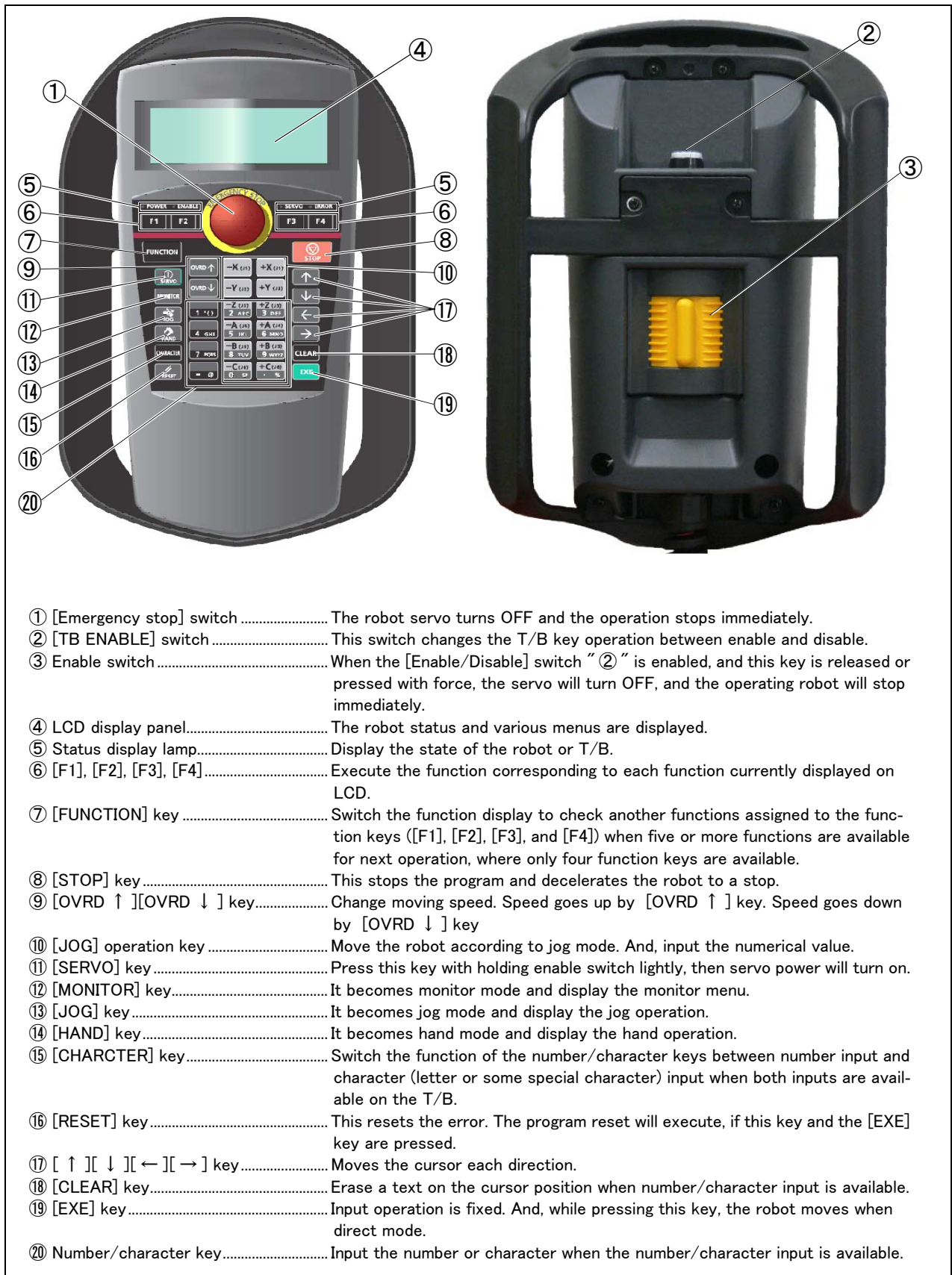
Fig.3-24 : Teaching pendant key layout and main functions
