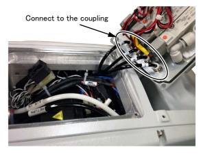
5) Installs the solenoid valve set on the forearm upside. (standard/internal wiring and piping specification common) Installs the solenoid valve set instead of the No.2 arm cover U removed above.
