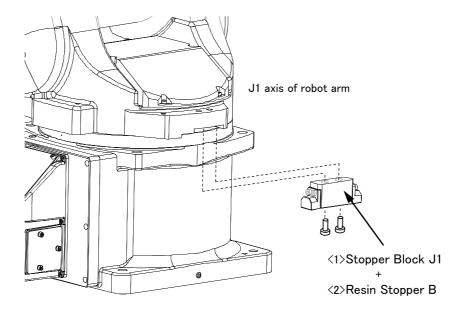
3) Because to install the Mechanical Stopper screw, once move the J1 axis to the position of 0 degree. Turn on the power supply and move the J1 axis by jog operation.
