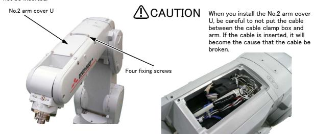
The condition of storing the cable inside the No.2 arm cover U
