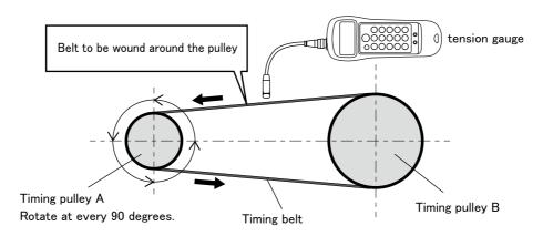
Fig.5-8: Timing belt tension measurement
