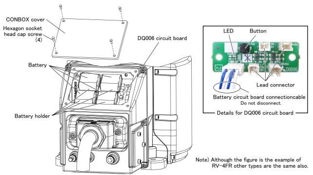
Fig.5-31: Replacing the battery (RV-4FR/7FR/13FR series)
