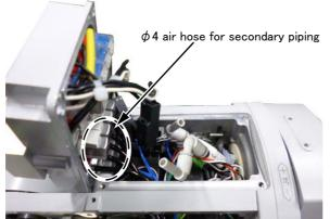
$\langle$ Enlarged view of the  $\phi$ 4 air hose connection area $\rangle$
