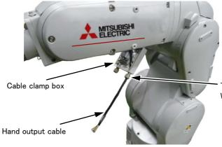
Threaded cap of the cable clamp (Tip) With the plug
