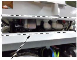
Visually check that the cables and air hoses are not pinched, and the air hoses are not bent.
