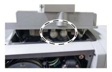
As shown in the above figure, adjust the direction of elbow couplings connected to AIR IN (white) and RETURN (black) as cross the solenoid valve to improve workability.
