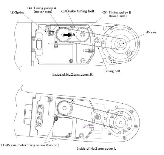
Fig.5-15: Inspection and replacement of J5 axis brake timing belt (RV-2FR series)
