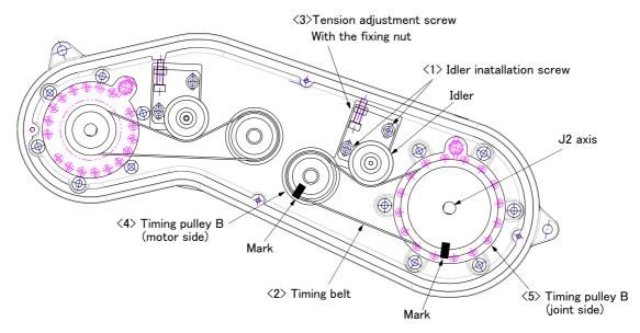
Fig.5-11: Inspection and replacement of J2 axis timing belt (RV-2FR series)
