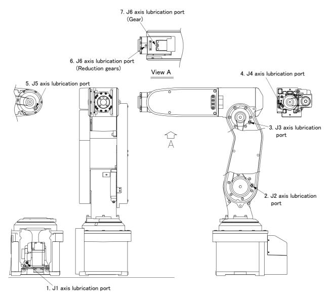
Fig.5-27: Lubrication positions (RV-2FR series)
