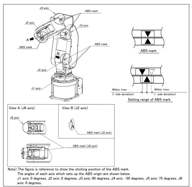
Fig.5-36: ABS mark attachment positions (RV-2FR series)
