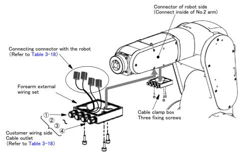
Fig.3-8: Installing the Forearm external wiring set
