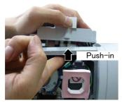
As shown in the above figure, push in the elbow couplings from the No.2 arm cover L side to improve workability.
