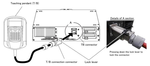
Fig. 2-13: Installing the T/B
