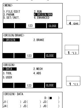
Press the [4] key on the menu screen, and display the ORIGIN/BRAKE screen.
