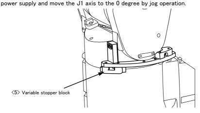
4) Install the Mechanical stopper screw A or B. Install the necessary screw with referring to Table 3-8 and Table 3-9.
