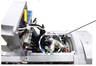
Attach the elbow couplings to the AIR IN (white) and RETURN (black) air hoses. Two elbow couplings are made to connect with the air hose of RETURN (black) to a
