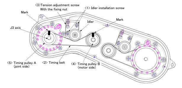
Fig.5-12: Inspection and replacement of J3 axis timing belt (RV-2FR series)
