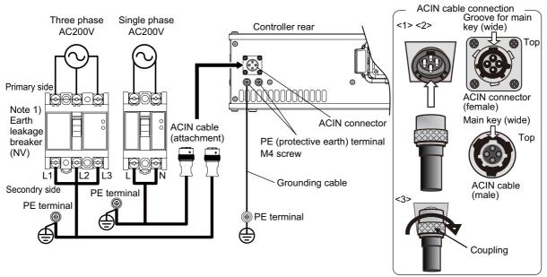
Note 1) Always use the terminal cover for the earth leakage breaker.
