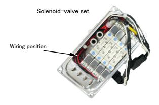
b) Connects the hand output cable inside the forearm (GR1 and GR2) to the connectors of the solenoidvalve set.
