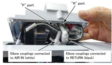
Note) The lead wire should be wired inside elbow couplings to prevent inserting the cable as shown in a figure
