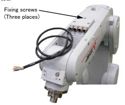
\* The figure is the example to which the J4 axis was moved to upside down position by jog operation. (For 6-axis type robot)
