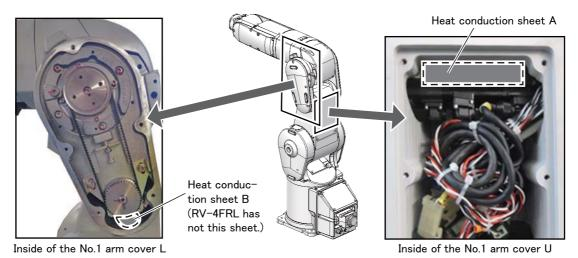
Fig.5-20: Heat conduction sheet position
