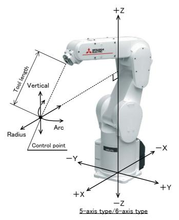
\* The current position is set as the arc centering on the Z axis, and the axis moves along that arc, expands and contracts in the radius direction, and moves vertically. At this time, the flange surface posture is maintained. Also, while maintaining the flange surface position, the flange surface posture changes.
