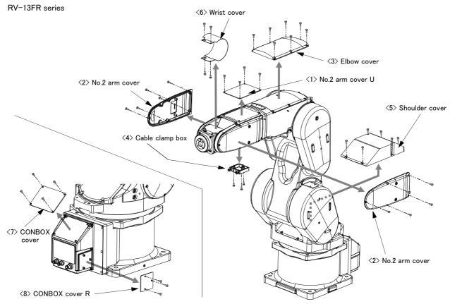
Fig.5-6: Installing/removing the cover (RV-13FR series)
