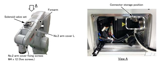
6) Connect the tool prepared by the customer with solenoid valve port A and B. (standard/internal wiring and piping specification common)
