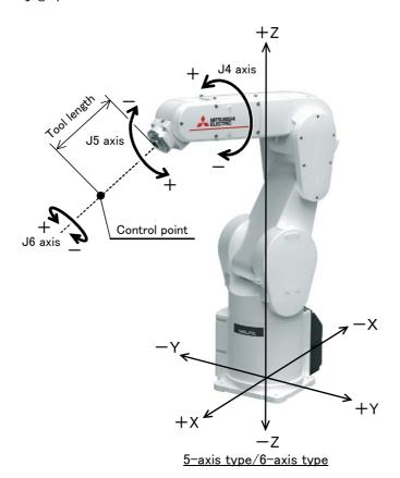
\* The axis moves straight along the base coordinate system. At this time, the flange surface posture is not maintained. Also, the flange surface posture changes. The flange surface position does not change at this time. It is effective to change the posture of the wrist, with the position maintained. The 5-axis type robot has no J4 axis.
