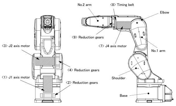
Fig 5-3: Outline structure of robot arm (RV-13FR series)
