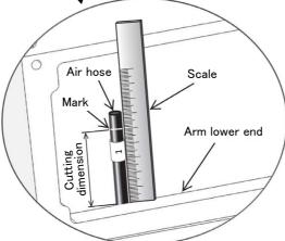
5) Cut the  $\phi$ 6 primary piping air hoses. (standard/internal wiring and piping specification common) To facilitate connection to the solenoid valve, measure the length of  $\phi$  6 primary piping air hoses (AIR IN and RETURN) from the end of rubber sheet at the base of the air hoses before cutting
