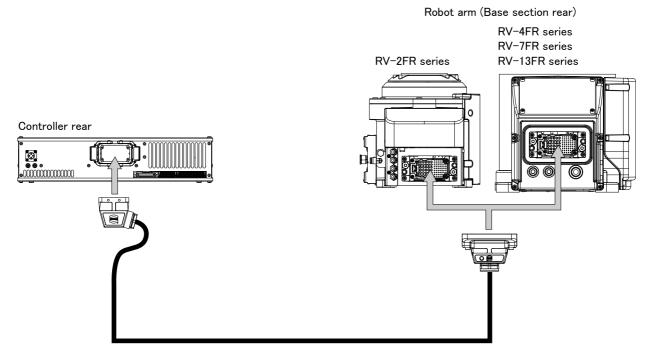
Fig.2-10: Connecting the machine cables
