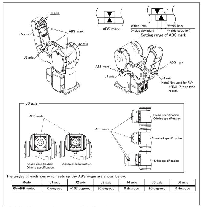
Fig.5-37: ABS mark attachment positions (RV-4FR series)
