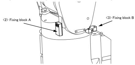
2) Install the Stopper plate <1>. Install by using each two screws (RV-4FR: screw <8>, RV-7FR: screw <7>), adjusting the combination position of the Fixing block A <2> and the Fixing block B <3>. Finally fix  $\langle 1 \rangle, \langle 2 \rangle, \langle 3 \rangle$  securely.
