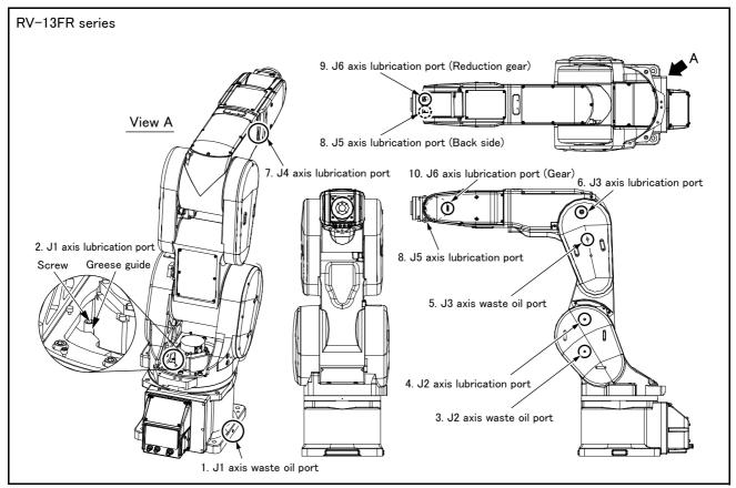
Fig.5-29: Lubrication positions (RV-13FR series)
