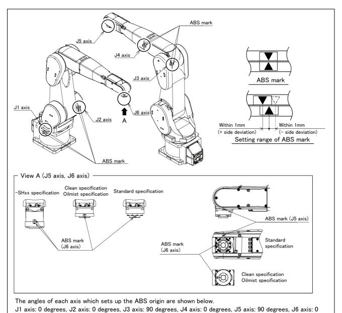
Fig.5-39 : ABS mark attachment positions (RV-13FR series)
