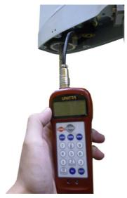
Fig.5-7: Tension adjustment method of timing belt
