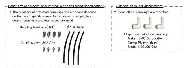
1) Removes the plug on the solenoid valve and installs the coupling. (only internal wiring and piping specification) Remove the plug of the position to use as shown in the figure.
