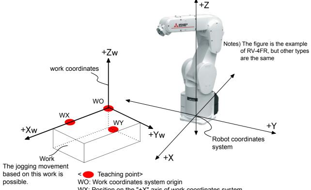
WX: Position on the "+X" axis of work coordinates system. WY: Position at the side of "+Y" axis on the X-Y plane of work coordinates system.
