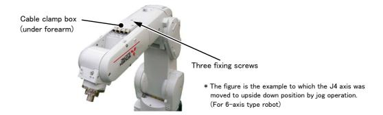
3) Feed the hand output cable through to the cable clamp box side from No.2 arm cover U side inside the arm. When the cable inside the No.2 arm cover U is pulled out, it will become easy. Feed the hand output cable through between the motors. (ellipse position of following figure)
