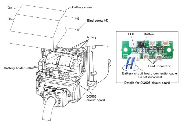
Fig.5-30: Replacing the battery (RV-2FR series)
