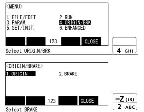
1) Press the [4] key on the menu screen, and display the Origin/Brake selection screen.
