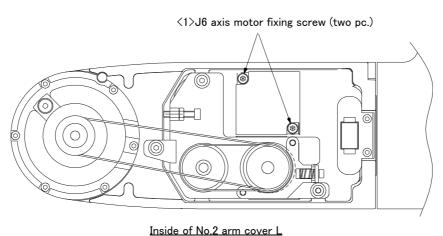
Fig.5-17: Inspection and replacement of J6 axis brake timing belt (RV-2FRB/2FRLB)
