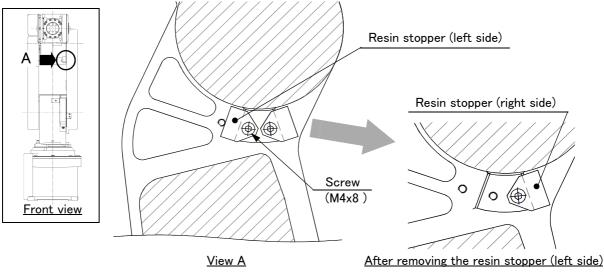
2) Install the stopper of the operating range change (option). Tighten screws firmly to fix the stopper. (Tightening torque: 4.6 Nm)
