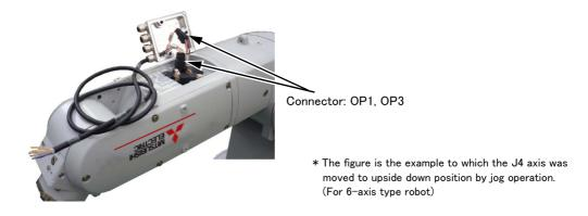
4) Fixes the cable clamp box securely by the fixing screws as before. Installs carefully so that the cable may not be inserted.
