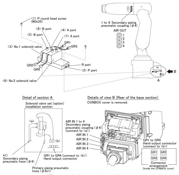
\*1) Please prepare by the customer the pneumatic hose to connect the solenoid valve set.
