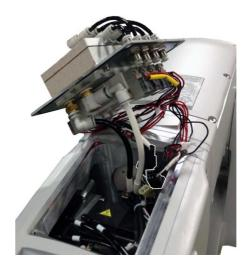
c) Connect the piping inside the wrist. (only internal wiring and piping specification) Cuts the air hose inside of the wrist to suitable length, and connect to the coupling on the back side of solenoid valve set. The number indicated on the air hoses inside of the wrist is same as the air hoses pulled out of the mechanical interface, so make it the reference at the piping to the tool. Table 3-14 shows the relation between hand condition and port number.
