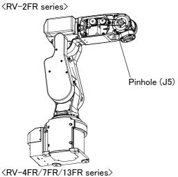
8) Move the J5 axis slowly with both hands to the following position and align the pinhole of the No.2 arm and the pinhole at the wrist.
