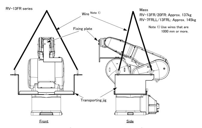
Fig.2-6: Transportation procedure (transporting with a crane: RV-13FR series)
