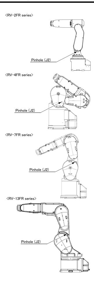
7) Move the J2 axis slowly with both hands to the following position and align the pinhole of the No.1 arm and the pinhole at the shoulder.
