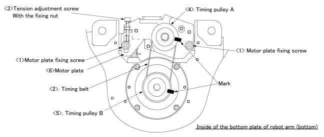
Fig.5-10: Replacing the J1 axis timing belt (RV-2FR series)
