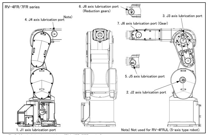
Fig.5-28: Lubrication positions (RV-4FR/7FR series)
