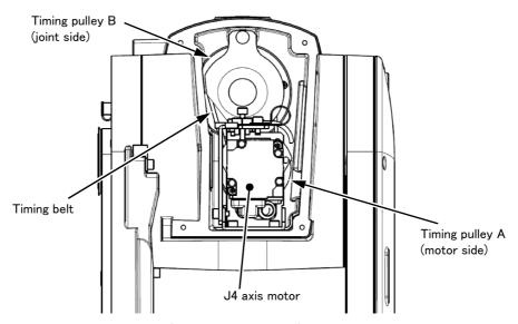
Fig.5-21: Inspection of J4 axis timing belt (RV-4FR/7FR series)
