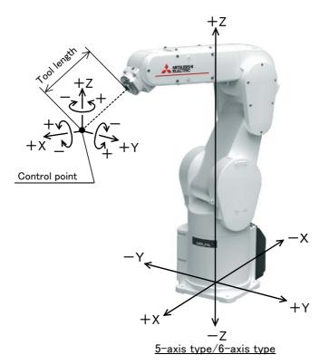
\* While maintaining the flange surface posture, the axis moves straight along the base coordinate system. The 6-axis type robot maintains the flange surface posture.
