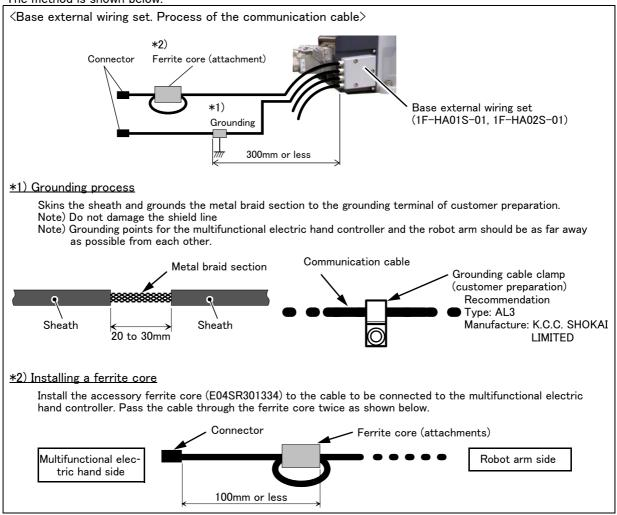
The installing of the base external wiring set is completed.
