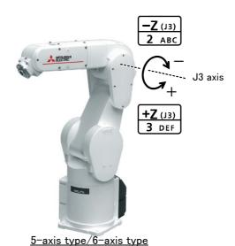
• When the [+Z (J3)] keys are pressed, the J3 axis will rotate in the plus direction. When the [-Z (J3)] keys are pressed, rotate in the minus direction.
