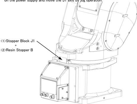
4) Install the <3> Mechanical Stopper screw. Install the <3> attached Mechanical Stopper screw to the needed point with referring to Table 3-11 and Fig. 3-4.
