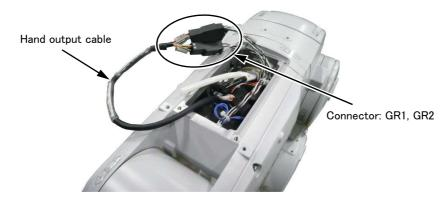
5) Feed the hand output cable through the cable clamp box. Loosens the threaded cap of the cable clamp and removes the plug of the cable clamp box. (Tip) Pass the cable with little by little, and pulls out the needed length, and fix the cable securely by tightening the threaded сар.
