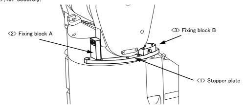
3) Install the Variable stopper block <5> by using two screws (RV-4FR: screw <8>, RV-7FR: screw <7>). There are two installation positions in the +/- side respectively. Install to the position of the angle which limits the operating range with referring to Table 3-8 and Table 3-9. Install the minus side in the same way. Move the J1 axis to the +70 degrees using jog operation previously, and install. (Turn on the power supply and move the J1 axis by jog operation) After installation, turn on the
