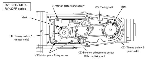
$Fig. 5-24: Inspection \ and \ replacement \ of \ J5 \ axis \ timing \ belt \ (RV-13FR/13FRL, \ RV-20FR \ series)$
