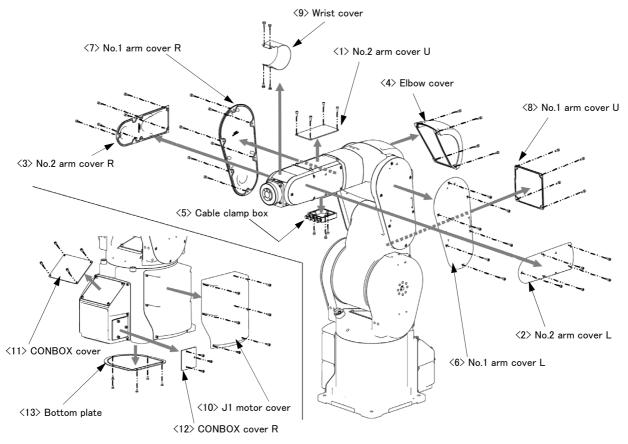
Fig.5-5 : Installing/removing the cover (RV-4FR/7FR series)
