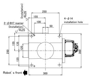
Fig.2-7: Installation dimensions
