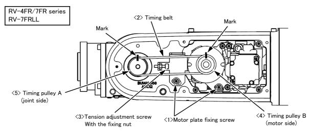
Fig.5-25: Inspection and replacement of J6 axis timing belt (RV-4FR/7FR series, RV-7FRLL)
