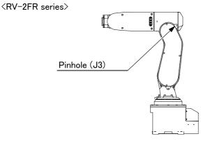
7) Move the J3 axis slowly with both hands to the following position and align the pinhole of the No.1 arm and the pinhole at the elbow.
