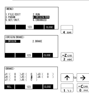
2) Press the [4] key on the menu screen, and display the Origin/BRK selection screen.
