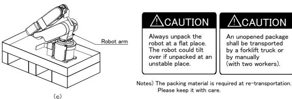
Fig.2-2: Unpacking the robot arm (RV-2FRL/2FRLB)
