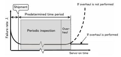
Fig.5-32: Periodic inspection/overhaul periods
