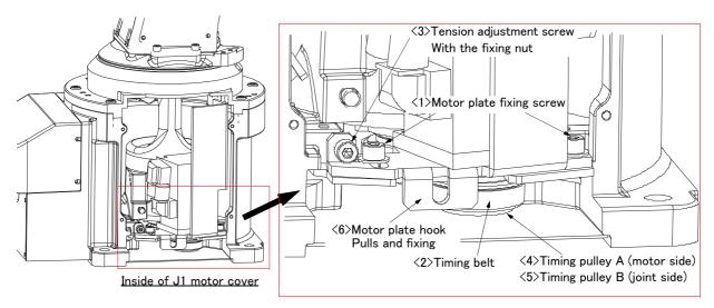
Fig.5-9: Inspection, maintenance and replacement of J1 axis timing belt (RV-2FR series)
