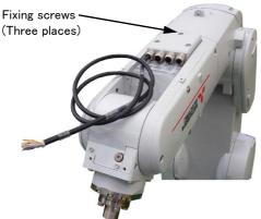
\* The figure is the example to which the J4 axis was moved to upside down position by jog operation. (For 6-axis type robot)
