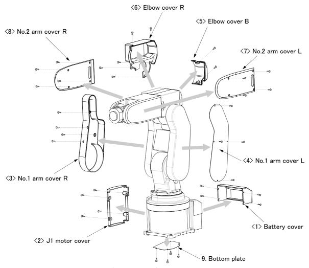
Fig.5-4: Installing/removing the cover (RV-2FR series)
