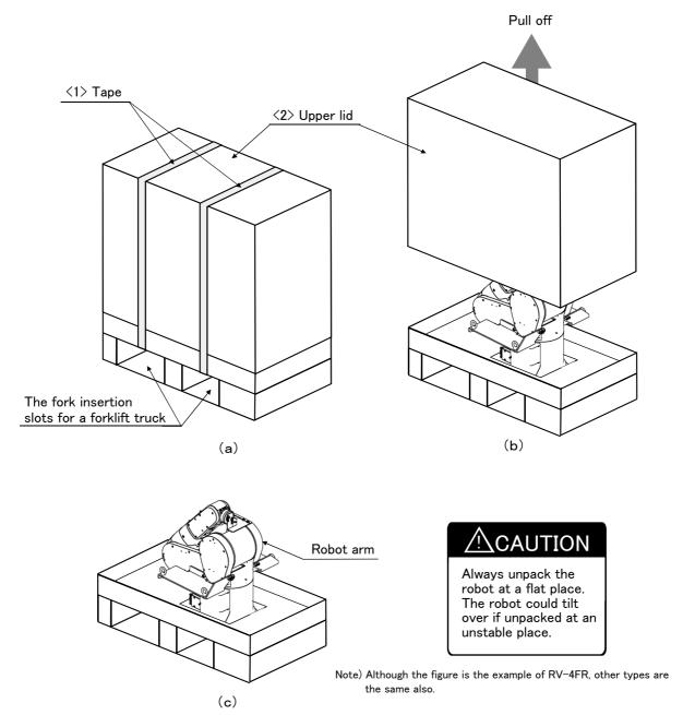
Fig.2-3: Unpacking the robot arm (RV-4FR/7FR/13FR series)
