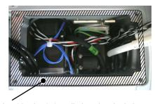
The solenoid valve is installed to the shaded area. To prevent cables from being pinched, push the cables into the forearm and avoid placing any cable on the shaded area.
