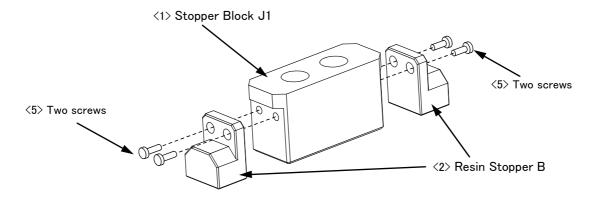
2) Install <1> Stopper Block J1 which combined with <2> Resin Stopper B to behind the J1 axis of robot arm by <4> two attached screws.
