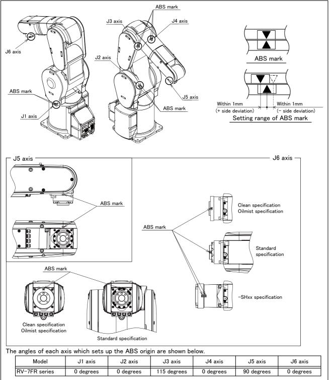
Fig.5-38 : ABS mark attachment positions (RV-7FR series)
