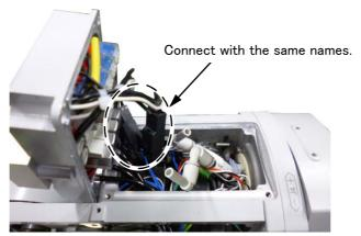
c) Store the connected connectors in the positions shown in the figure below.
