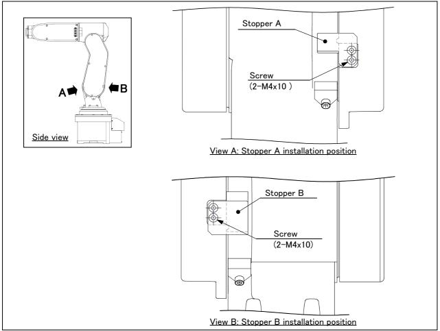
Fig.3-2: Installation procedure of optional stoppers
