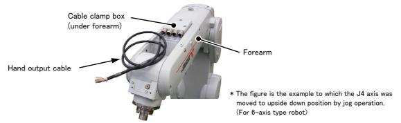
Fig.3-7: Image which pulled out hand output cable
