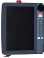
This is used to create, edit, and control the program, teach the operation position, and perform jog feed. This high-performance teaching pendant is equipped the graphical user interface with a touch panel, which makes it easy to perform each operation. Also, for safety purposes, a 3-position enable switch <sup>\*1)</sup> is mounted.
