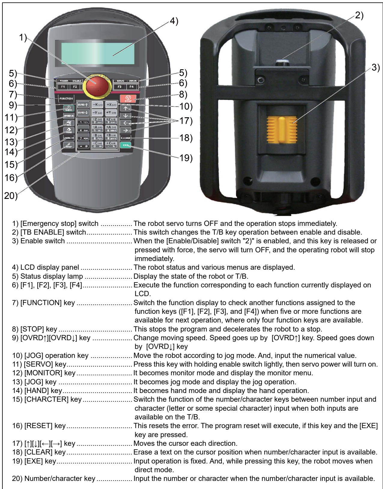
Fig.3-19: Teaching pendant key layout and main functions
