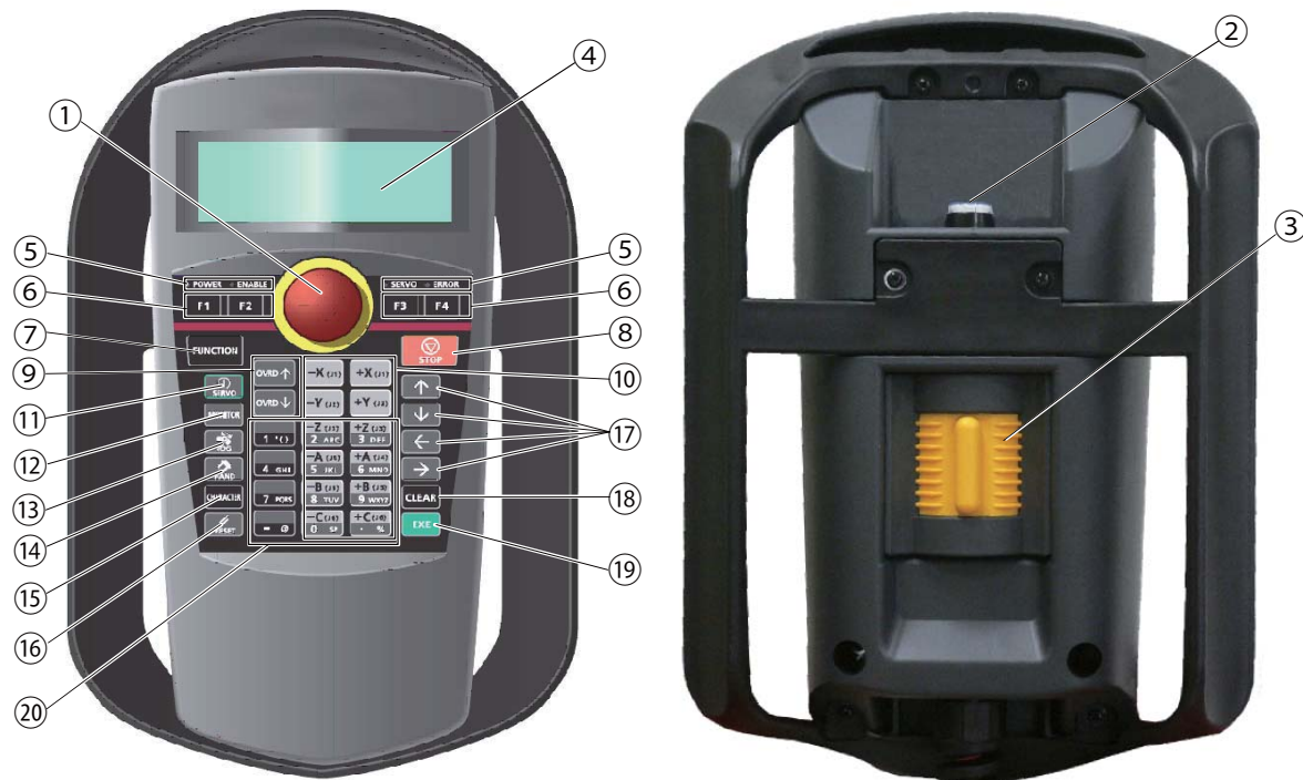
Fig.: Teaching pendant key layout and main functions
