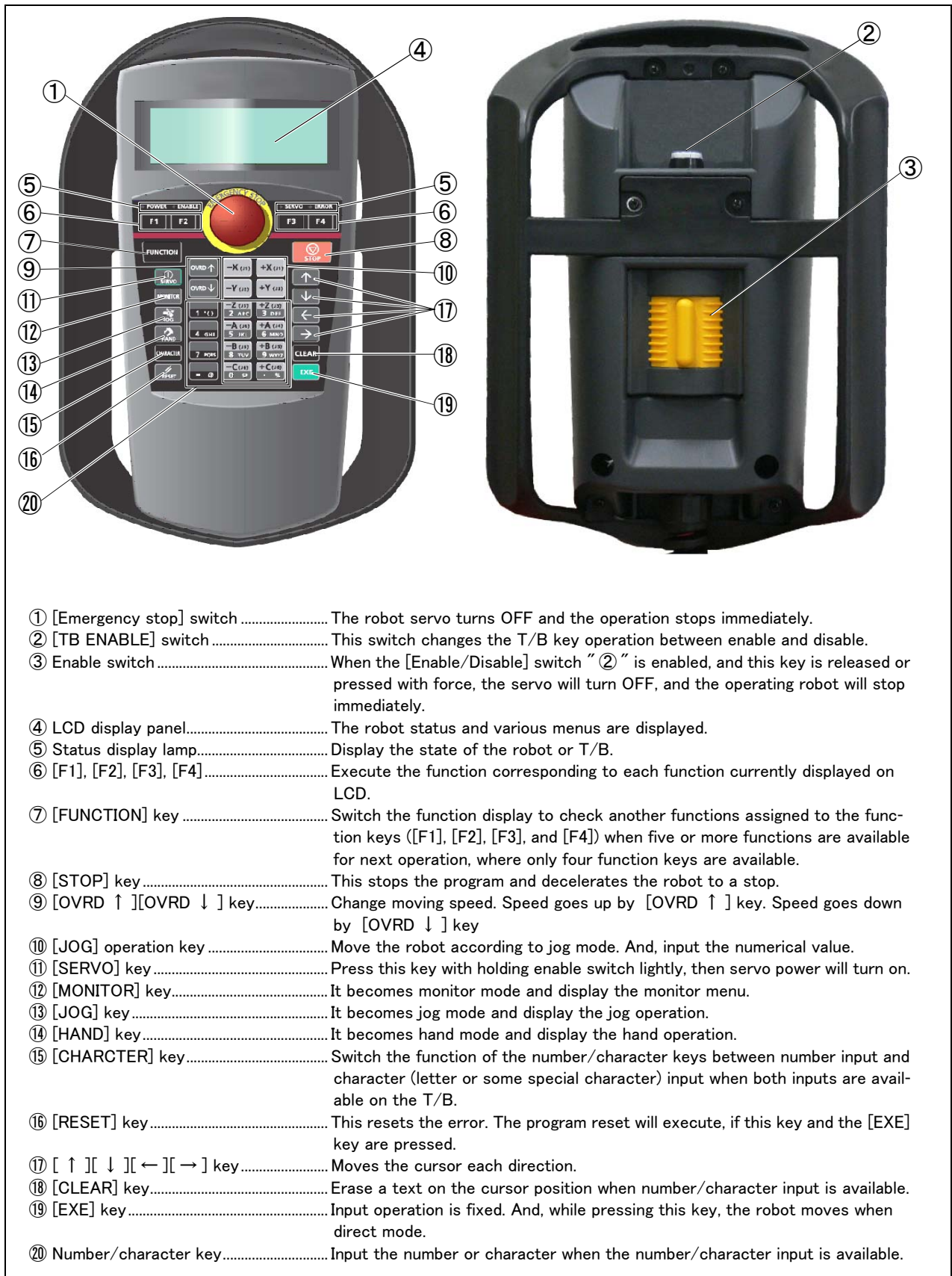
Fig.3-24 : Teaching pendant key layout and main functions
