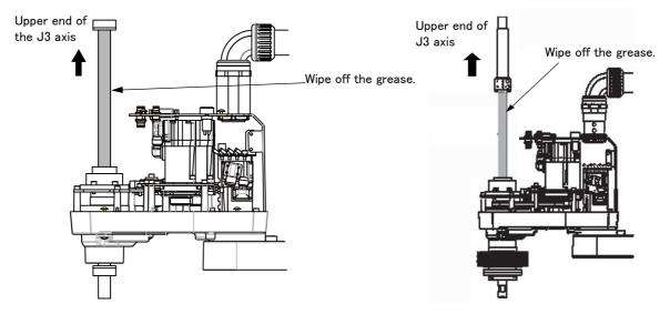
7) Apply the specified amount of grease to the shaft. Fill the shaft grooves with the grease. Also, apply the grease lightly to the areas other than the grooves on the shaft surface to prevent rusting.
