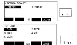
2) Press the [1] key on the ORIGIN/BRAKE screen, and display the origin setting method selection screen.
