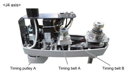
Fig.5-11: Inspecting the timing belt
