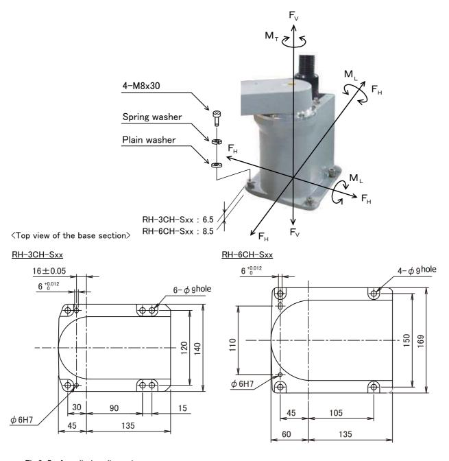
Fig.2-5: Installation dimensions
