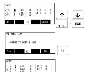
4) Input "1" into the axis to origin setting. Press the [EXE] key, and display Confirmation screen.
