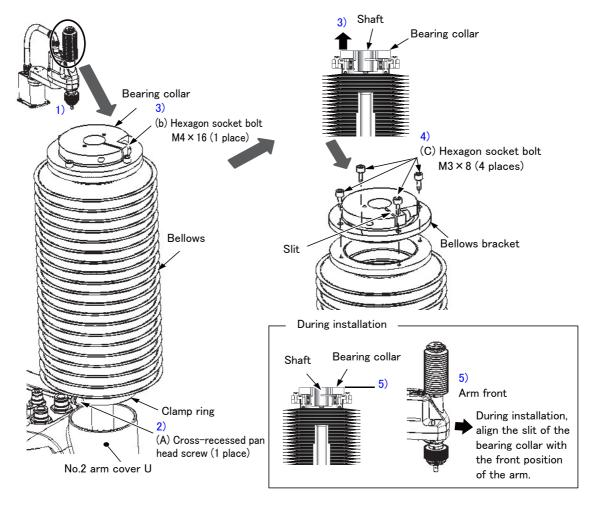
Fig.5-6: Installation/removal of bellows U
