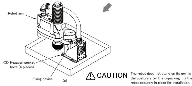
the posture after the unpacking. Fix the robot securely in place for installation.
