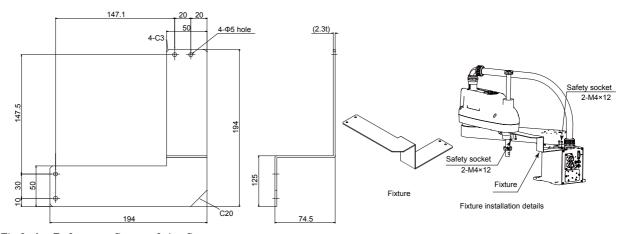
Fig.2-4: Reference figure of the fixture
