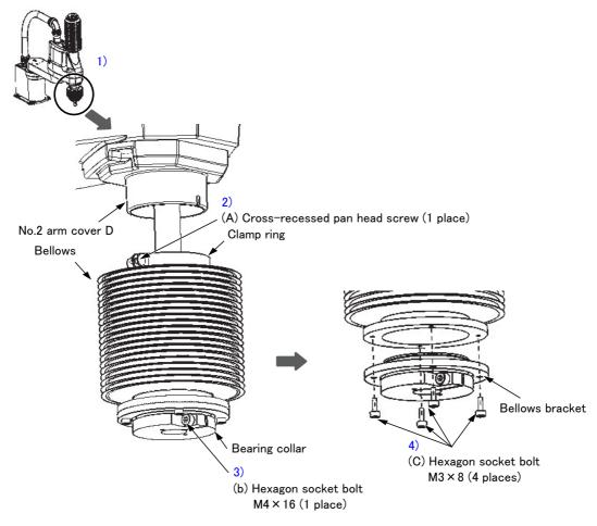
Fig.5-7: Removing bellows L
