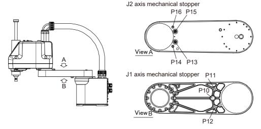
Fig.3-1: Mechanical stopper position
