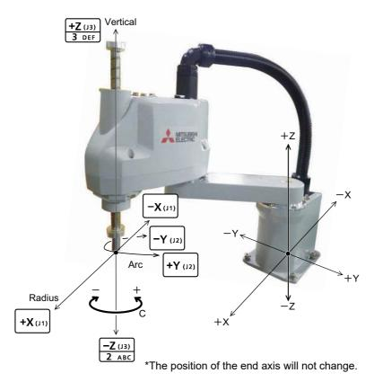
• When the [+C (J6)] keys are pressed, the Z axis will rotate in the plus direction. When the [-C (J6)] keys are pressed, rotates in the minus direction.
