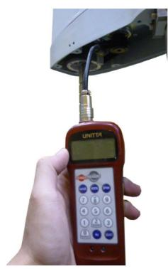
Fig.5-9: Tension adjustment method of timing belt
