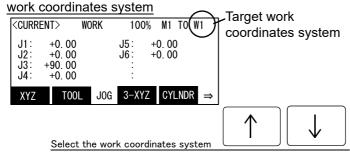
Confirm the target work coordinates system. The current target number is displayed on the screen upper right. (W1 - W8)
