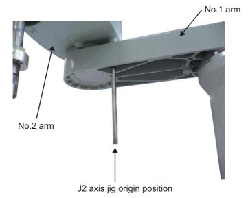
2) Move the J2 axis slowly using both hands. Align the pinholes of the No. 1 and No. 2 arms, feed through the origin jig into the pinholes and
