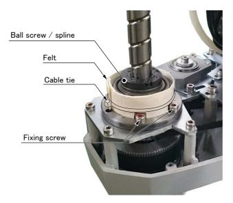
Fig.5-14: Replacing the felt
