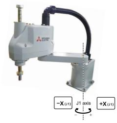
When the [+X (J1)] keys are pressed, the J1 axis will rotate in the plus direction.
