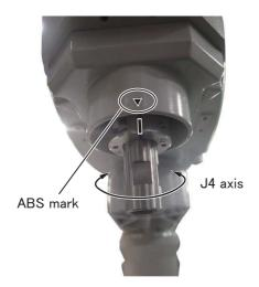
7) Hold the J4 axis with your hand and rotate it slowly to align the slit with the ABS mark. \*Move the J4 axis with maintaining the condition that the releasing brake of the J3 axis and the J3 axis contact to the mechanical stopper.
