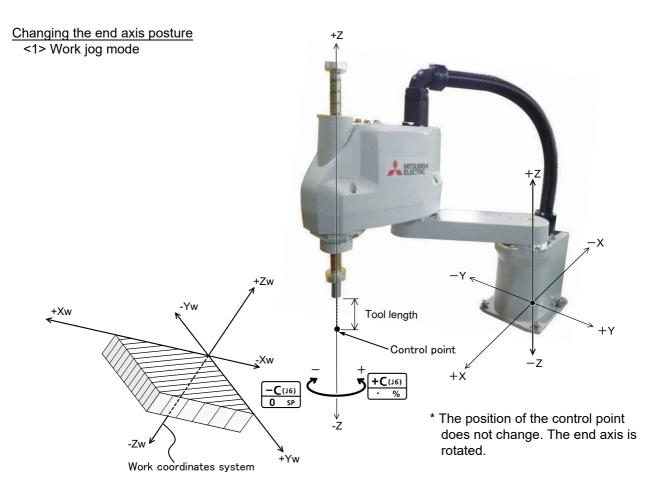
• When the [+C (J6)] keys are pressed, the Z axis will rotate in the plus direction of the XYZ coordinate system. When the [-C (J6)] keys are pressed, rotate in the minus direction.
