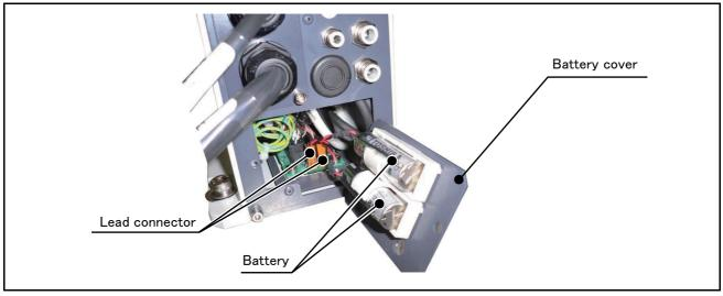
Fig.5-13: Replacing the battery
