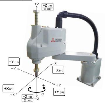
•When the [+X (J1)] keys are pressed, the robot will move along the X axis plus direction of the tool coordinate system.
