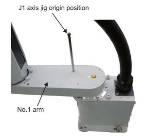
2) Move the J1 axis slowly toward the front using both hands. Align the pinhole of the No.1 arm and the pinhole at the base section, feed through the origin jig into the pinholes and fas-
