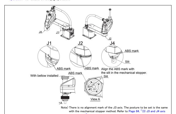
The angles of each axis which sets up the ABS origin are shown below.
