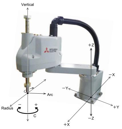
\* The current position is set as the arc centering on the Z axis, and the axis moves along that arc, expands and contracts in the radius direction, and moves vertically. At this time, the end axis posture is maintained. Also, while maintaining the axis posture position, the end axis posture changes.
