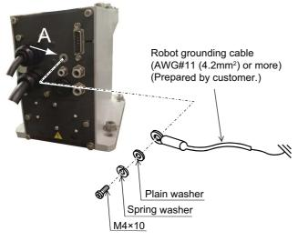
Fig.2-7: Connecting the grounding cable
