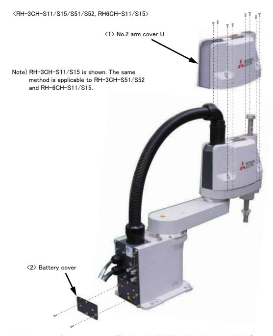
$Fig. 5-4: Installing/removing \ the \ cover \ (RH-3CH-S11/S15/S51/S52, \ RH-6CH-S11/S15)$
