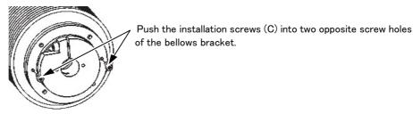
For the bolting torque of each screw, refer to Table 5-4.
