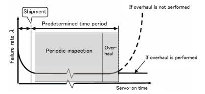
Fig.5-15: Periodic inspection/overhaul periods
