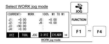
[JOG] Press the key and display the jog screen. ("JOG" is displayed on the screen bottom)
