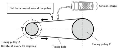
Fig.5-10: Timing belt tension measurement
