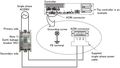
Note 1) The earth leakage breaker is the customer preparation. Always use the cover below. Recommendation: NV30FAU-2P-10 A-AC100-240 V-30 mA, (Cover: TCS-05FA2)
