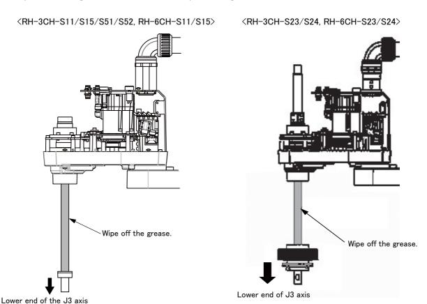
5) Turn on the controller's power supply, and move the J3 axis to the upper end limit by jog operation. Then, turn off the controller's power supply again.
