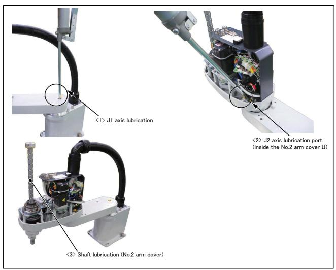
Fig.5-12: Lubrication positions
