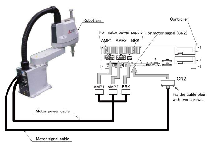
Fig.2-8: Connecting the machine cables
