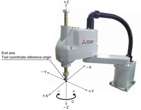
\* While maintaining the end axis posture, the axis moves straight along the tool coordinate system.
