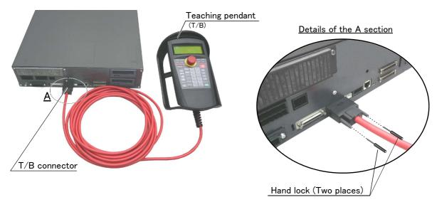
Fig. 2-9: Installing and removing the T/B (CR751controller)
