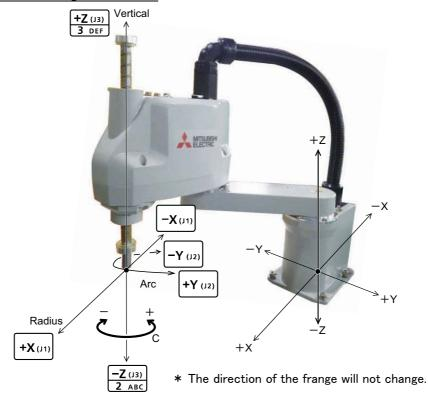
Assuming that the current position is on an arc centering on the Z axis, the robot moves along that arc.
