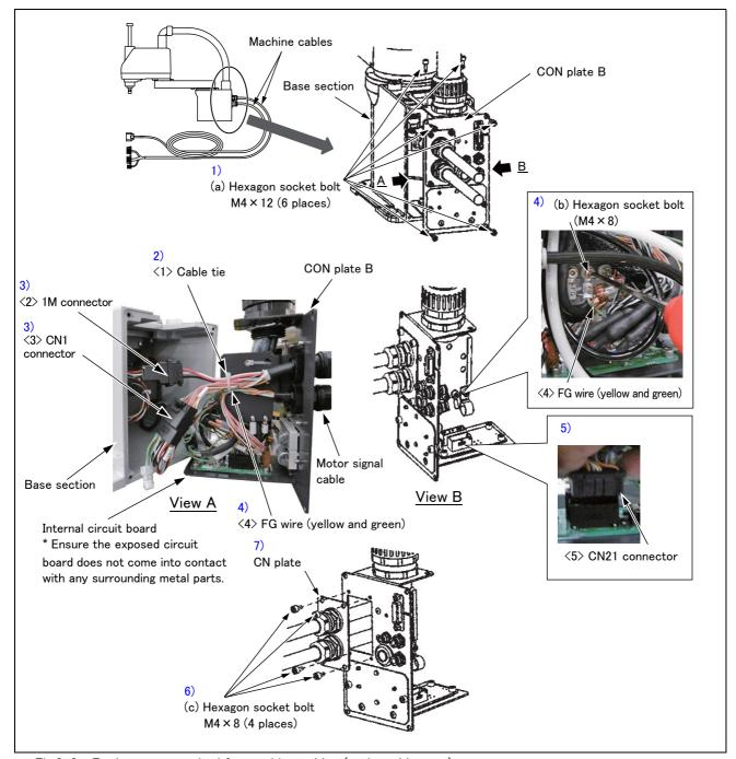
Fig.3-2: Replacement method for machine cables (replaceable type)
