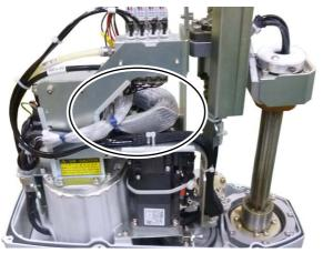
5) Fix the expanding sleeve with a cable tie using a hole on the metal plate.
