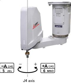
• When the [+A (J4)] keys are pressed, the J4 axis will rotate in the plus direction. When the [-A (J4)] keys are pressed, rotate in the minus direction.
