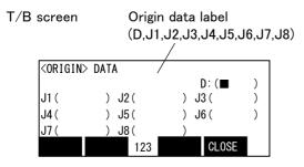
Input the value confirmed in section Page 90, "(1) Confirming the origin data". The correspondence of the origin data label value and axis to be input is shown in Fig. 5-17.
