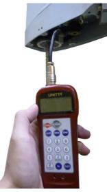
Fig.5-8 : Tension adjustment method of timing belt
