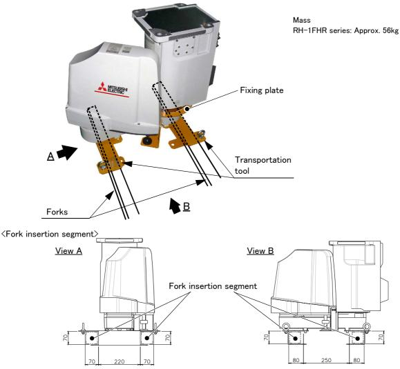
Fig.2-3 : Transportation of robot arm
