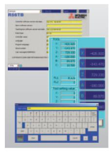
The R56TB is a powerful operating panel for carrying out all tasks directly at the robot, from controlling the robot and displaying the loads by means of the input/output display to complete program creation and parameterisation.
