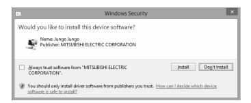
• If the driver is not installed, communication may be partly interrupted. In this case, reinstall MR Configurator2.
