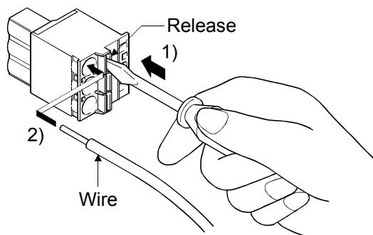
**(Note):** When using a ferrule, make sure the bumpy side is facing towards the release.
