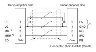
\*1 Encoder cables that meet the following specifications are recommended.
