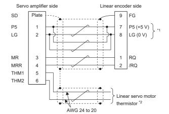
Housing: 1-172161-9 Connector pin: 170359-1 (TE Connectivity or equivalent) Cable clamp: MTI-0002 (Toa Electric Industrial)
