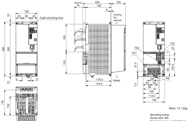
Tightening torque: 3.24 [N•m]
