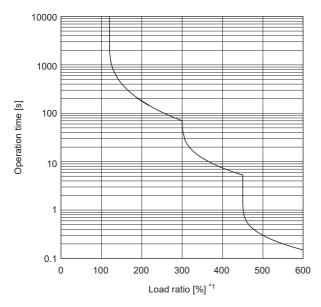
\*1 A resistive force of 100 % indicates the continuous rating of the converter unit.
