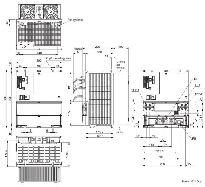
Terminal TE2-2 Screw size: M10 TE2-1 TE1 Tightening torque: 12.0 [N•m]
