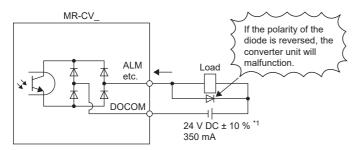
\*1 If the voltage drop (a maximum of 2.6 V) interferes with the relay operation, apply high voltage (a maximum of 26.4 V) from an external source
