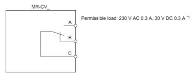
\*1 For compliance with the IEC/EN/UL/CSA standards, operate at 30 V DC or less.
