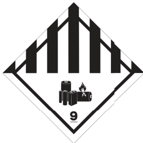
Figure 2: Lithium battery hazard label example
