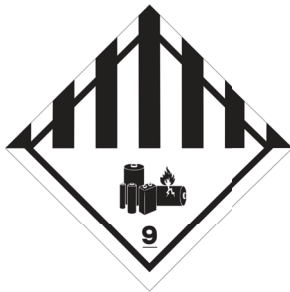
Figure 2: Lithium battery hazard label example
