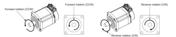
The positive and negative directions of the linear servo motor are as follows.
