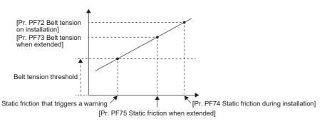
Belt tension threshold = [Pr. PF76 Belt tension irregular threshold]/100 × [Pr. PF72 Belt tension on installation]
